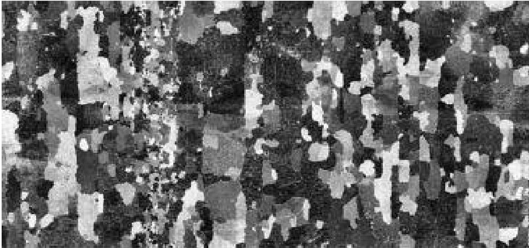
Figure 24 The example of grain structure of GO steel: in the left part an incompletely recrystallized line is visible [30]
