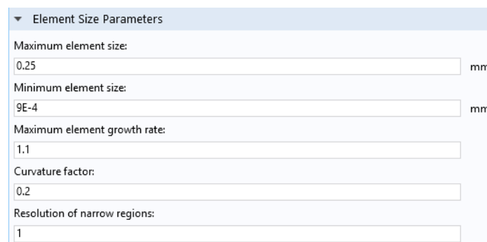
Figure 2.23: Finite element size parameters.
