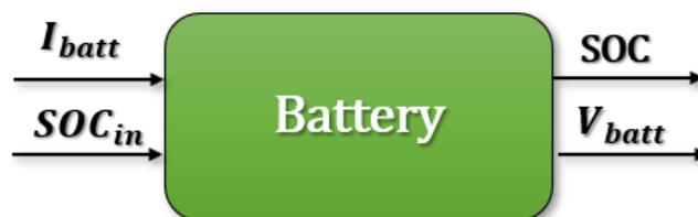
Figure 3.39: **Battery** subsystem.
