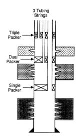
Figure 5.5: Wellbore diagram of a conventional triple completion, [29].
