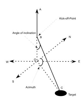
Figure 2.1: Measurement Parameters of a directional well, [5].
