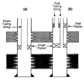
**Figure 5.4:** (a) casing-tubing dual completion. (b) completion with dual packers and dual tubing strings, [29].
