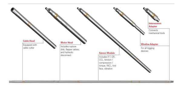
Figure 5.12: The industry's shortest real-time coiled tubing solution with full intervention and diagnostic capabilities, [36].
