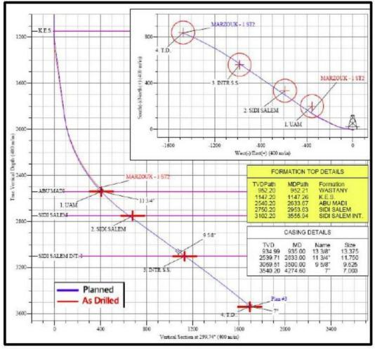
Figure 2.5: J Profile Directional well plan (Jones et al., 2008), [7].
