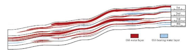
Figure 4.2: The quasi-continuous oil tight sandstone reservoirs, [15].
