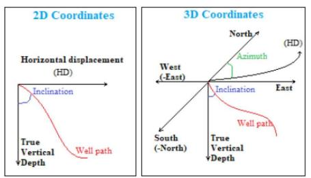
Figure 3.9: 2D and 3D cases for well path visualization, [11].
