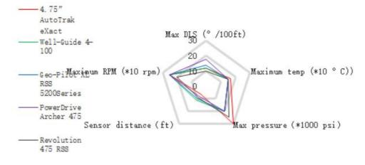
Figure 3.5: Comparison of performance indicators of 4.75-inch RSS Tools, [13].
