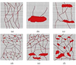
**Figure 4.1:** Different patterns of fractured-vuggy medium. (a) fracture network; (b) isolated cave; (c) cave-fracture-cave; (d) pore-fracture-pore; (e) pore-fracture-cave; (f) Cave network [24].
