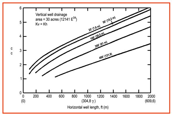
Figure 4.4: Horizontal/Vertical Well Productivity Index Ratio as a Function of the Reservoir Thickness, [15]
