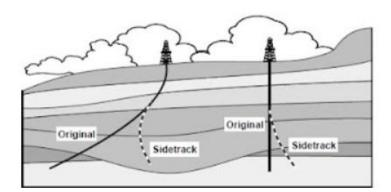
Figure 2.6: Sidetracking
