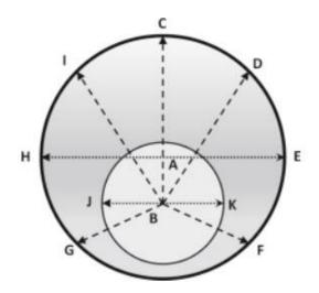
Figure 2.12: Tool centering in the wellbore, [6].
