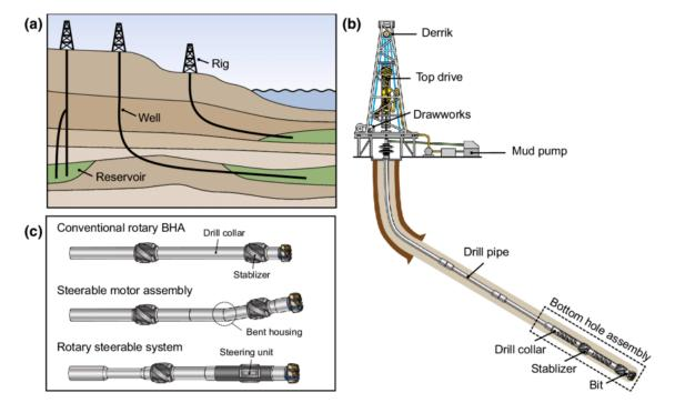
**Figure 3.1: A)** Applications of directional wells: single surface location for multiple wells, onshore drilling to an offshore reservoir, B) schematic representation of a typical drilling system, C) three typical kinds of BHAs widely used in the oil field, including the conventional rotary BHA, the steerable motor assembly, and the RSS, [10].
