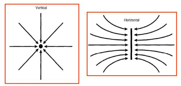
Figure 4.3: Comparison of flow geometries of vertical and horizontal wells, [15].
