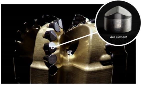
Figure 4.17: Axe blade element fitted in Drilling Bit, [26].
