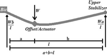
Figure 3.8: Beam bending analysis, [11].
