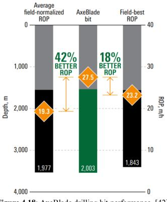
Figure 4.18: AxeBlade drilling bit performance, [42].
