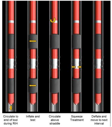
Figure 5.14: Electric inflatable packer SPECTRUM e-IP, [38].
