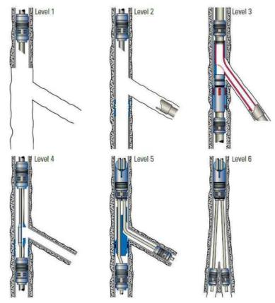
**Figure 5.8:** Multilateral standards classify junctions as TAML Level 1, 2, 3, 4, 5, or 6 based on mechanical complexity, connectivity, and hydraulic isolation, [32].
