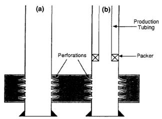
Figure 5.3: (a) perforated completion. (b) completion string inside perforated casing, [29].
