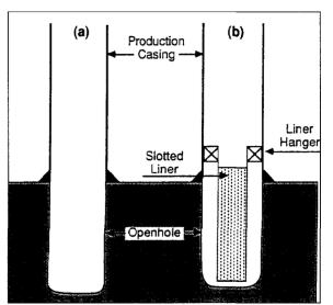
Figure 5.1: The diagram of a wellbore (a) open hole completion. (b) a slotted liner completion, [29].
