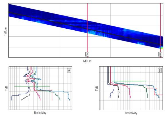
Figure 4.15: IriSphere service differentiated between stringers and the expected target carbonate in real time, [41].
