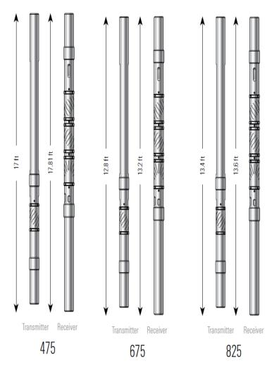
Figure 4.14: IriSphere tool size, [24].
