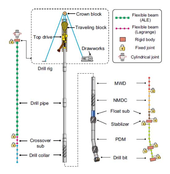
**Figure 3.2**: Schematic of the whole drilling system and its multibody dynamic model. The length of the drill pipes is greatly reduced to clearly illustrate such a slender system, [10].
