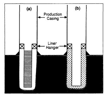
Figure 5.2: A. screen and liner completions. B. cement liner completion, [29].
