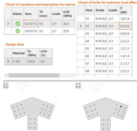
Figure 62: Type of plates and bolts type 3 connection
