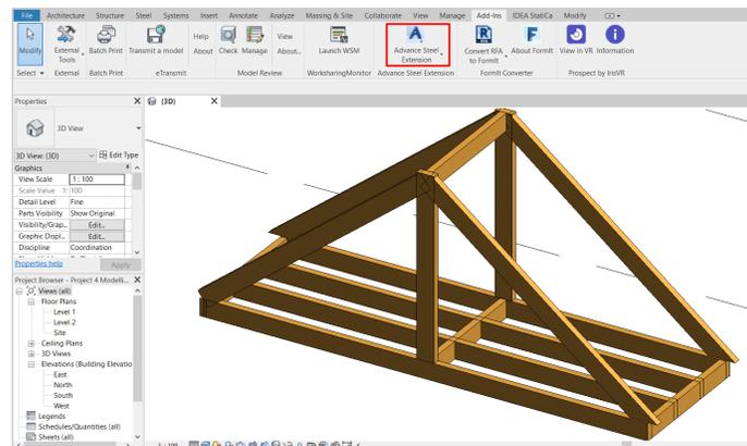
Figure 48: Interoperability - Add in to pass from Revit to Advance steel
