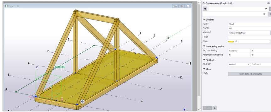
Figure 73: Superstructure (Piedicavallo bridge) using Tekla
