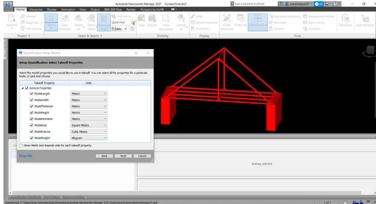
Figure 76: Project quantification - Using Navisworks
