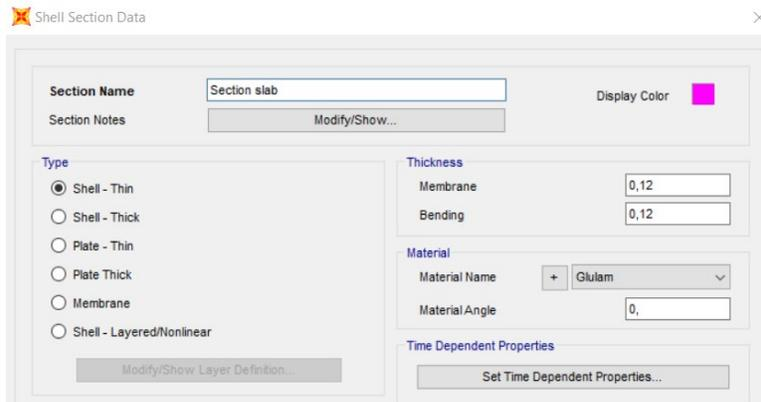
Figure 26: Section dimension of the floor (Glulam Slab)
