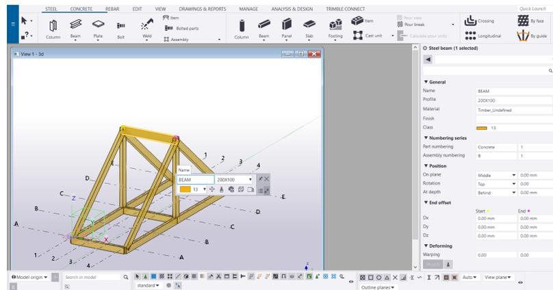
Figure 72: Construction of the architectural design, Tekla view.
