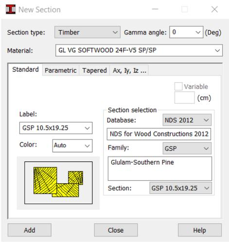
Figure 40: Section and material used for Piedicavallo bridge.
