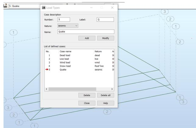
Figure 42: Types of loads – Robot
