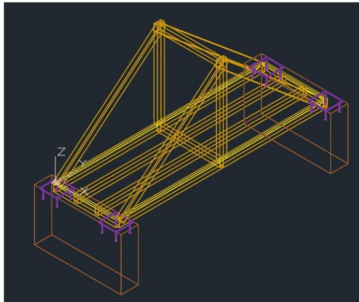
Figure 110: Bridge design – AutoCAD 3D
