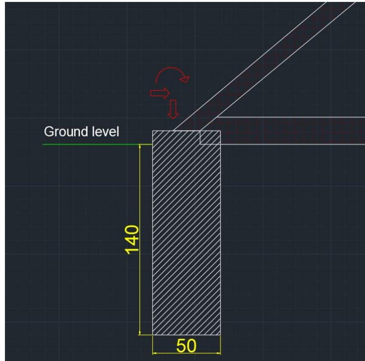
Figure 63: Dimensions of foundation using Autocad
