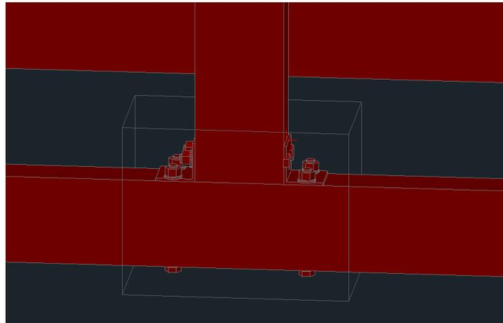
Figure 54: Connection beam perpendicular to column - Type 2
