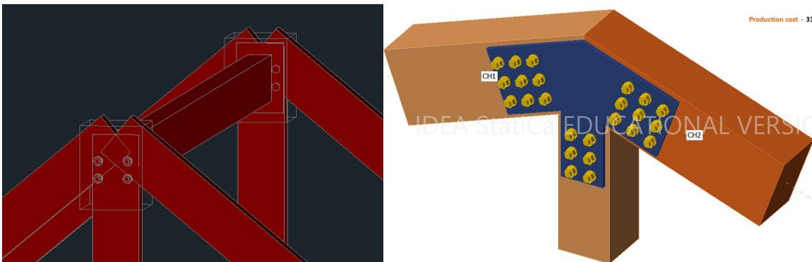
Figure 55: Top connection bridge - Type 3
