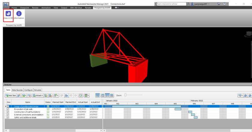
Figure 109: Export Detailed Piedicavallo bridge into a VR view - Using Navisworks Manage
