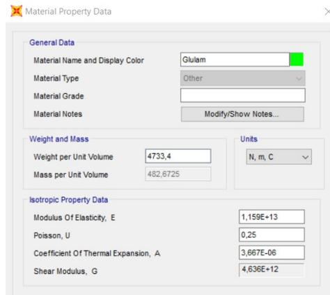
Figure 24: Structural data of GL24c
