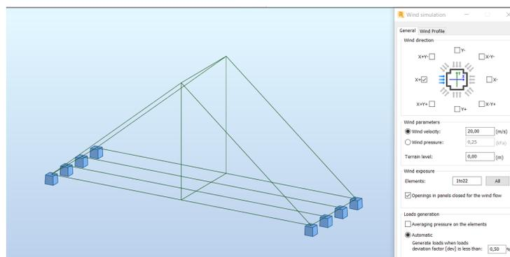
Figure 43: Wind load cases – Robot
