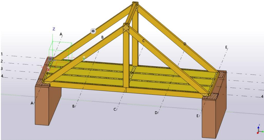
Figure 75: Final Executive architectural design, including joint assembly with foundation
