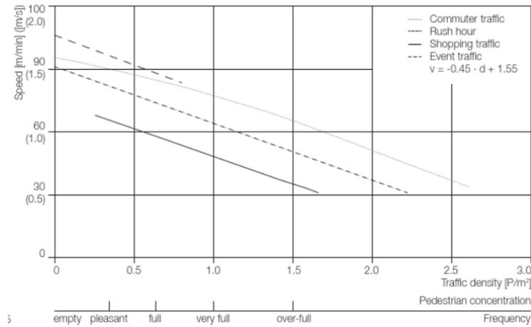
Figure 5: Graph - Linear relationship between traffic density and speed taken from (Keil, 2013)
