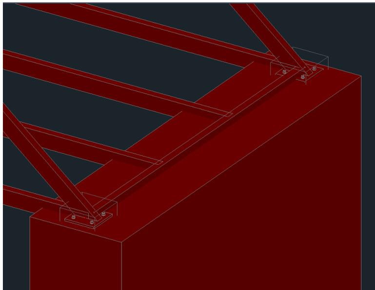
Figure 53: Border Base plate connection - Type 1
