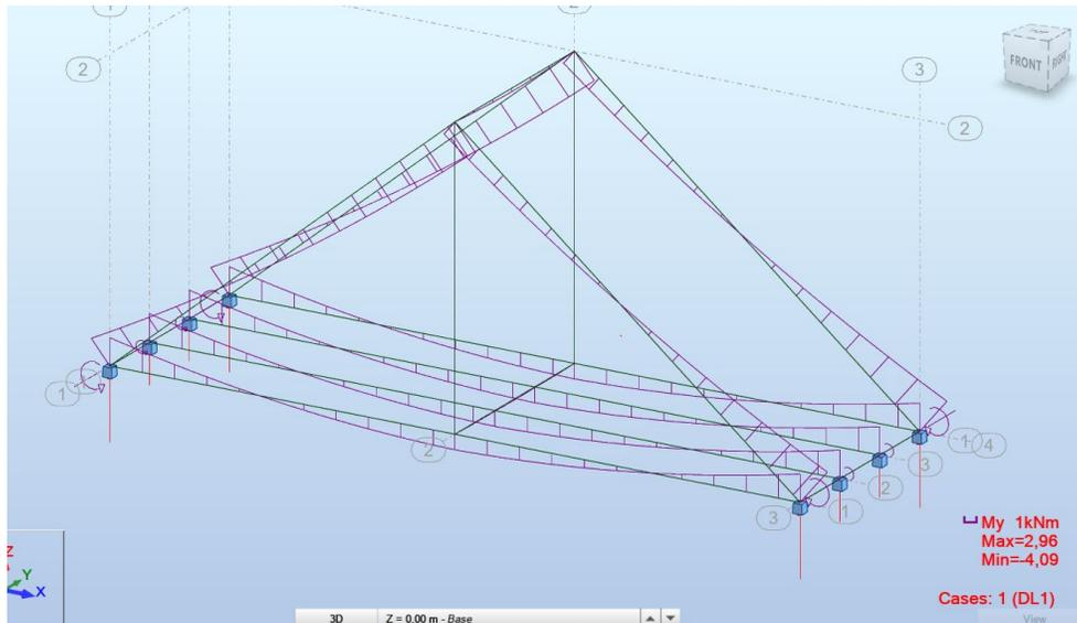
Figure 47: Final structure (Loads and reactions) – Robot
