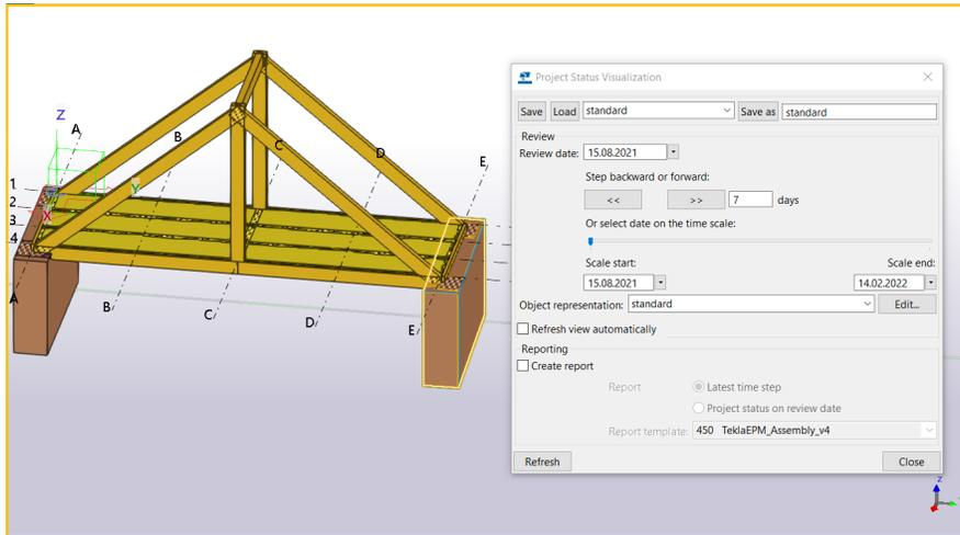
Figure 101: Project Status - Using Tekla Structures
