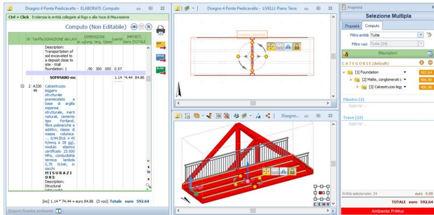
Figure 68: Edificius connection with Primus screen - Selection of components for assigning the corresponding activities
