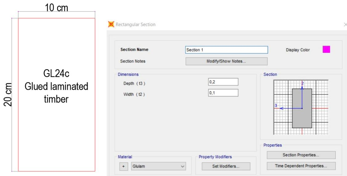
Figure 25: Section dimension of all elements (Columns and beams)
