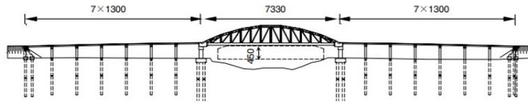
**Fig. 1.** Elevation view of Qifeng Bridge (unit: cm)
