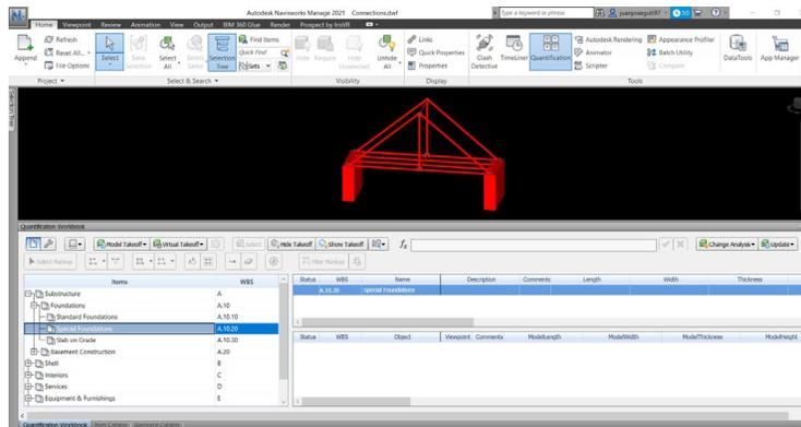
Figure 77: Model takeoff - Using Navisworks
