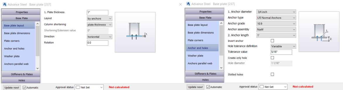
Figure 52: Dimension of plates and bolts
