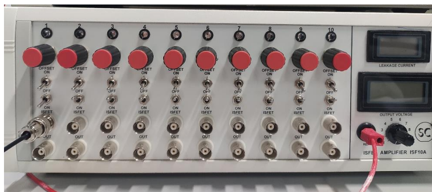
Figure 12 : ISFET amplifier. On the top right screen, the amount of leakage current detected from all the active ISFETs. On the display below, the output voltage is displayed depending on which channel is selected.
