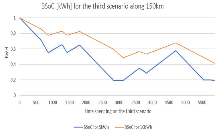
Figure 53 - Battery State of Charge for different constant velocities on third scenario with a capacity of 10KWh and 5Kwh
