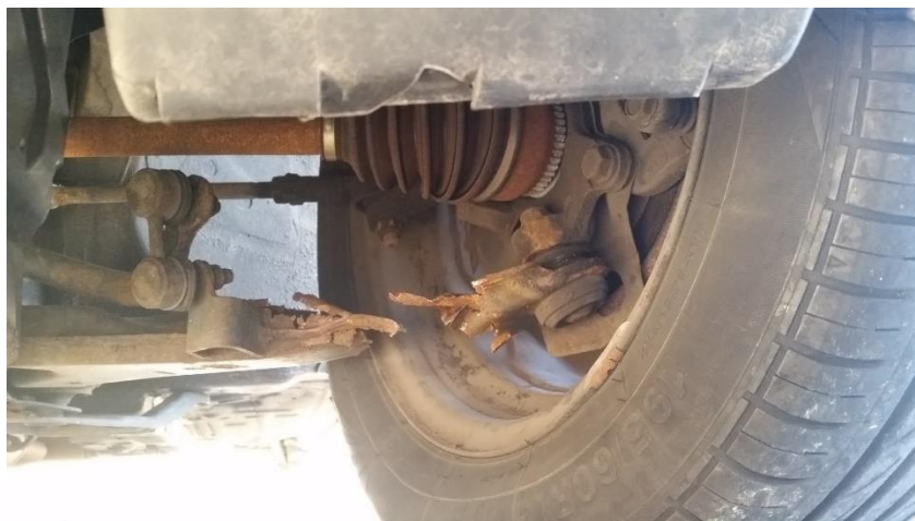
Figure 6 - A steering arms broken probably by a too huge vertical impact
