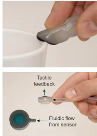
Figure 3.5: Hydraulic haptic feedback [33].
