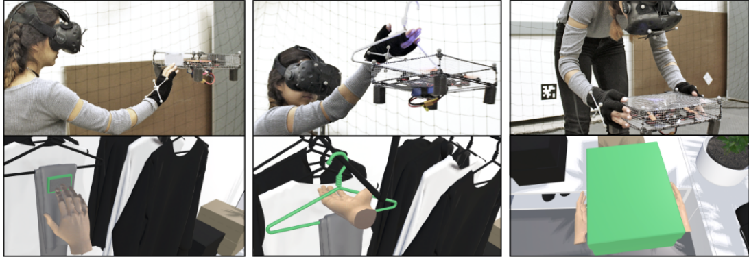
Figure 3.23: On the left the drone is used for texture rendering, in the center the drone is user for animation props and on the right the drone is used for passive haptic purpose [55].
