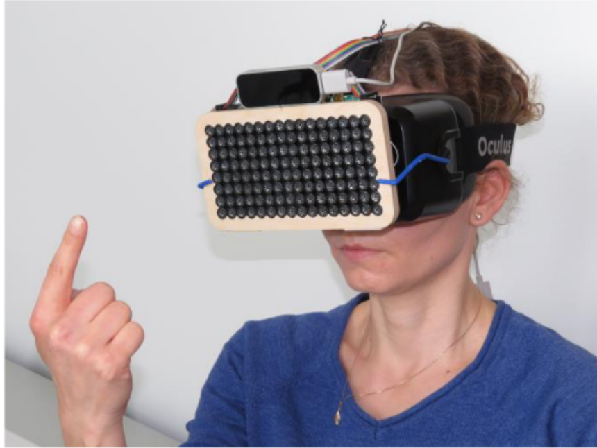
Figure 3.31: Array of transducers on HMD [63].
