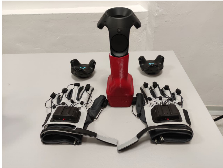
Figure 4.20: Configuration composed by ManusVR gloves and mockup.
