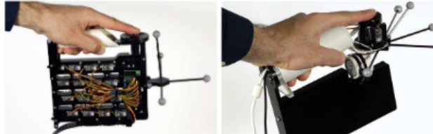
Figure 3.8: On the left the SenseTouch controller, on the right NormalTouch controller [39].
