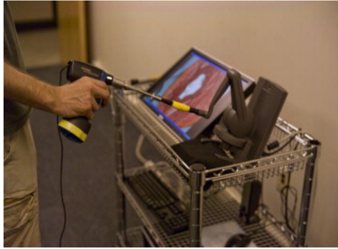
Figure 3.32: Drilling operation in orthopedic simulation.
