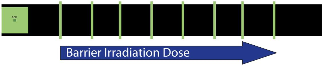
**Figure 2.28:** Irradiation scheme in scale of a long stripe to tune the barrier strength. The nucleation of the domain wall occurs on the left-hand side of the stripe due to background and ANC irradiation. The ion dose, as well as the barrier strength, increases from left to right over the different barriers.
