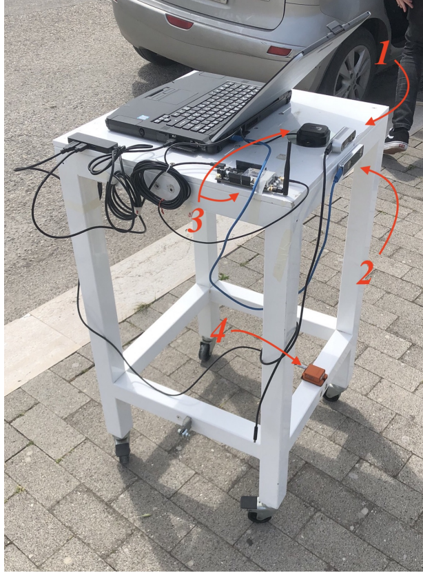
Figure 3.4: The figure shows the initial setup consisting of a mobile cart with sensors: 1) Intel® RealSense™ D435 depth camera, 2) Intel® RealSense™ T265 tracking camera, 3) GPS, 4) IMU.
