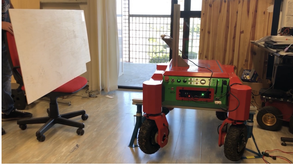
Figure 4.2: The picture depicts the robot, raised, with the Intel® RealSense™ D435 camera mounted on top to identify the orientation of the moving panel.
