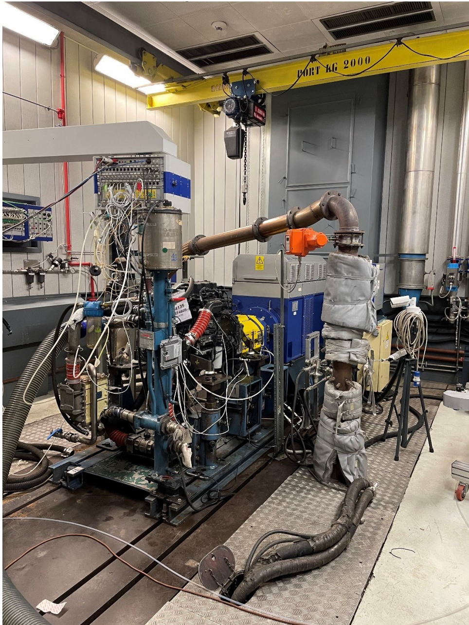
Figure 1.2: Engine and dynamo system.
