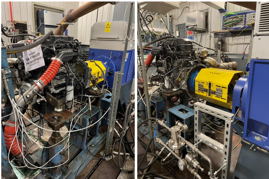
Figure 1.1: On the left, the test bench. On the right, a detail of the connection between engine and dynamo.
