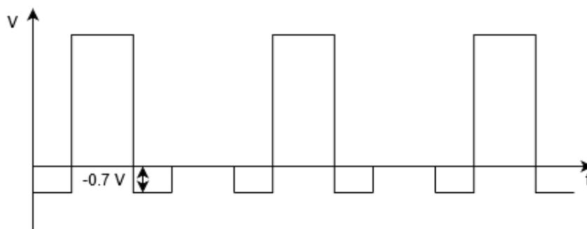
FIGURE 2.6: Voltage waveform of the switching node in a Buck converter that employs Silicon Mosfets as switches.
