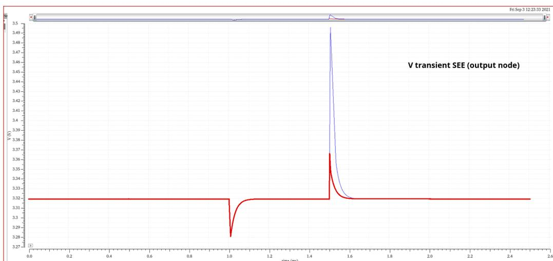
FIGURE 3.36: Comparison of SEE affecting the output voltage value with and without the sink NMOS transistors.
