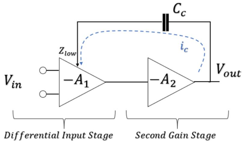
FIGURE 3.4: Diagram that shows an example of Indirect Feedback compensation [6].
