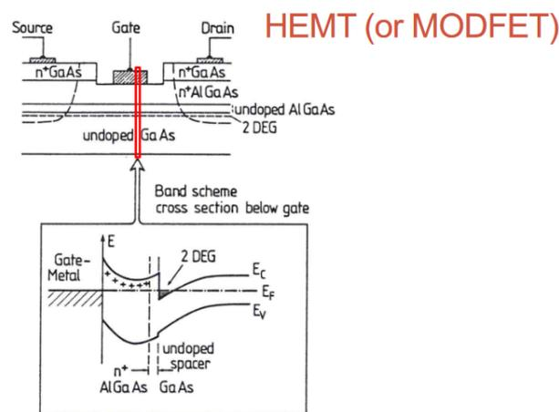
FIGURE 2.4: Example of band diagram of a HEMT [4].
