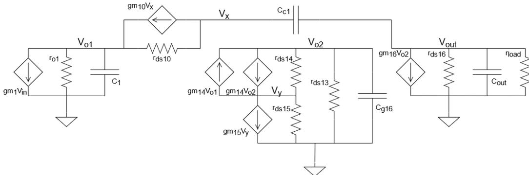
FIGURE 3.7: Small signal representation of the indirect feed-back compensated circuit (implemented topology).
