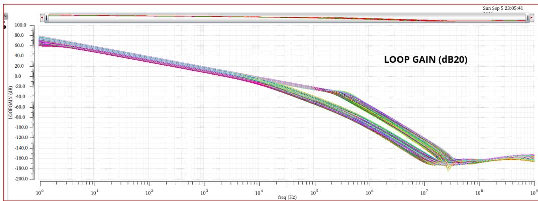
FIGURE 3.16: Loop Gain (dB20) of the circuit with the real bandgap across all design points.
