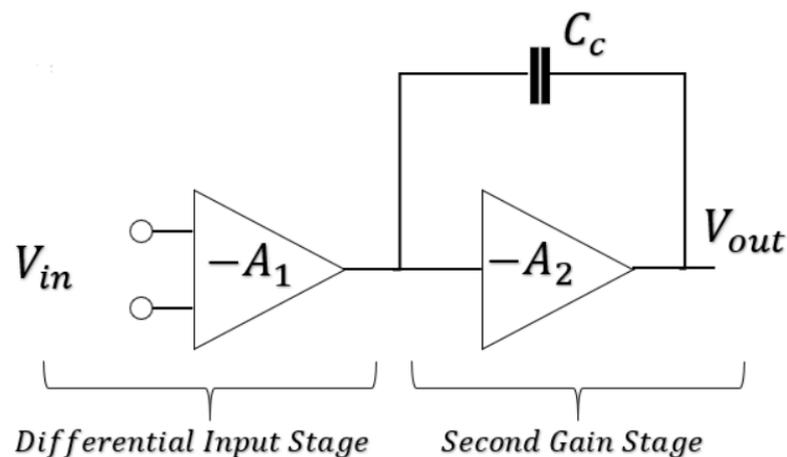
FIGURE 3.3: Diagram that shows an example of Miller compensation [6].
