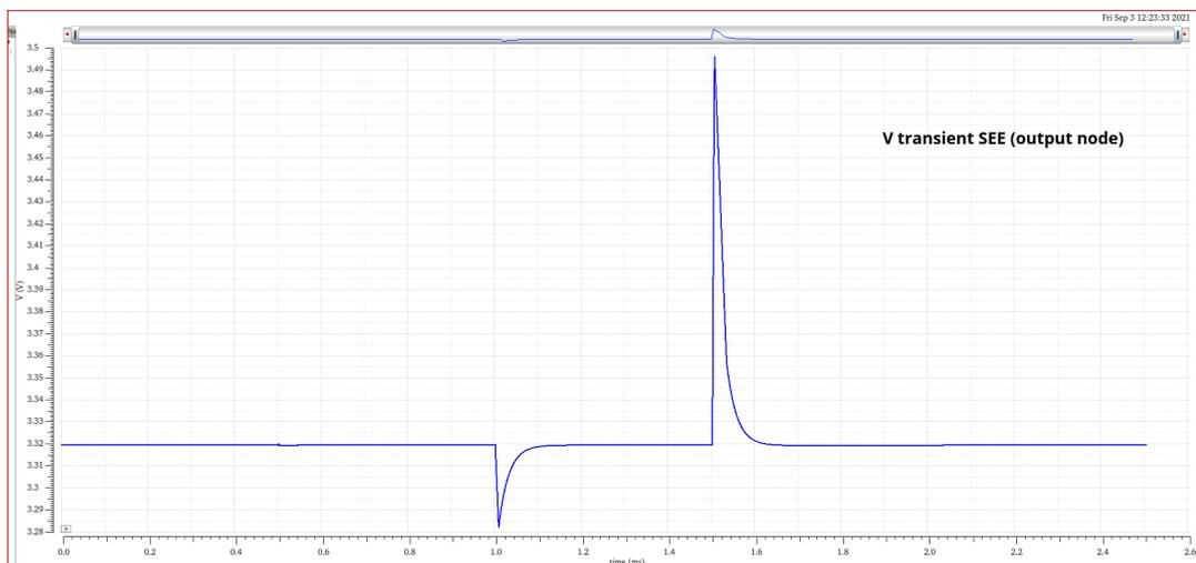
FIGURE 3.32: SEE affecting the output voltage value.
