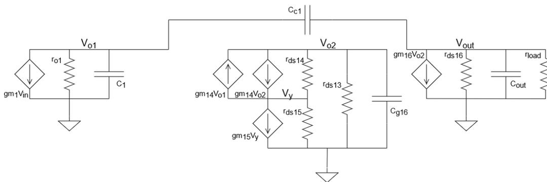
FIGURE 3.9: Small signal representation of the Miller compensated circuit (not implemented).
