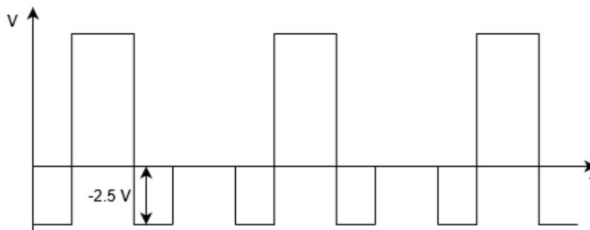
FIGURE 2.7: Voltage waveform of the switching node in a Buck converter that employs GaN FETs as switches.
