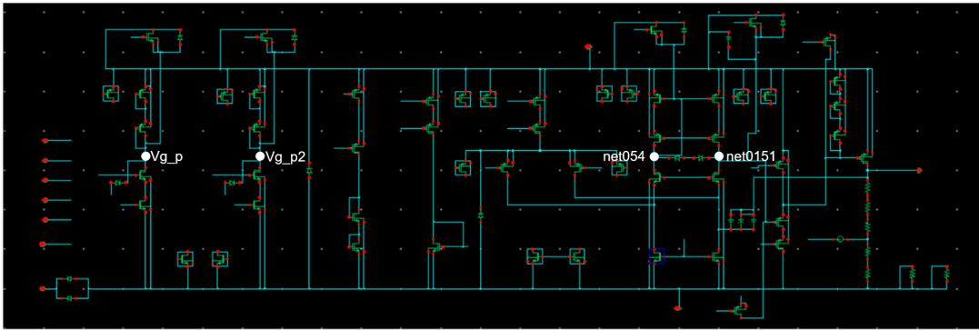
FIGURE 3.31: Critical nodes for SEE highlighted in the schematic.
