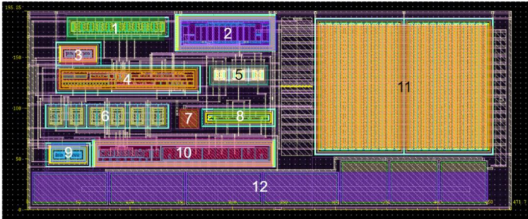
FIGURE 3.38: Screenshot of the final layout of the circuit with its components highlighted.
