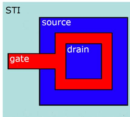
FIGURE 1.3: Representation of an Enclosed Layout Transistor.
