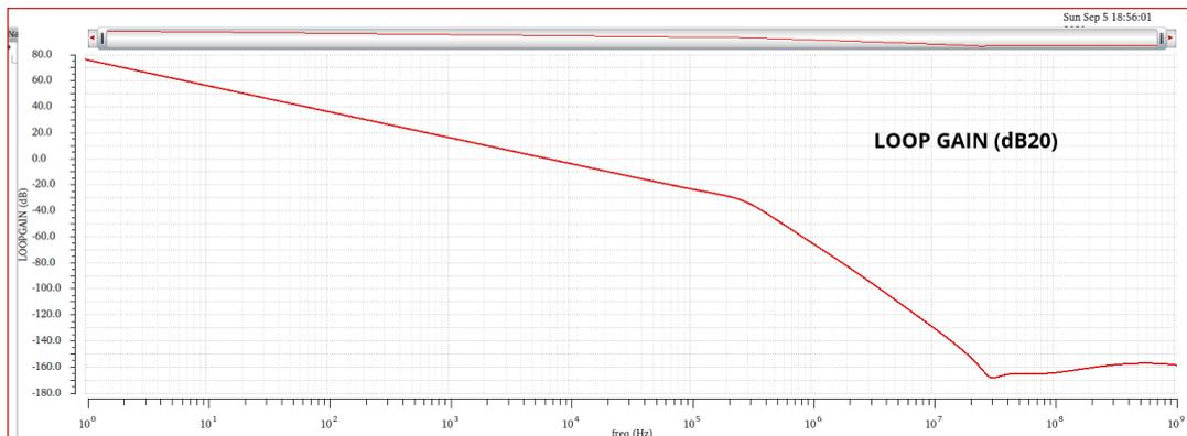
FIGURE 3.11: Loop Gain (dB20) of the circuit with the real bandgap in the nominal case.
