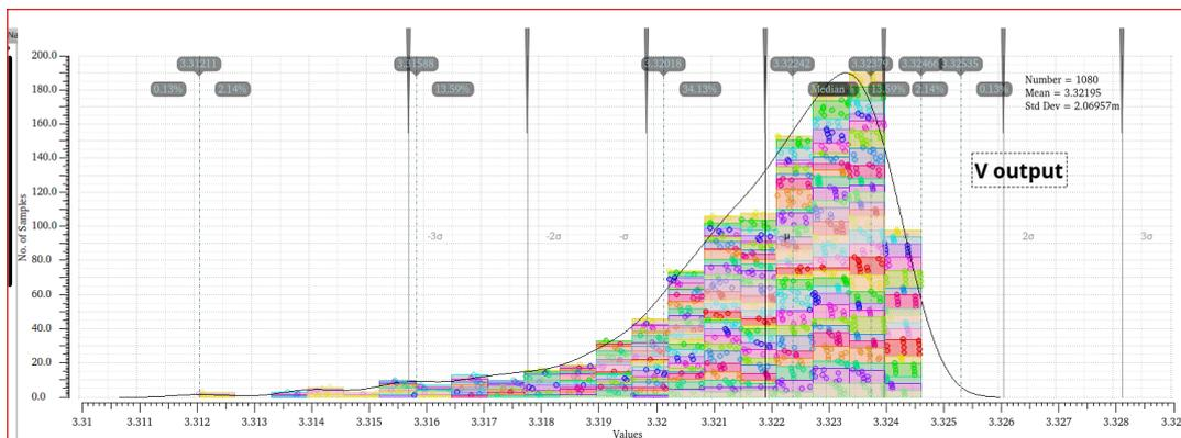
FIGURE 3.24: Histogram of the output voltage with the ideal bandgap across all design points.
