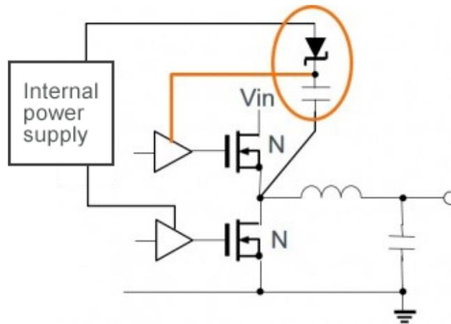
FIGURE 2.5: Example of bootstrap technique applied to a circuit [12]
