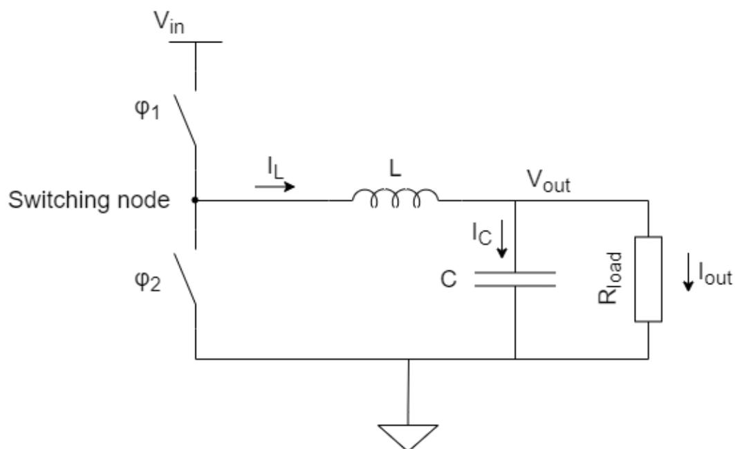
FIGURE 2.1: Architecture of a Buck converter.
