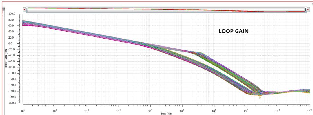
FIGURE 3.21: Loop Gain (dB20) of the circuit with the ideal bandgap across all design points.
