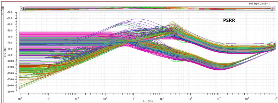
FIGURE 3.18: PSRR vs frequency of the circuit with the real bandgap across all design points.
