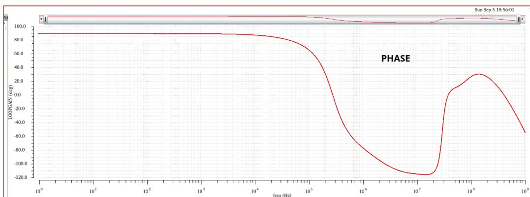
FIGURE 3.12: Phase vs frequency of the circuit with the real bandgap in the nominal case.
