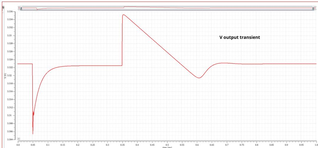
FIGURE 3.29: Transient simulation of abrupt changes in the current load over time.
