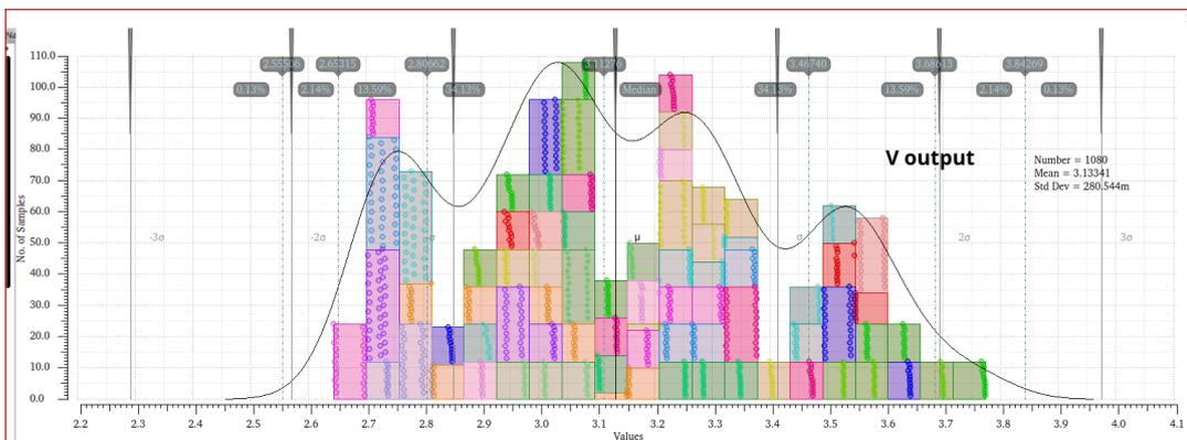
FIGURE 3.19: Histogram of the output voltage across all design points.
