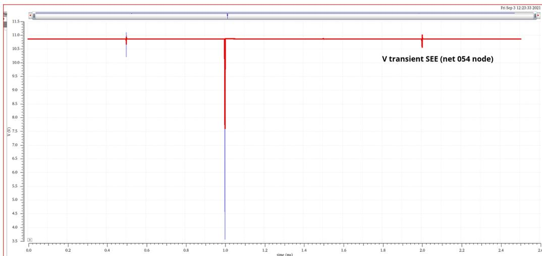
FIGURE 3.34: Comparison of SEE on *net054* node with and without the sink NMOS transistor.
