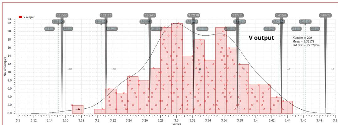
FIGURE 3.15: Histogram of the output voltage following a 200 points MonteCarlo Mismatch simulation.
