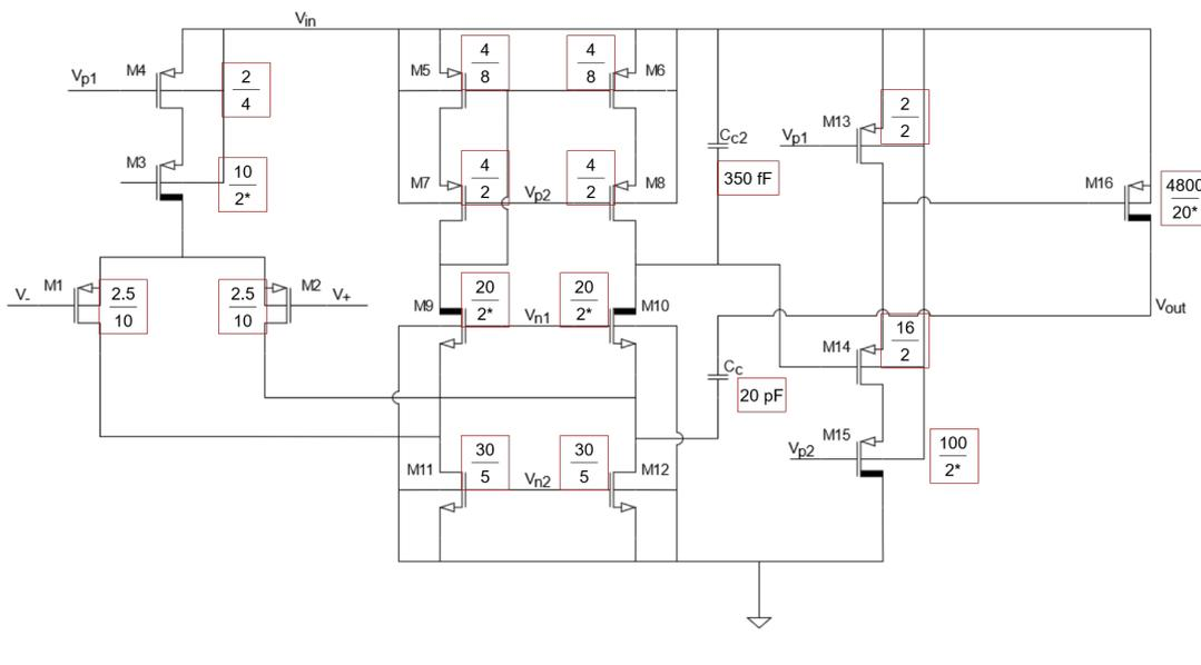
FIGURE 3.5: Transistor sizing of the linear regulator.
