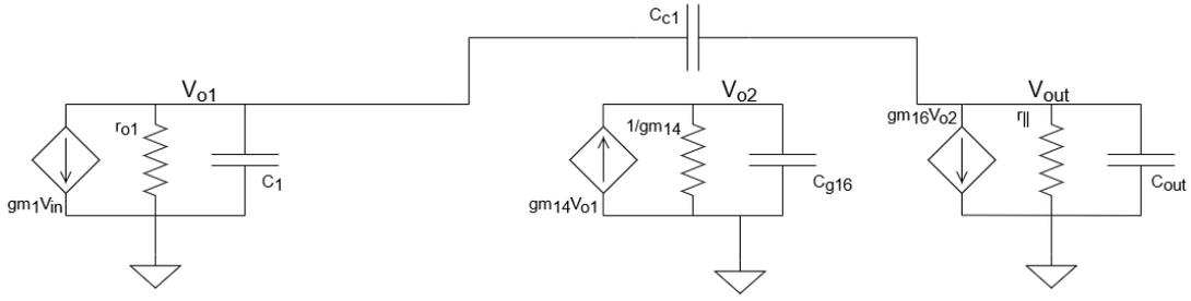
FIGURE 3.10: Small signal simplified representation of the Miller compensated circuit (not implemented).
