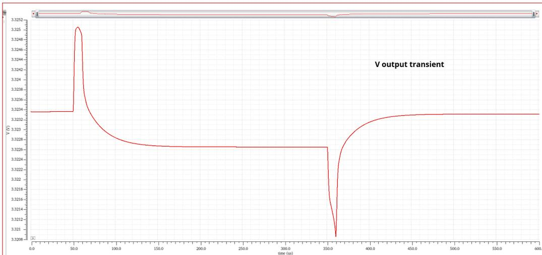
FIGURE 3.27: Transient simulation of abrupt changes in the input voltage over time.
