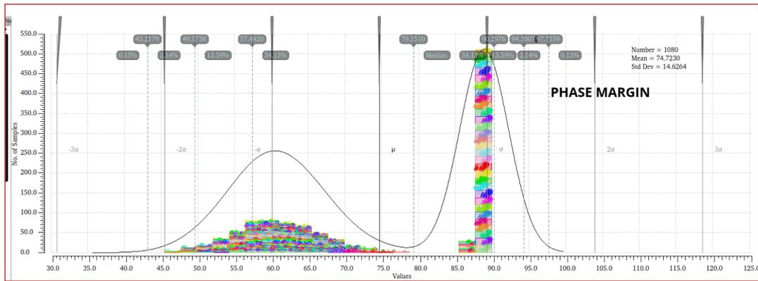
FIGURE 3.25: Histogram of the phase margin with the ideal bandgap across all design points.
