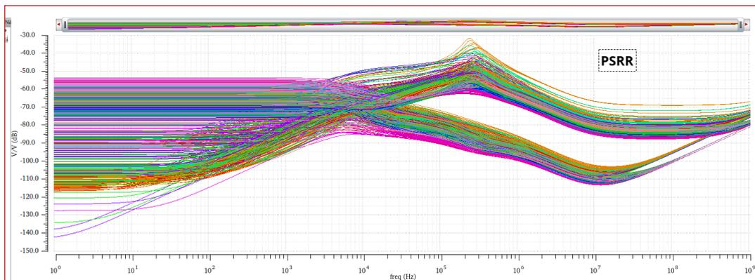
FIGURE 3.23: PSRR vs frequency of the circuit with the ideal bandgap across all design points.
