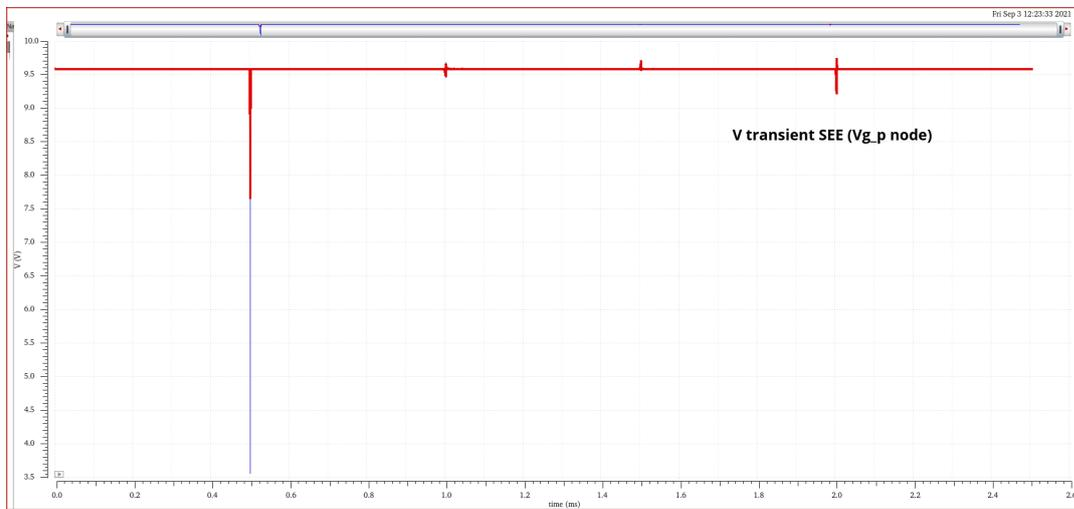
FIGURE 3.33: Comparison of SEE on  $V_{g_p}$  node with and without the sink NMOS transistor.
