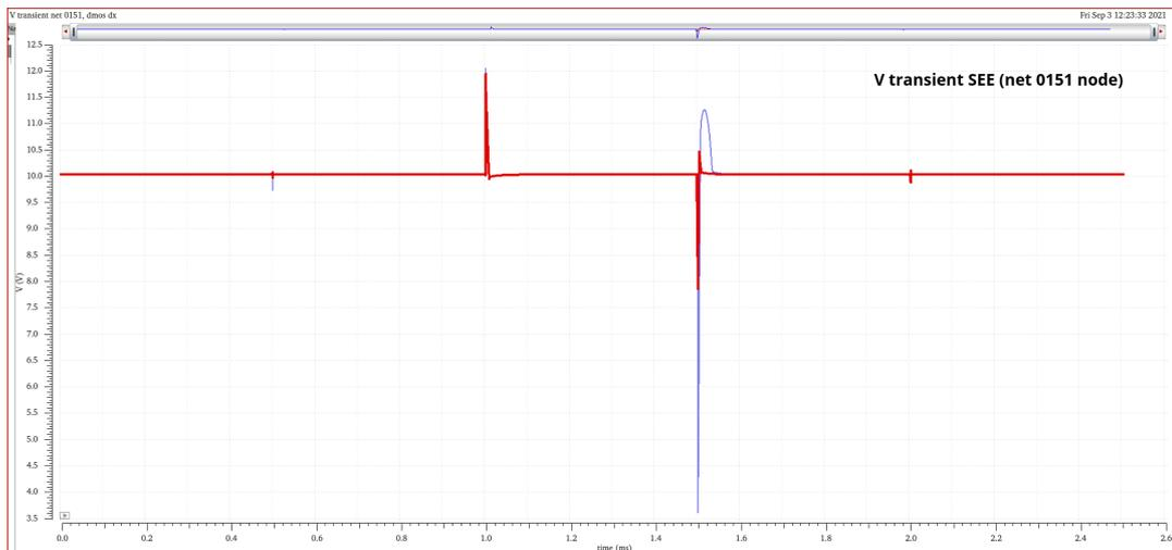
FIGURE 3.35: Comparison of SEE on *net0151* node with and without the sink NMOS transistor.
