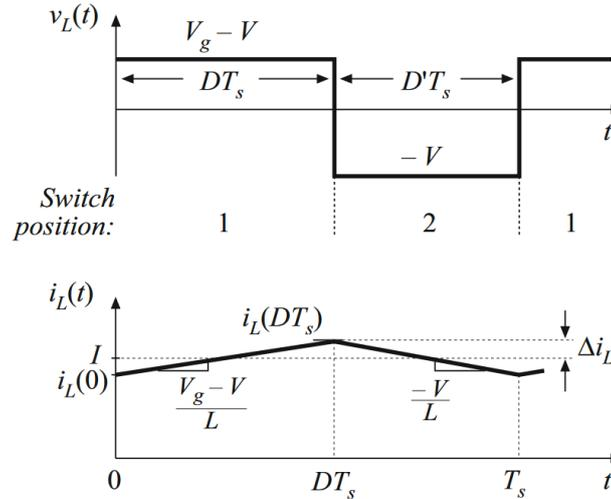
FIGURE 2.2: Voltage and current waveform of the inductor in a Buck converter.
