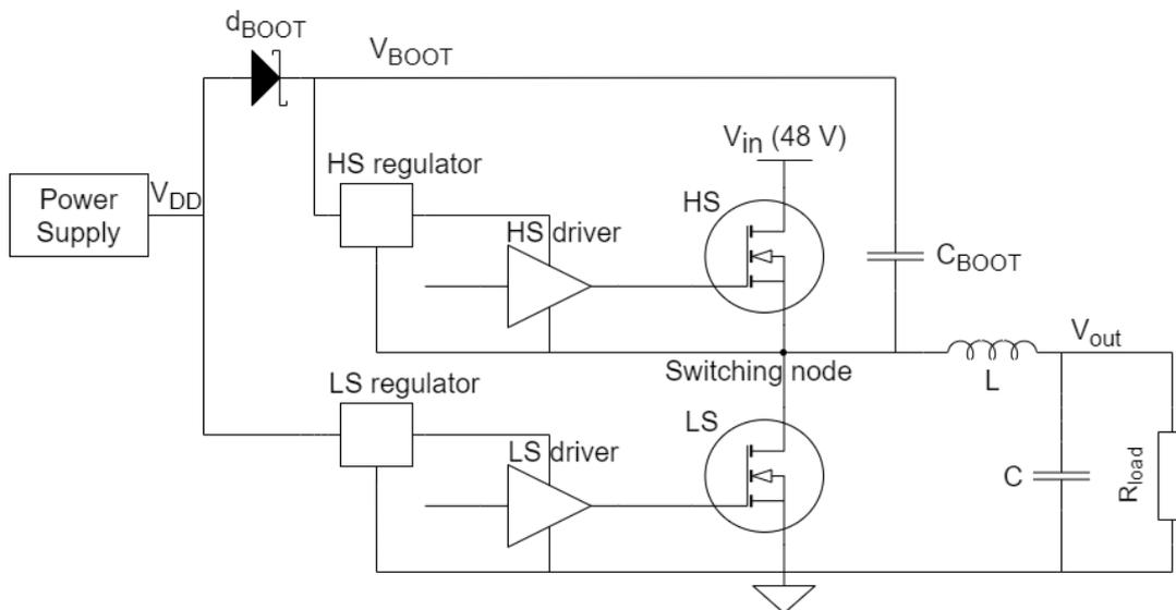
FIGURE 2.8: Schematic of the circuit with the implemented regulators.
