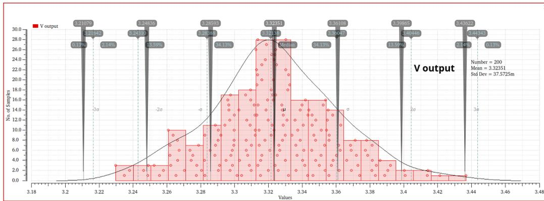
FIGURE 3.14: Histogram of the output voltage following a 200 points MonteCarlo Process simulation.
