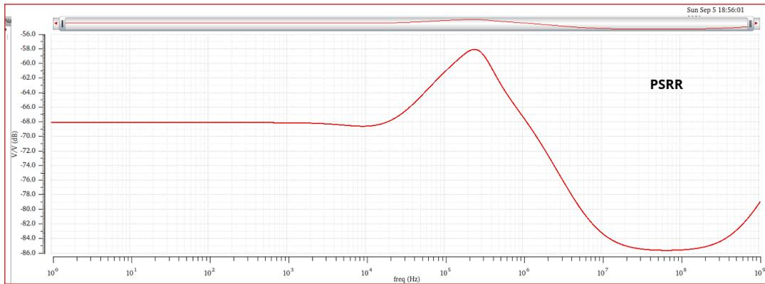
FIGURE 3.13: PSRR vs frequency of the circuit with the real bandgap in the nominal case.
