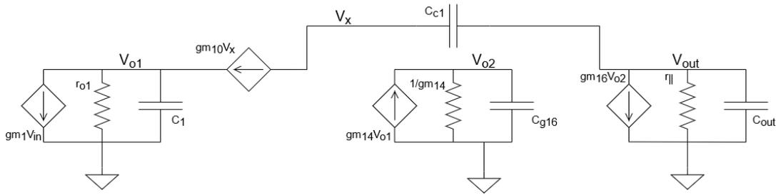
FIGURE 3.8: Small signal simplified representation of the indirect feedback compensated circuit (implemented topology).
