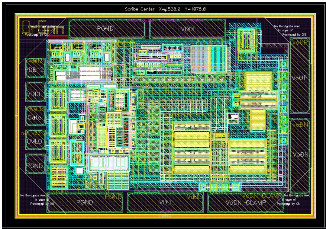
FIGURE 3.39: Screenshot of the final layout of the converter driving circuit.
