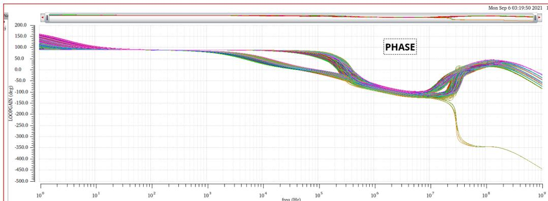
FIGURE 3.22: Phase vs frequency of the circuit with the ideal bandgap across all design points.
