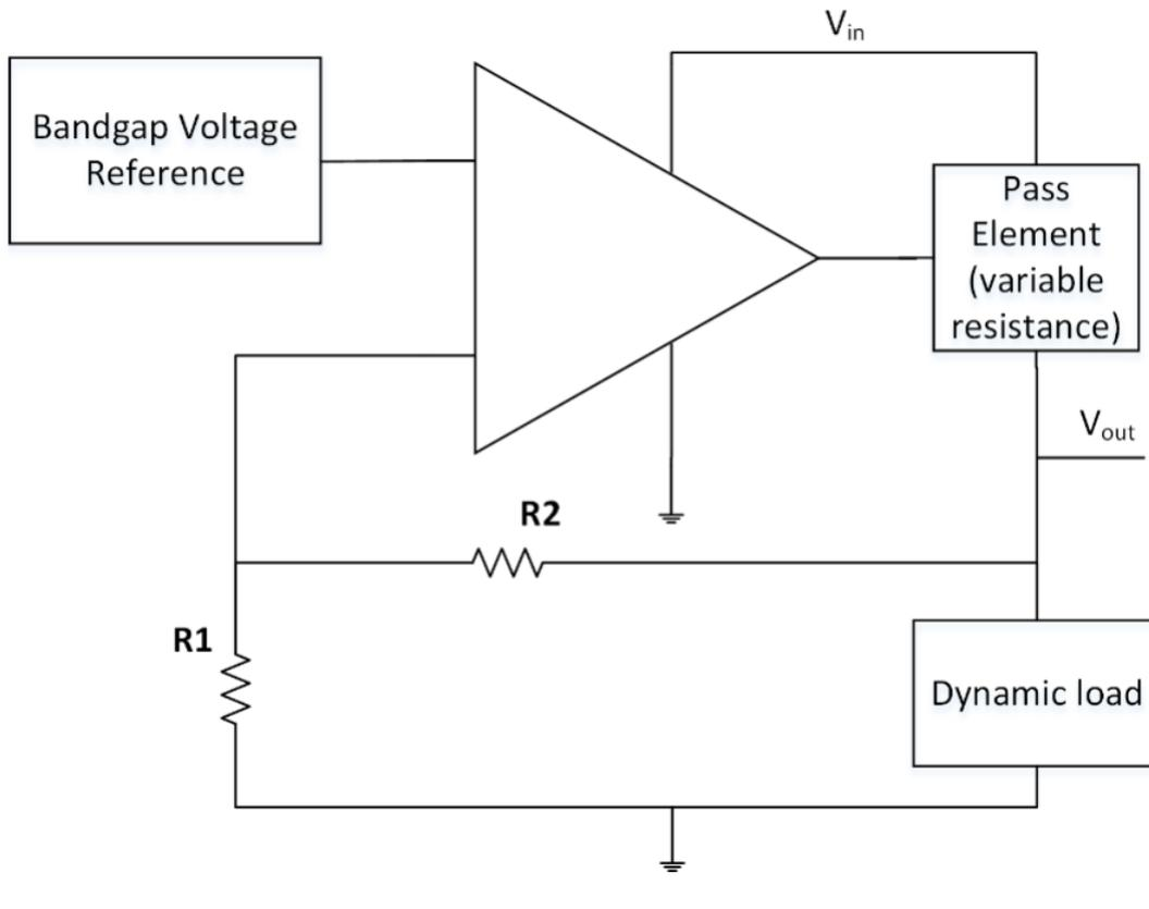
FIGURE 3.1: Schematic of a series linear regulator [17].
