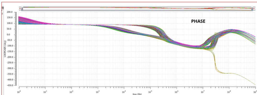
FIGURE 3.17: Phase vs frequency of the circuit with the real bandgap across all design points.
