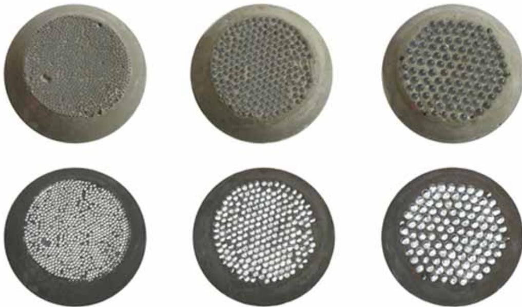
TEST PIECES OF REFLECTIVE CONCRETE WITH AND WITHOUT INCIDENT LIGHT
