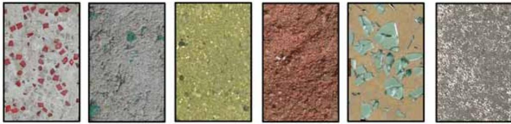
SURFACES' EXAMPLES: CEMENT+PLASTIC, CEMENT+RUBBER, CEMENT+RESINS AND PIGMENTS, CEMENT+METALS AND ALLOYS, CEMENT+GLASS, CEMENT+GLASS MICROSPHERES
