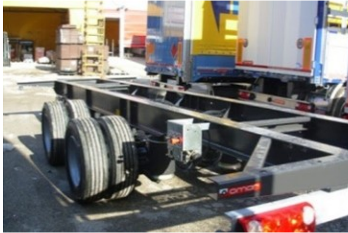
Figure 2.7: Bare chassis biga
