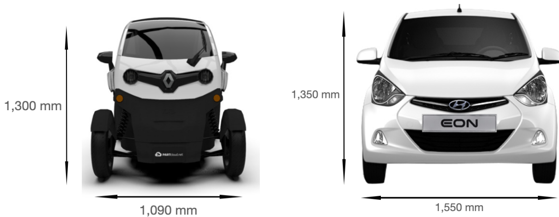
Figure 2.2.2: Front cross-sectional dimensions of a Renault Twizy (Left) and a Hyundai Eon (Right)
