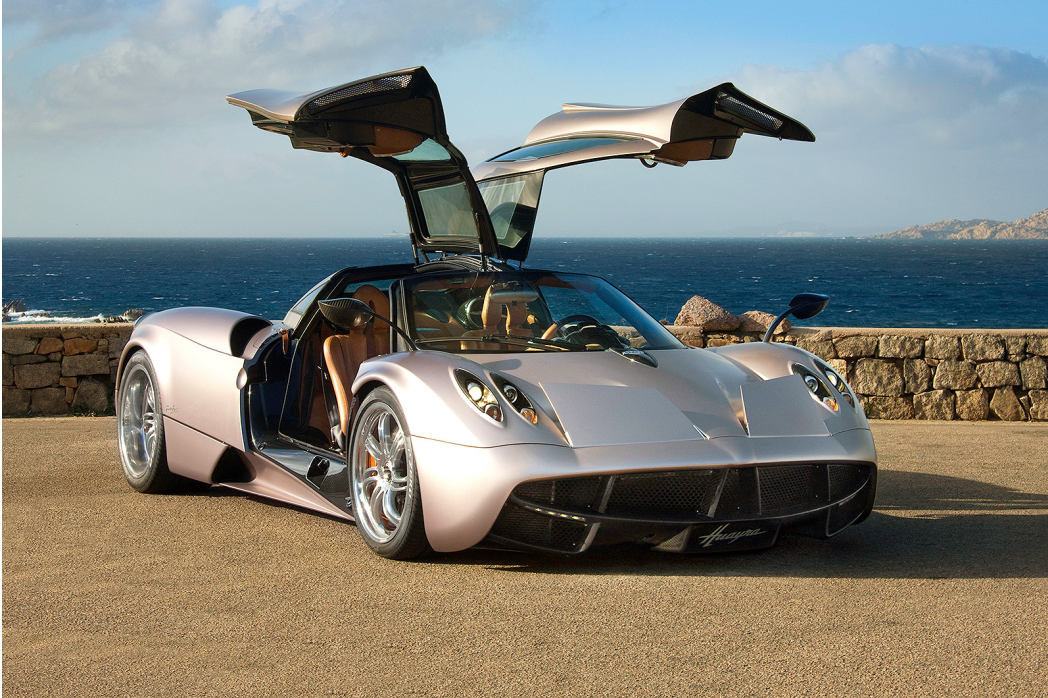
Figure 2.1.1: Gull wing doors on a Pagani Huayra [41]
