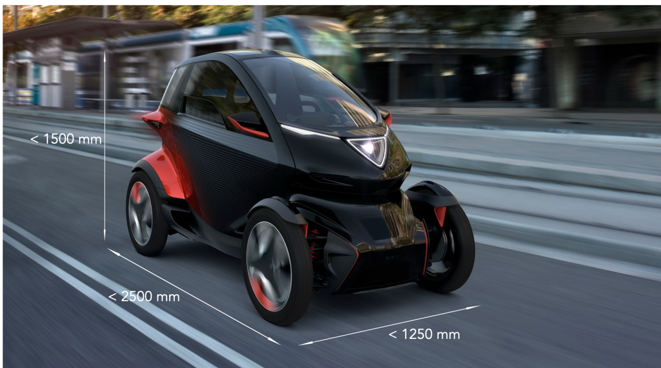
Figure 2.2.1: Suggested dimensions for the quadricycle
