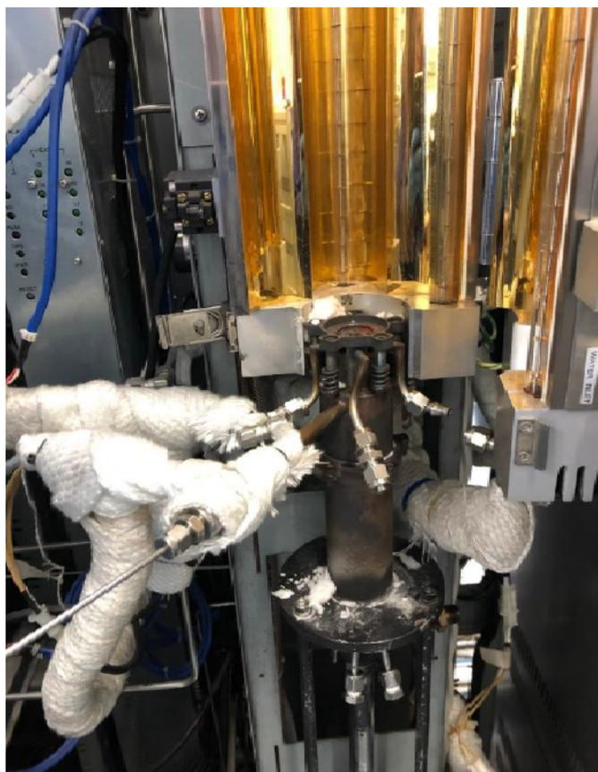
**Figure 2.2:** Reactor unit with pre-heating quartz tube removed from furnace and mixing plate exposed
