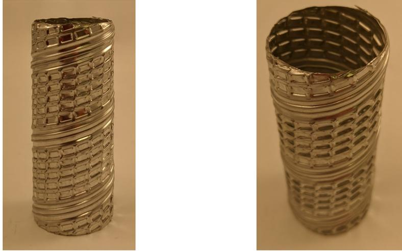
**Figure 6.1:** Perforated support of the real filter
