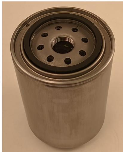
**Figure 7.4:** Experimental Oil Filter
