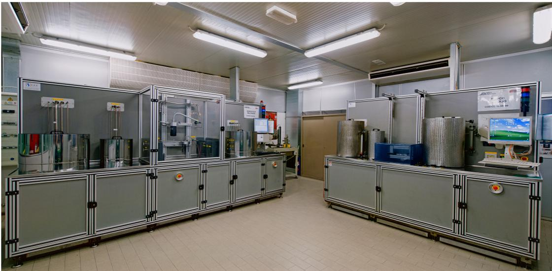
**Figure 7.1:** DELGROSSO S.R.L Multipass Test bench
