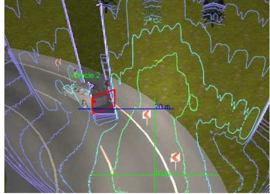
(b) When the vehicle enters the corner, glare is created, corresponding to the first peak in Figure 24.
