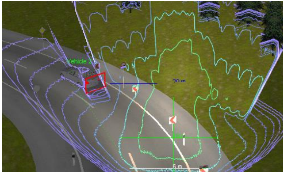
(c) When the stimulus vehicle exit the high beam area, there is a short time when glare drops to zero, corresponding to the area between two peaks in Figure 24.
