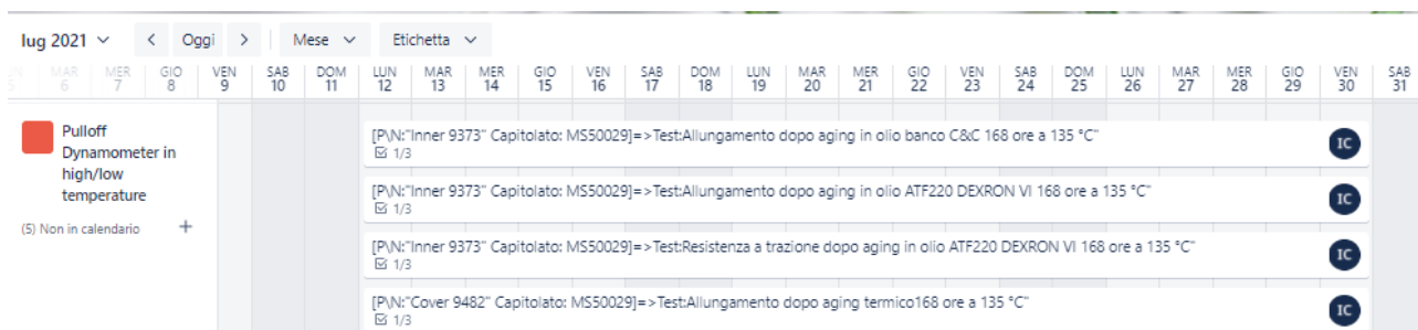
Fig. 28 Wrong way of scheduling test over one machine: overlapping tests involving the same machine
