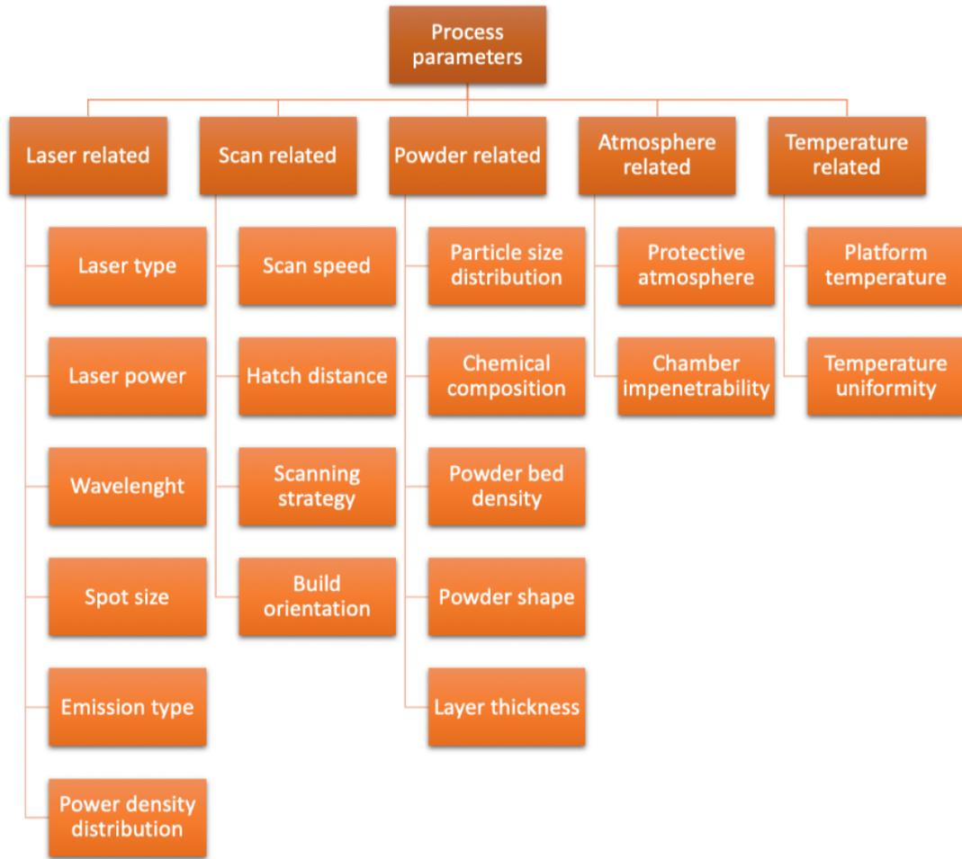
Figure 2.2: Principal process parameters
