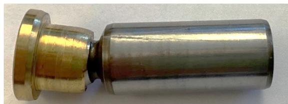
Figure 10: cylinder damage (oil contamination)
