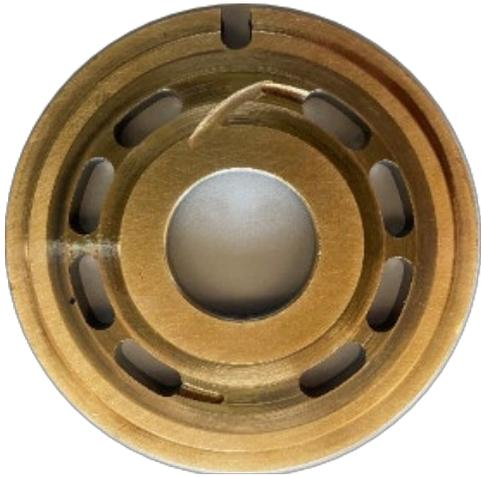
Figure 57: extremely damaged valveplate
