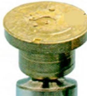
Figure 28: lack of lubrication damaged slipper
