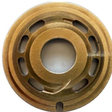
Figure 30: Extremely damaged valve plate
