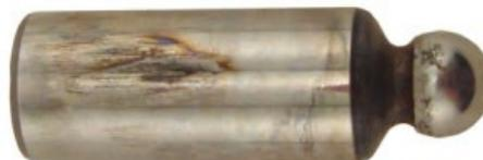
Figure 9: cylinder damage (lack of lubrication)
