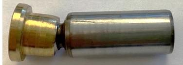
Figure 27:piston damaged by oil contaminants
