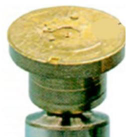
Figure 7: lack of lubrication damage
