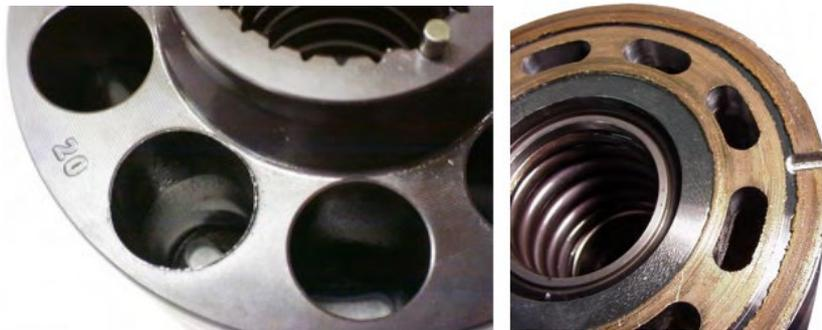
Figure 12: cylinder block damage (lack of lubrication)
