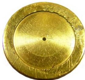
Figure 6: oil contamination damage
