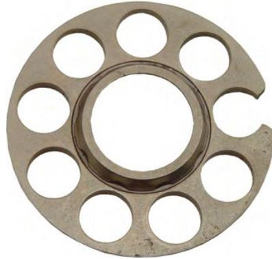
Figure 11: slipper retainer damage
