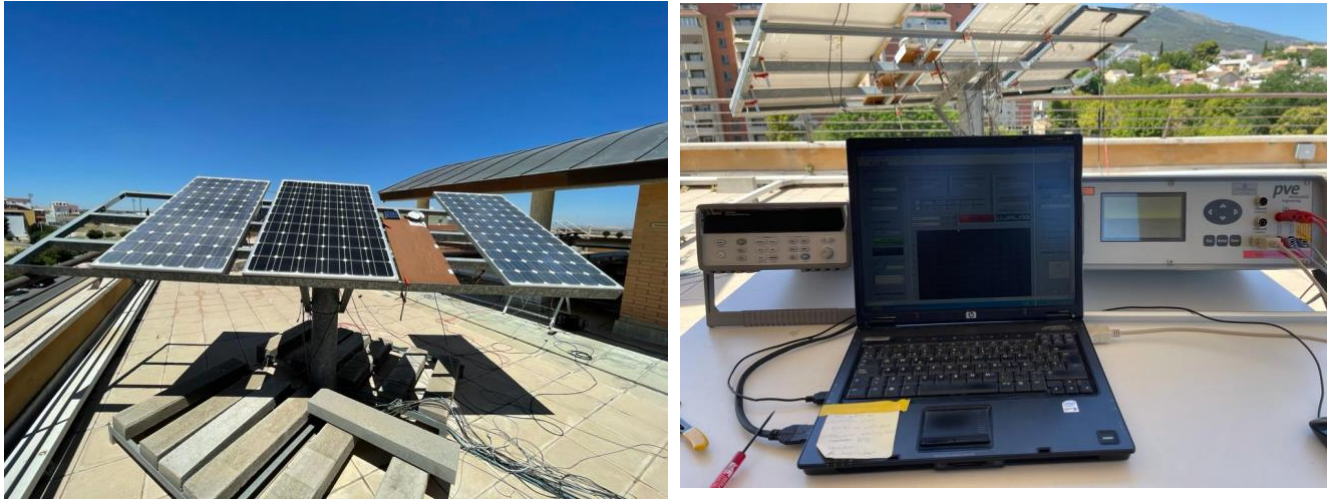
Figure 3-11: (Left) Fixed system connected with (Right) PVPM and data logger controlled by LabVIEW program.
