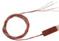
Figure 3-14: Pt-100 probe used to measure module temperature.
