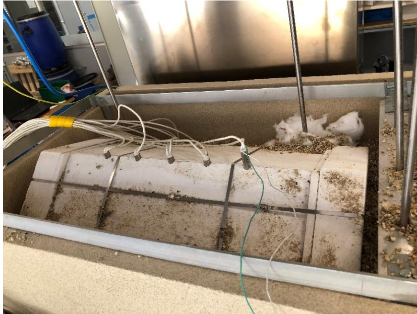
Figure 5: Photo of the box which contains the air electrical heaters to heat-up the inlet air in the stack.
