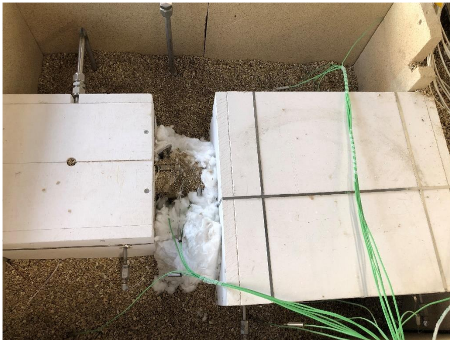
Figure 4: Photo of the boxes in which are contained the heat exchangers of the ComESto system, which transfer heat from the outlet streams from the stack to the inlet ones.
