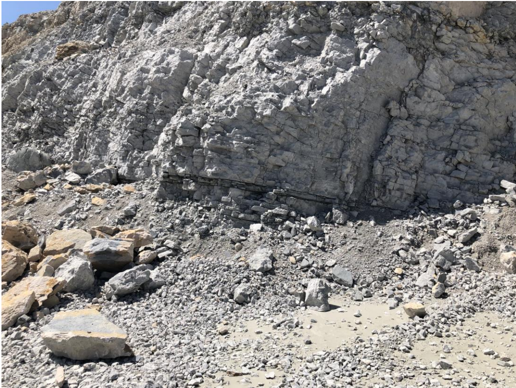
Figure 4.4 – Area of weakness on the West face of Faraona quarry (July 2021).
