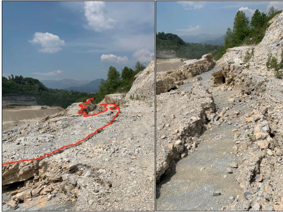
Figure 4.8 – Tension crack in the left. Planar sliding in the right (Griffini 2020).
