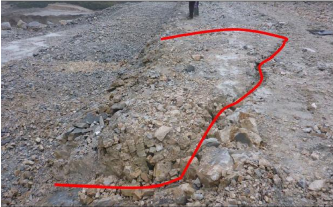
Figure 4.7 – The red line describes the trend of the new tension crack in the East zone (Griffini 2018).
