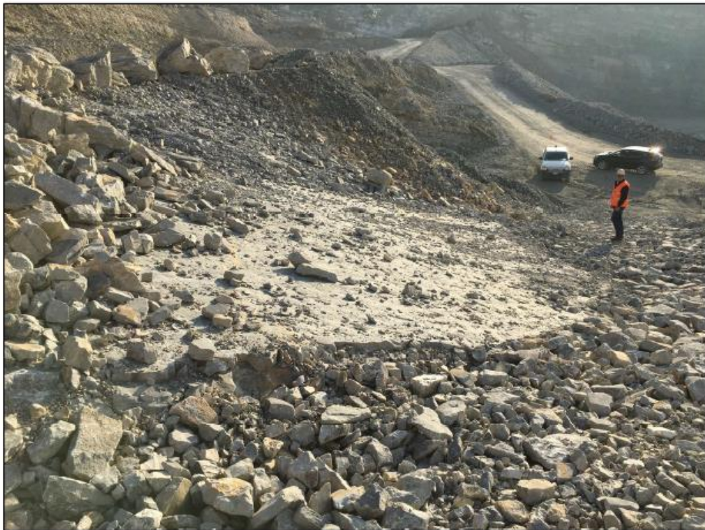
Figure 4.5 – Planar sliding of the material occurred in 2017 (Griffini 2018).
