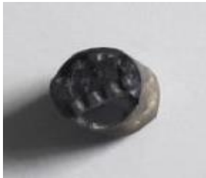
Figure 3.8 - Sample 3, completely worn PCD tool
