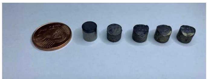
Figure 2.8 - PCD tools. The first tool is new, the others are damaged and unusable
