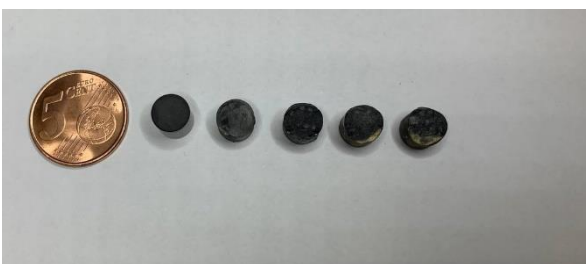
Figure 2.8 - PCD tools. The first tool is new, the others are damaged and unusable
