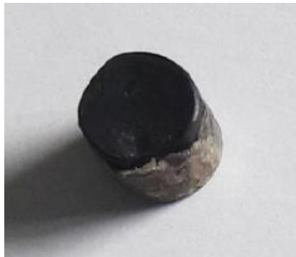
Figure 3.4 - Sample 2, chipped PCD tool
