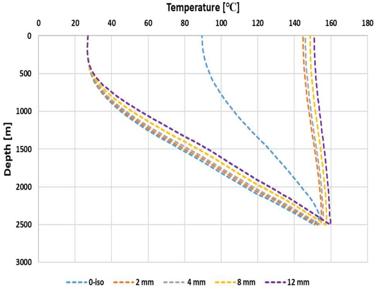
**Fig.25** Effect of the insulation thickness
