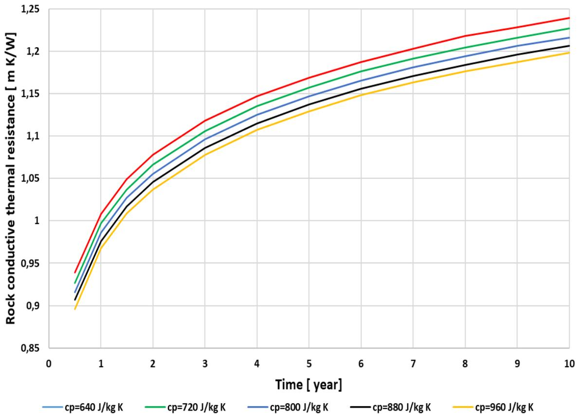
**Fig.19** Soil resistance within years depending on the rock specific heat
