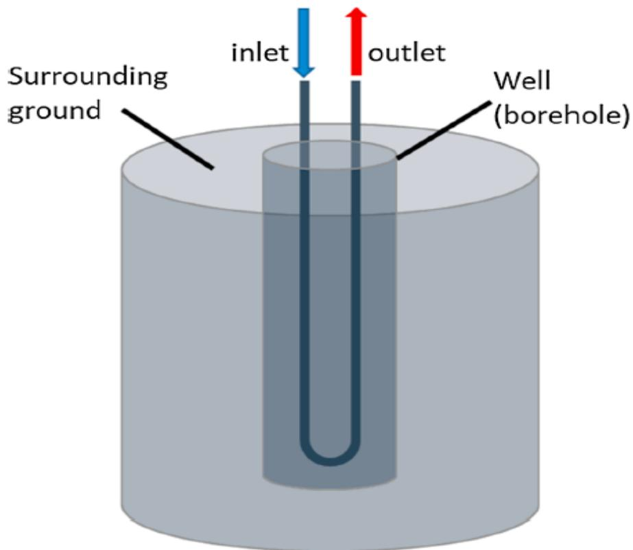
**Fig.7** Scheme of Vertical U-tube heat exchanger [35].
