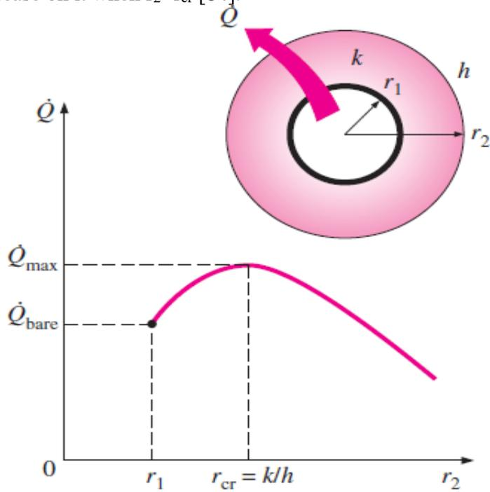
**Fig.14** Variation of heat transfer rate with  $r_2$ , outer radius of insulation when  $r_1 < r_{cr}$  [84].
