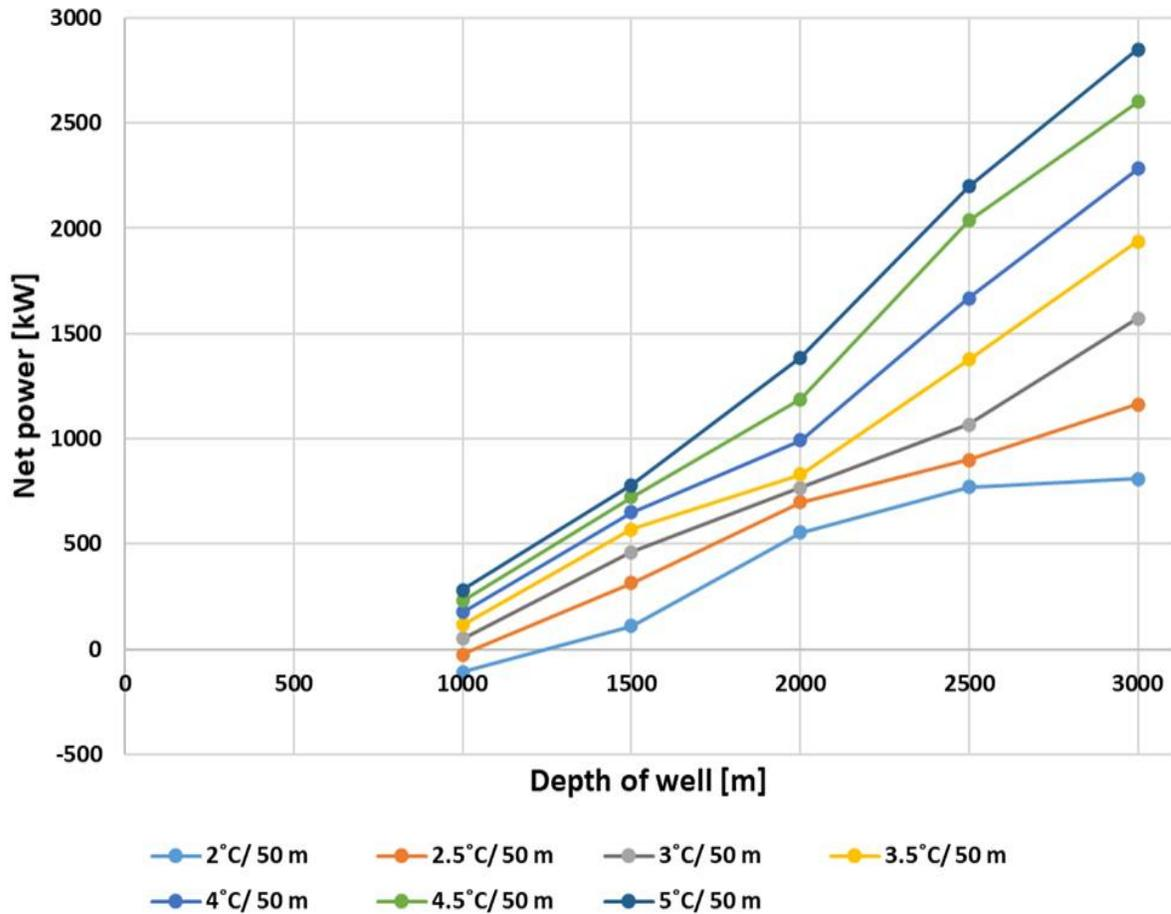
**Fig.24** Effect of the geothermal gradient and the depth of DHE to the net power. (Working fluid: R134a,  $m_{\text{fluid}} : 30 \text{ kg/s}$ ,  $\Delta T : 3^\circ\text{C}/50\text{m}$ ,  $c_{p\text{rock}} : 800 \text{ J/kg K}$ ,  $\rho_{\text{rock}} : 2600 \text{ kg/m}^3$ ,  $k_{\text{rock}} : 2.5 \text{ W/m K}$ )
