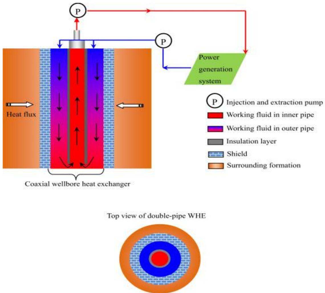
**Fig.8** Schematic diagram of geothermal power generation using AOGW [23].
