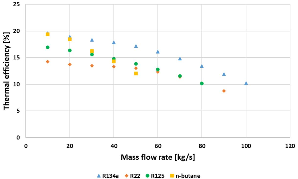
**Fig.29** The thermal efficiency depending on mass flow rate
