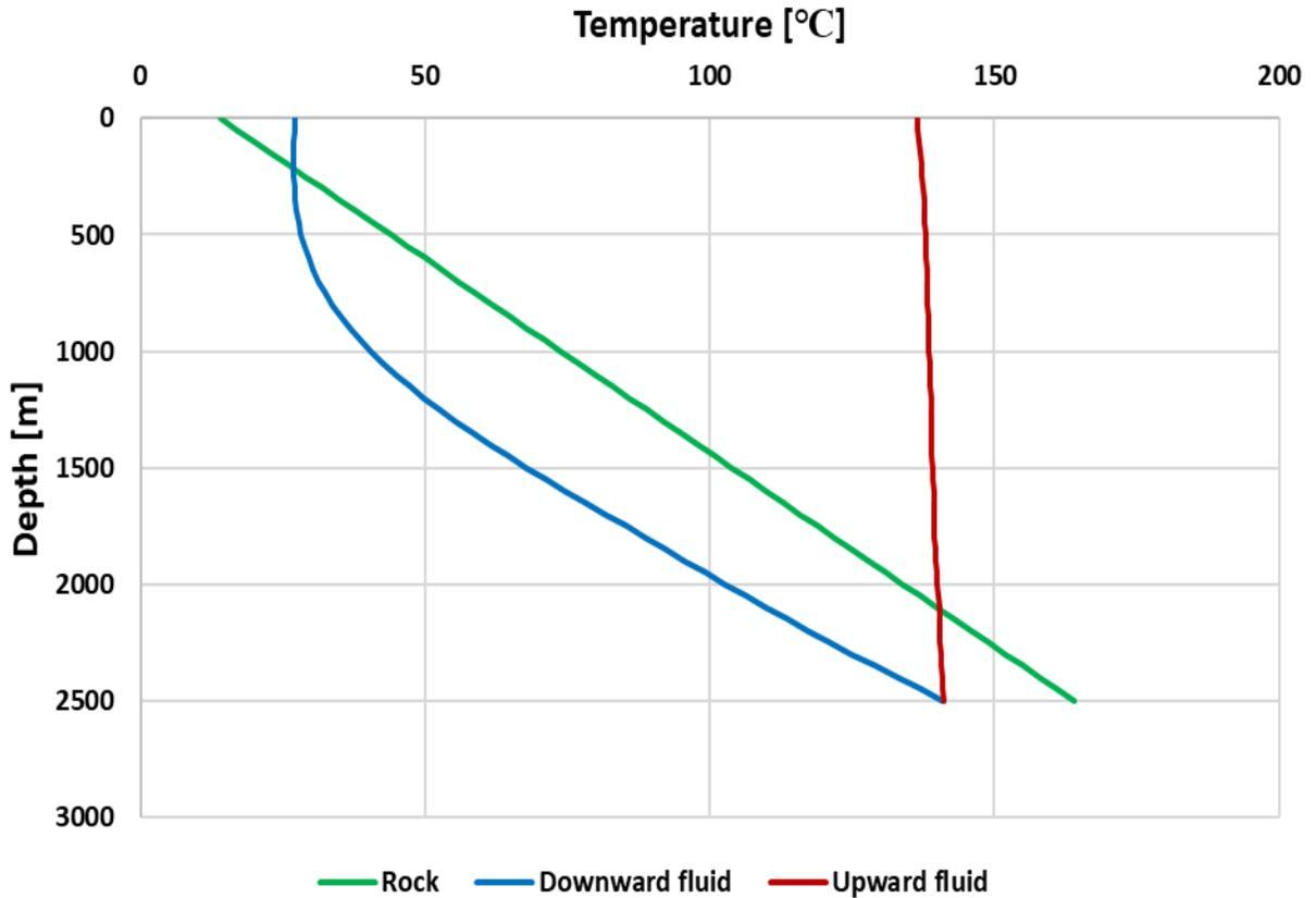
**Fig.23** The profile of temperature through the well
