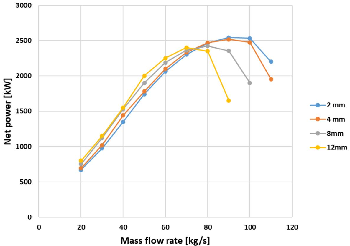
**Fig.26** Effect of insulation thickness on the mass flow rate
