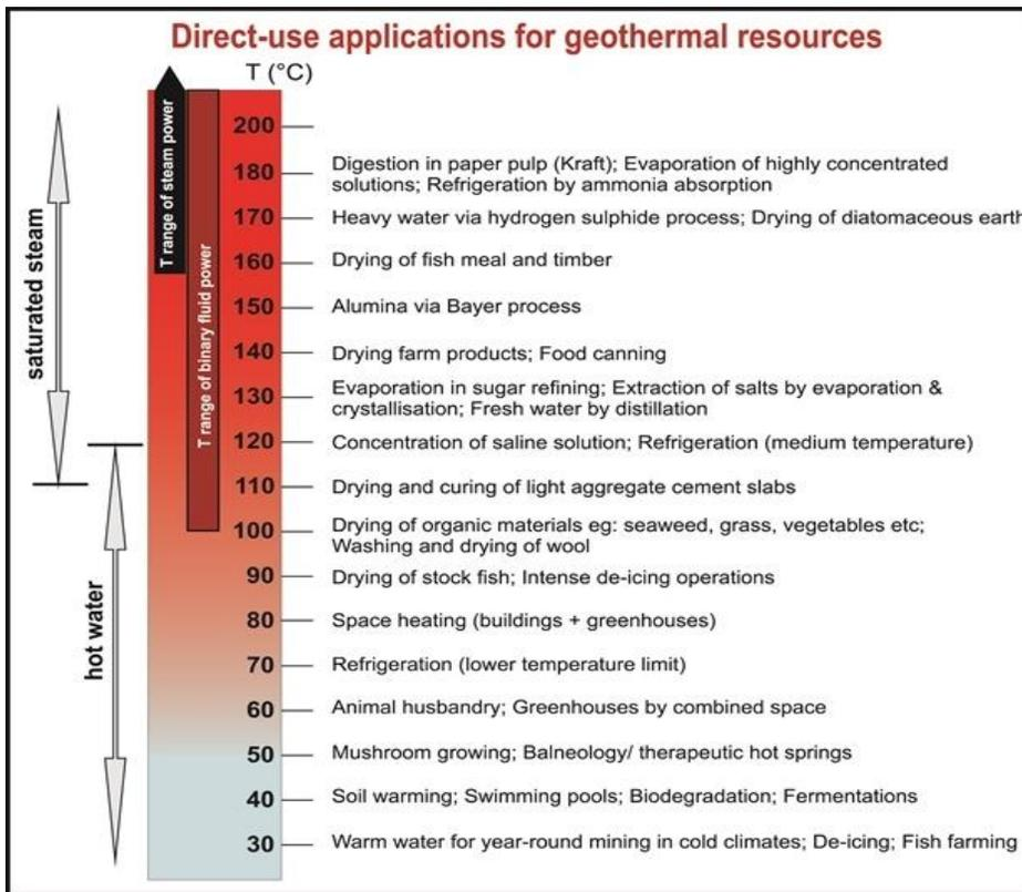
**Fig.1** The Lindal diagram shows that a range of applications for different temperature geothermal resources [5].
