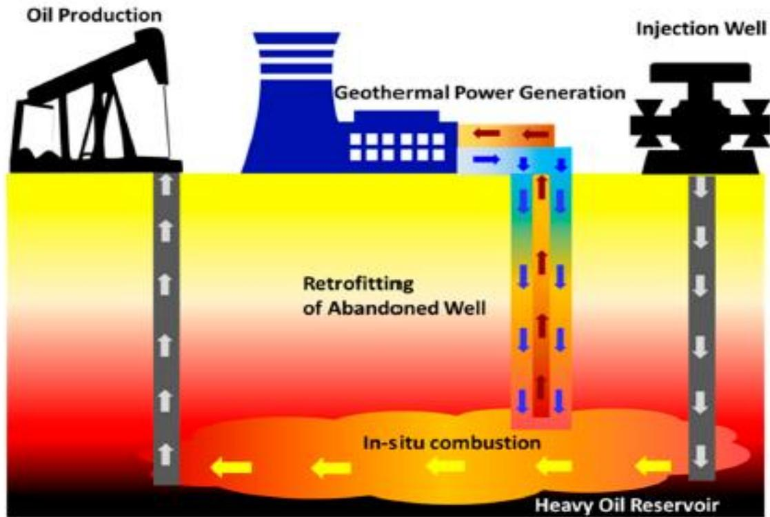
**Fig.11** The scheme of utilizing in situ combustion system for abandoned wells [72].
