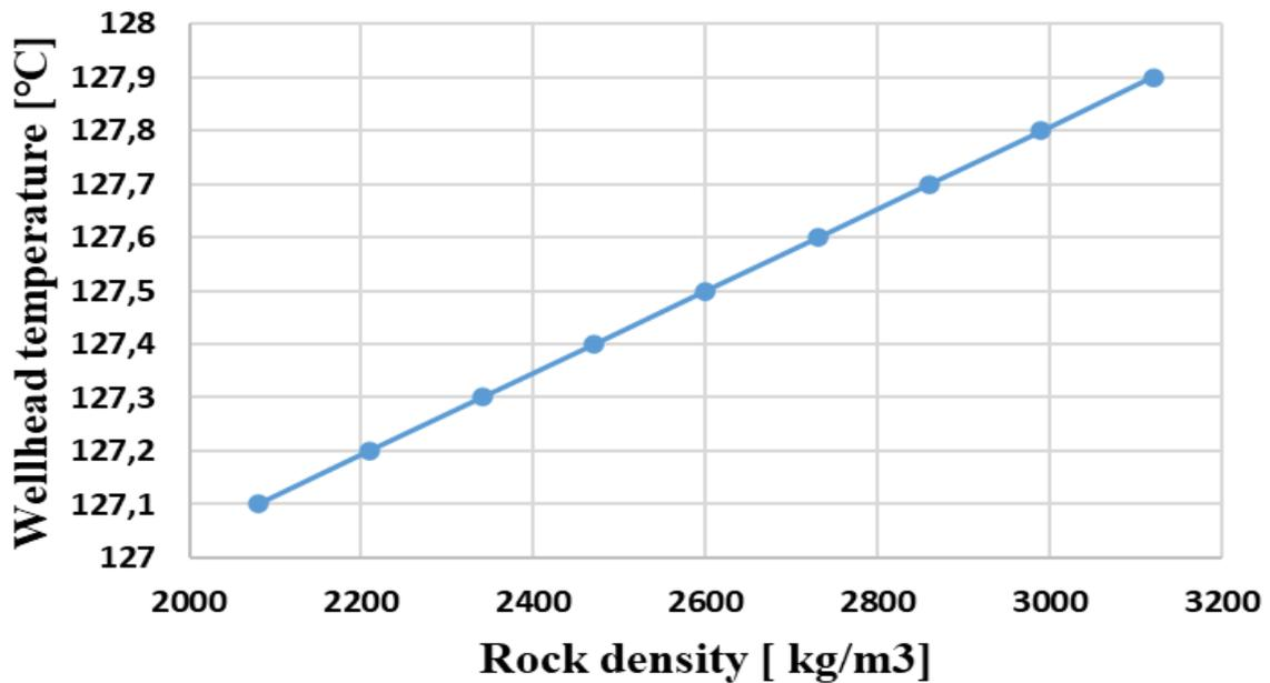
**Fig.18** Dependence of the wellhead temperature from rock density
