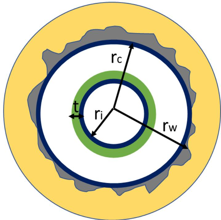
**Fig.13.**The cross section of wellbore heat exchanger (Add reference).
