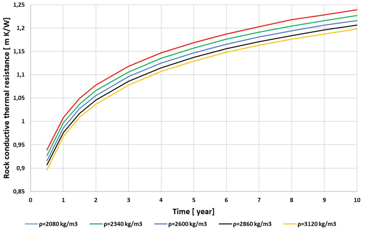
**Fig.17** Soil resistance within years depending on the rock density
