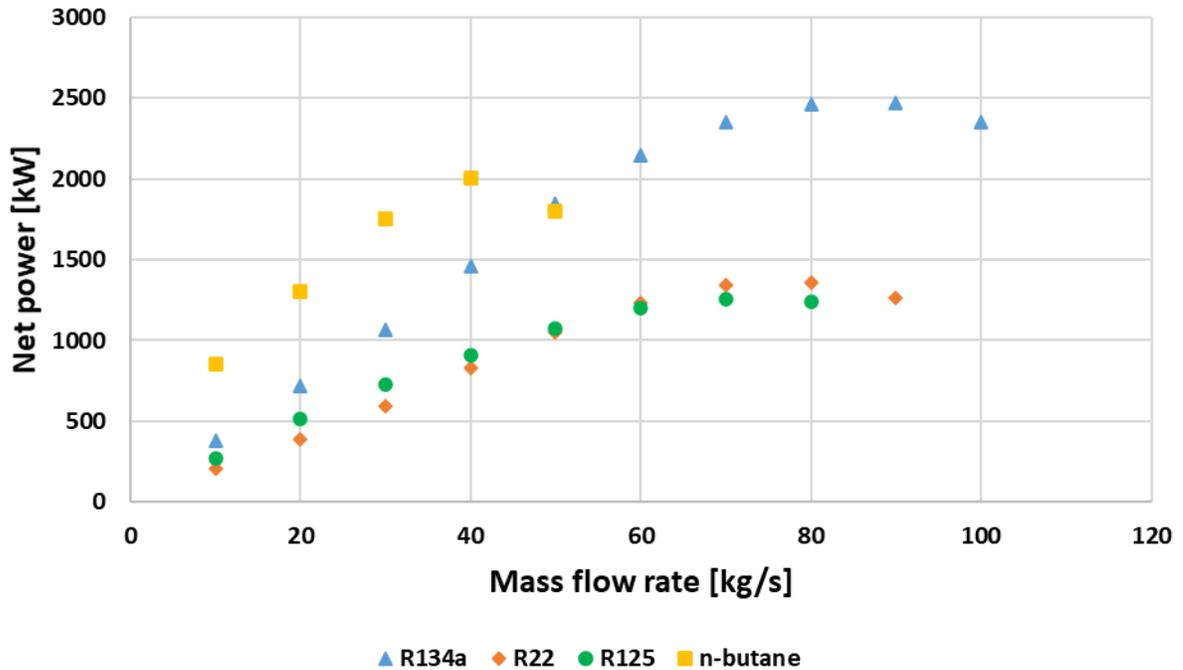
**Fig.28** The net power for different working fluids
