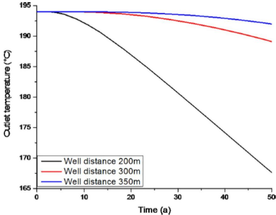
**Fig.10** The average outlet temperature with various distances (m) between the production and injection wells [71].
