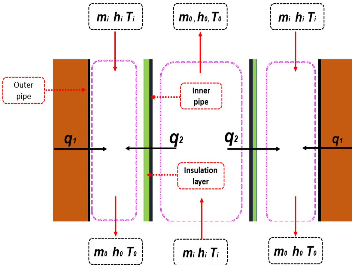
**Fig.15** The chart of the heat flow of the system
