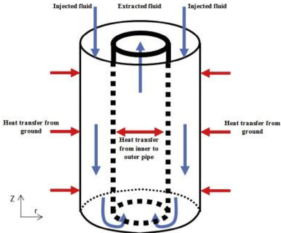
**Fig.9** Scheme of a double pipe heat exchanger which can be applied to a hydrocarbon well [24].
