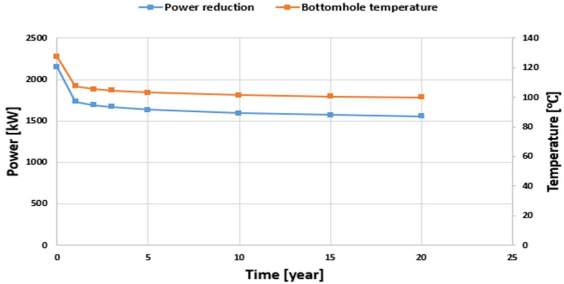
**Fig.27** Power reduction and bottomhole temperature depending on time
