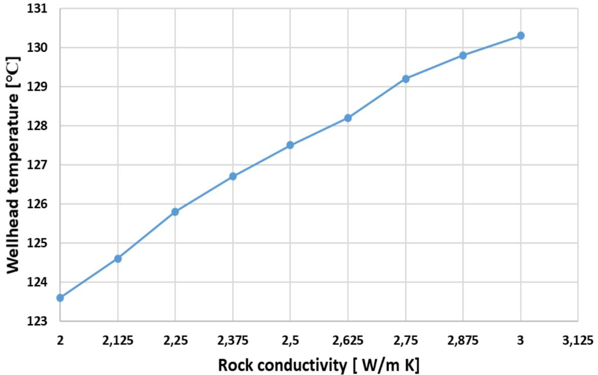
**Fig.22** Effect of rock conductivity on wellhead temperature
