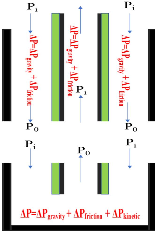
Fig.16 Pressure drops within the downhole heat exchanger
