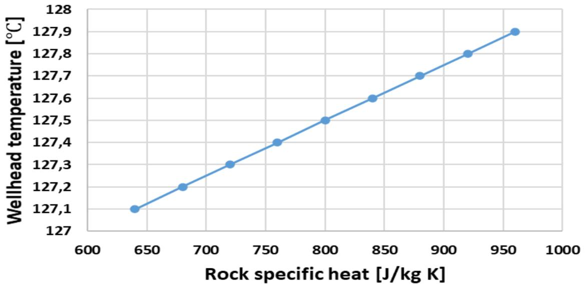
**Fig.20** Dependence of the wellhead temperature from rock specific heat.
