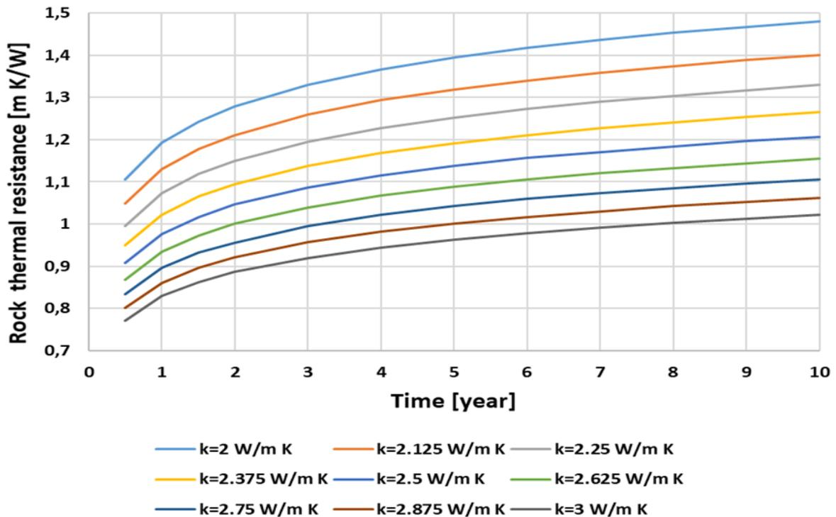
**Fig.21** Soil resistance within years depending on the rock conductivity
