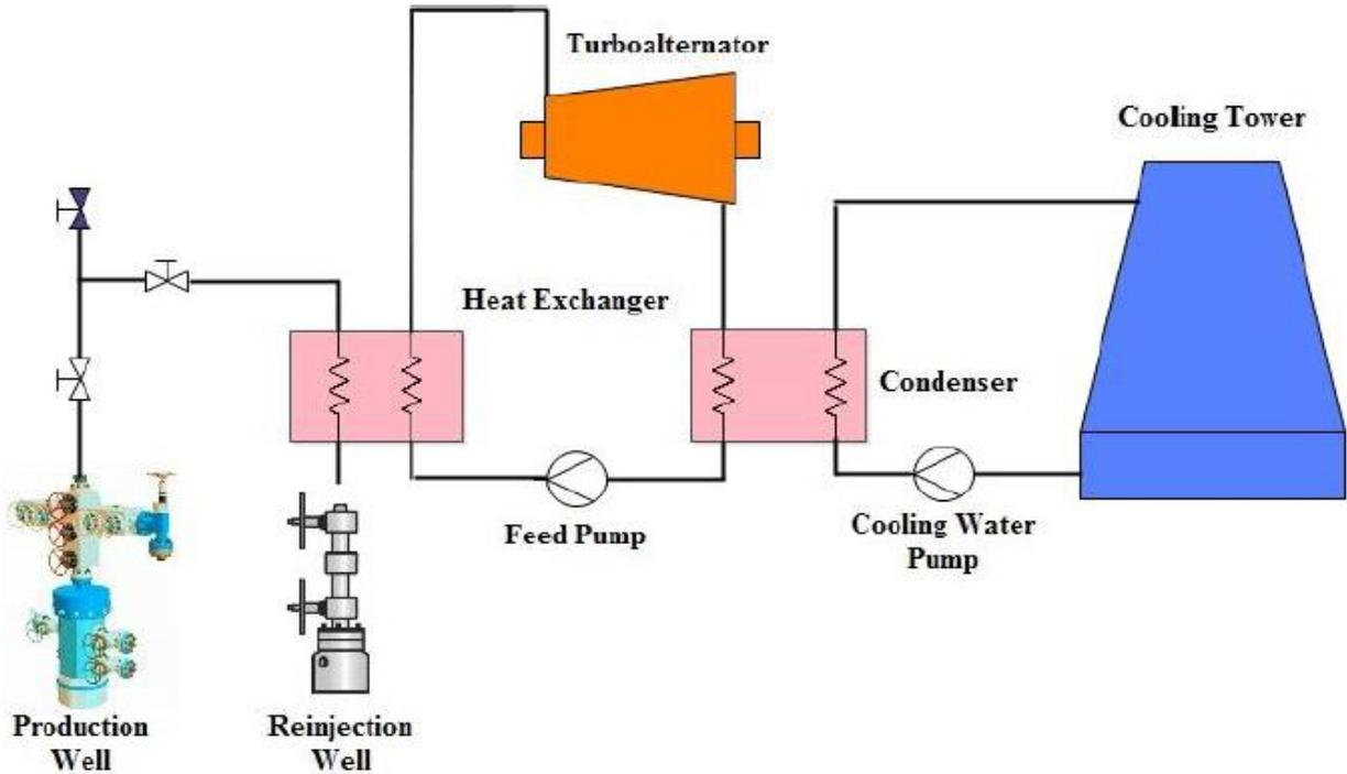
**Fig.6** Binary cycle geothermal plant [34].
