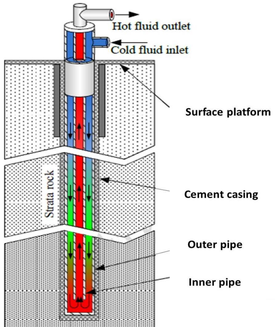
**Fig.12** The scheme of double-pipe downhole heat exchanger.
