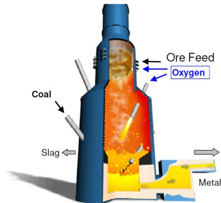
Figure 2.2. Graphical representation and schematics of HIsarna process [22]
