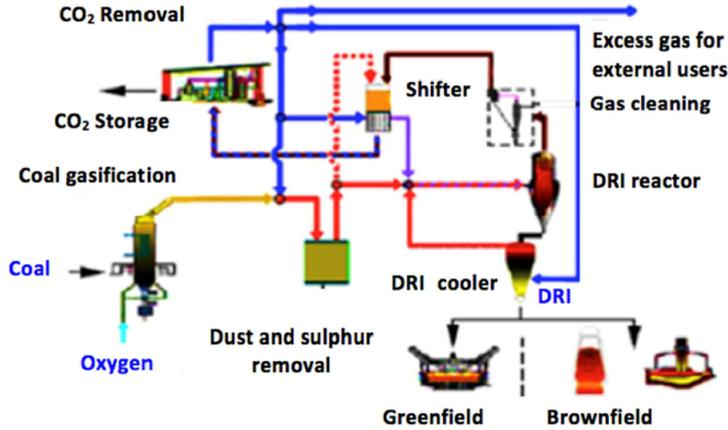
Figure 2.5. ULCORED process schematics [26]
