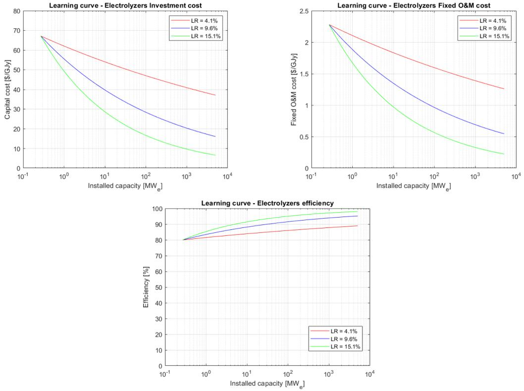
Figure 3.13. Electrolysis: Investment cost, Fixed O&M costs and efficiency
