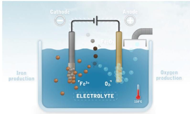
Figure 2.8. Electrowinning cell simplified scheme [36]
