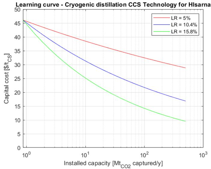
Figure 3.12. Cryogenic distillation CCS learning curve
