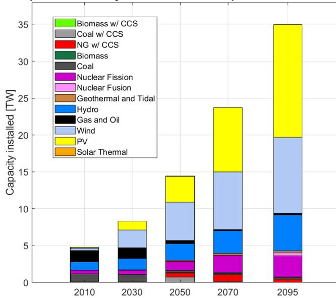
Figure 4.1. Power plants capacity installed per source in five milestone years
