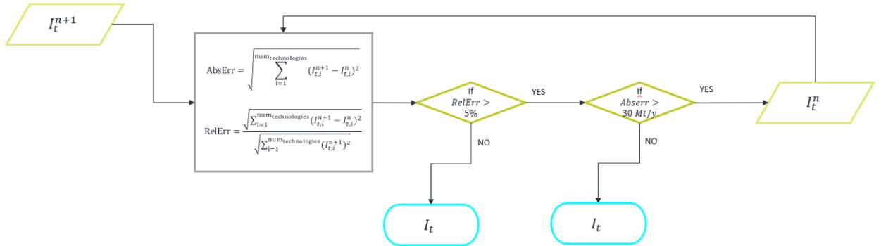
Figure C.3. Convergence criterion for steelmaking technologies
