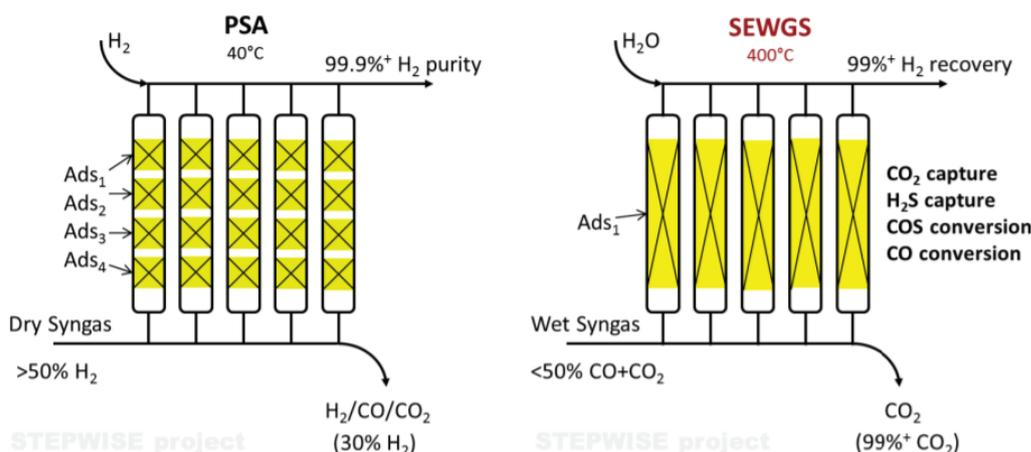
Figure 2.3. Compared PSA and SEWGS adsorbing processes [45]
