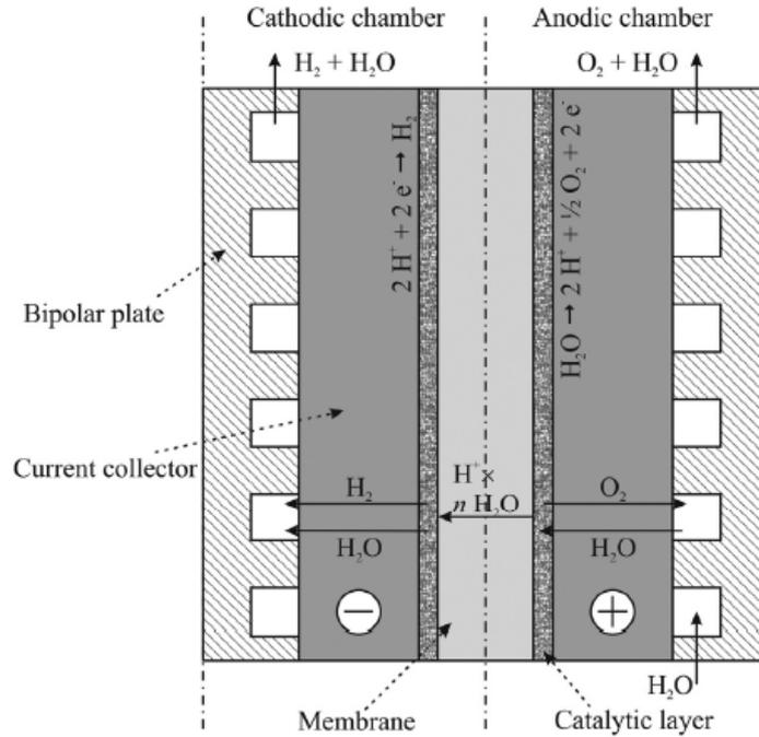
Figure 2.7. Scheme of the principle of the PEM electrolysis cell [62]
