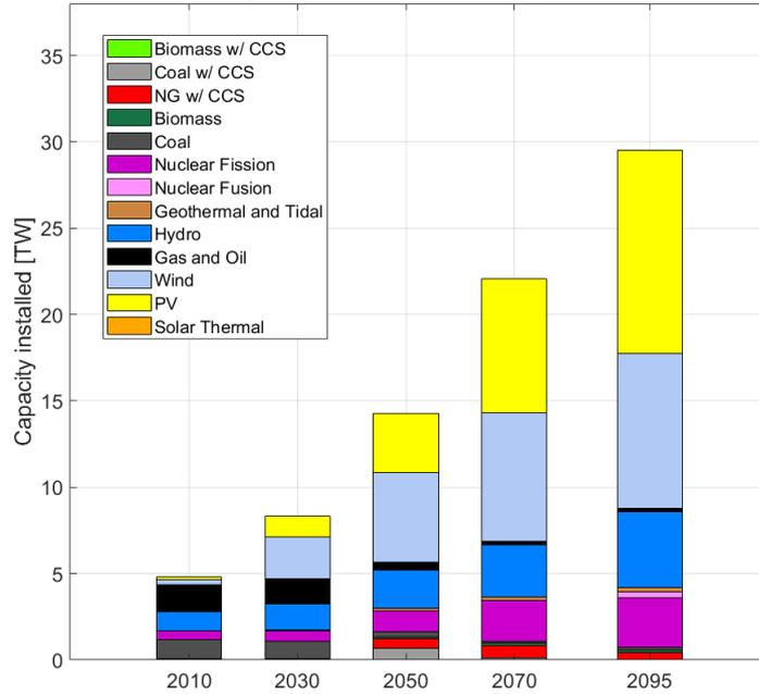
Power plants installed by source - with sector-specific emissions constraints
