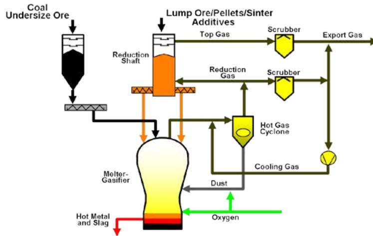
Figure 2.1. Smelting reduction process [21]
