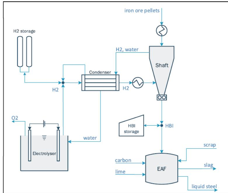
Figure 2.6. Schematic of the HDR-EAF process design [29]
