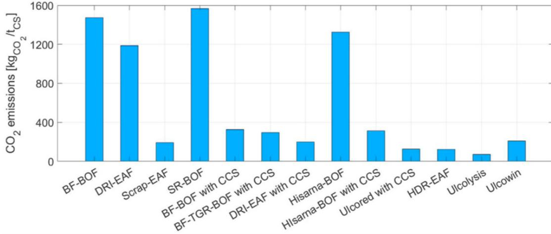
Figure 3.8. Emissions related to each steelmaking process [19]
