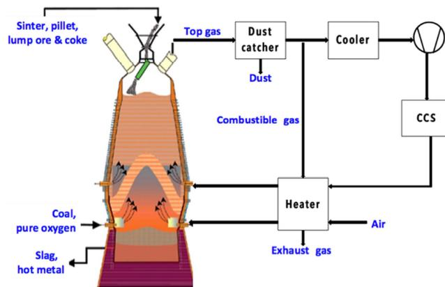
Figure 2.4. Simplified scheme of the BF-TGR-BOF process [26]
