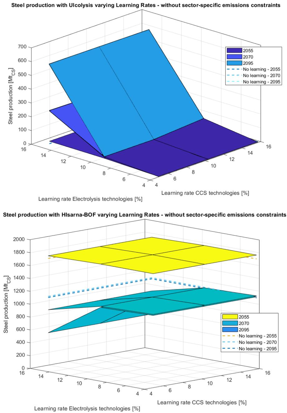
Figure 4.7. Production rates for Ulcolysis and Hisarna-BOF varying the LRs
