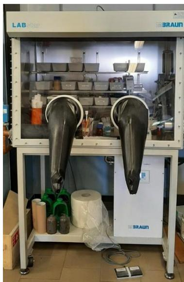
Figura 3.5 Glovebox MBraun® Labmaster Pro.
