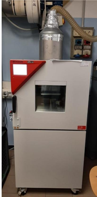
Figura 3.11 Camera climatica Binder<sup>®</sup> MKF 56.
