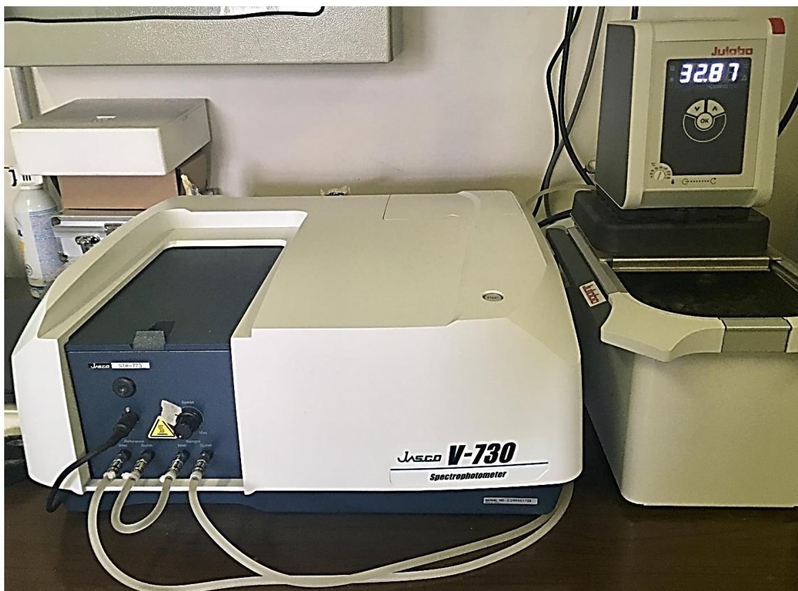
Figure 3.4 Picture of the spectrophotometer Jasco V-730 involved in all the absorbance tests within this thesis work; on the right, the thermostatic water bath is visible with the piping system that brings water to the spectrophotometer chamber.
