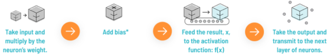
Figure 4.7: The process implemented by a neuron in a neural network. The image was taken from [64].
