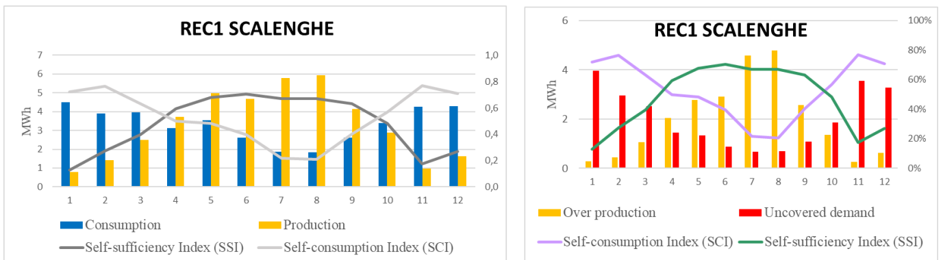
Figure 66 REC1 shows the correlation between consumption, production and self-consumption and self-sufficient (left), the aggregation between over production, Uncovered demand and self-consumption and self-sufficient (right)
