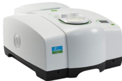
**Figure 3.4.** ATR-FTIR Frontier FT-IR Perkin Elmer.
