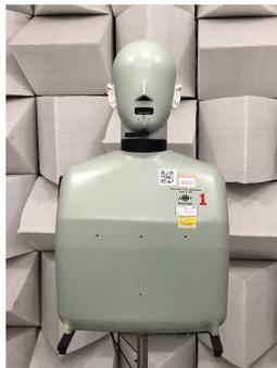
**Figure 3.17:** Pictures of HATS - frontal view in the anechoic chamber.
