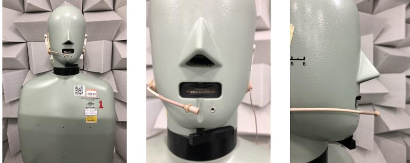
**Figure 3.22:** Microphone in air aligned with the screws on the HATS chin.
