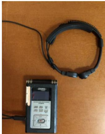
**Figure 3.10:** Contact Microphone
