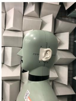
**Figure 3.18:** Pictures of HATS - lateral view in the anechoic chamber.
