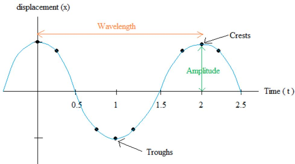
Figure 9 Description of a waveform
