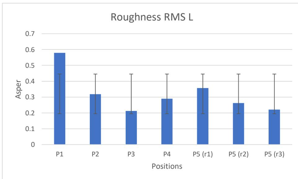
Figure 56: Roughness RMS left values - comparison between positions.
