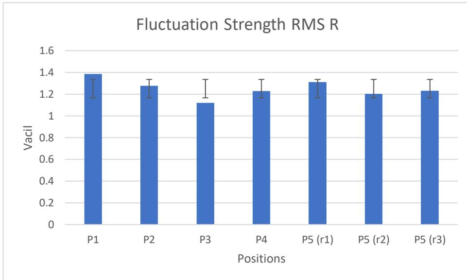
Figure 63: Fluctuation strength RMS right values - comparison between positions.
