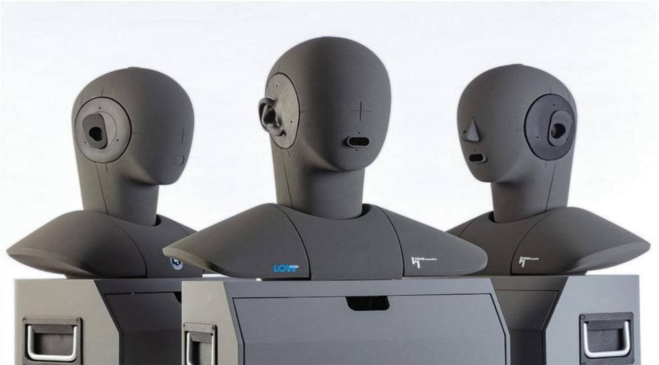
Figure 15 Dummy head for binaural recording.
