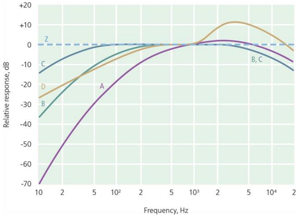
Figure 13 Weighting curves including Z-curve
