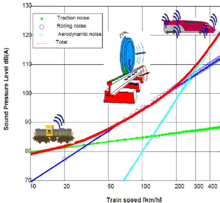
Figure 1: Relation between speed and noise source
