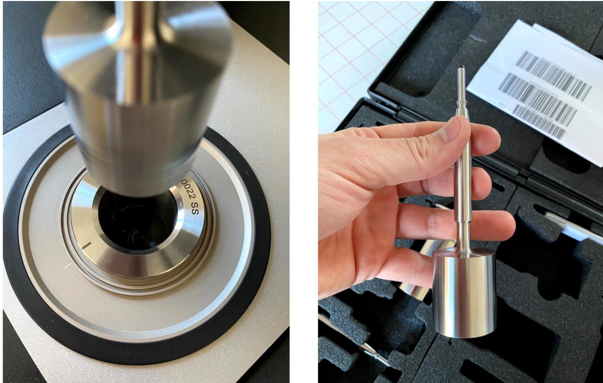
Figure 33. a) Content of the cement sample poured into the cylindrical test container. b) Peltier Cylinder Cartridge geometer
