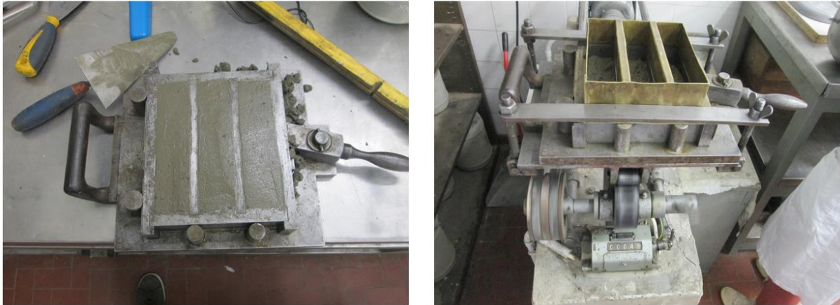
Figure 29. a) Mortar specimens. b) Mold and hopper firmly clamped to the jolting table.
