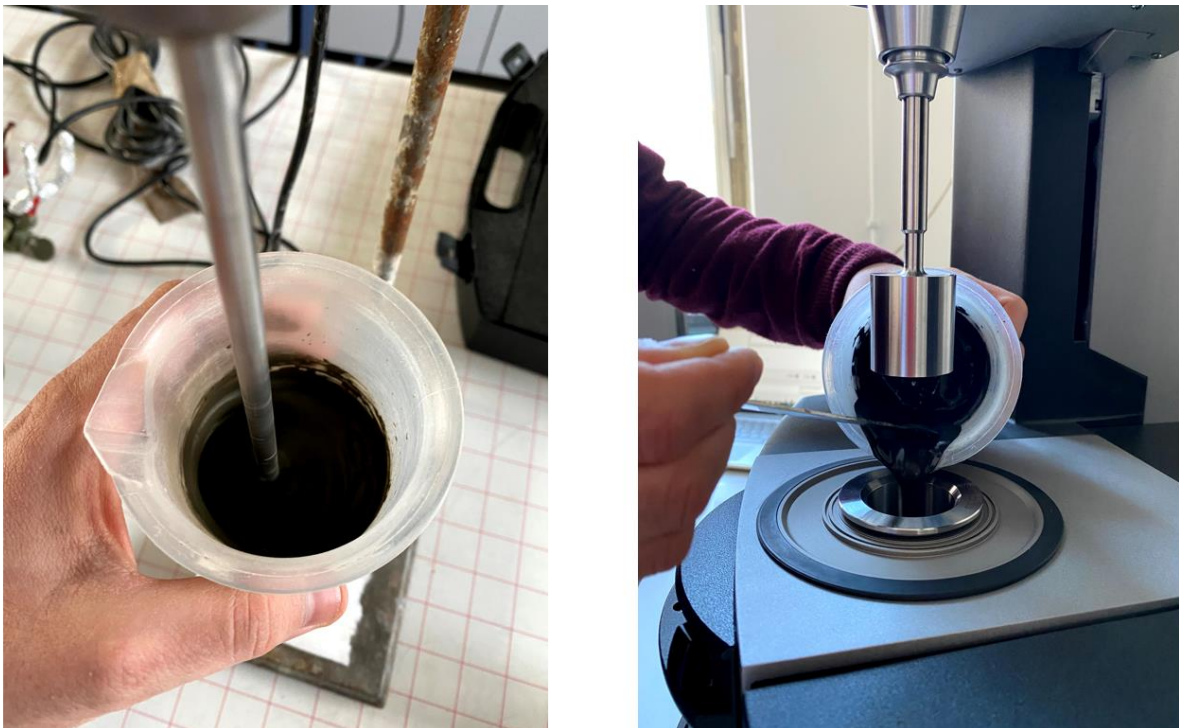
Figure 21. Specimen manufacturing for rheological test. b) Specimen poured in the cylindrical stain-less container.
