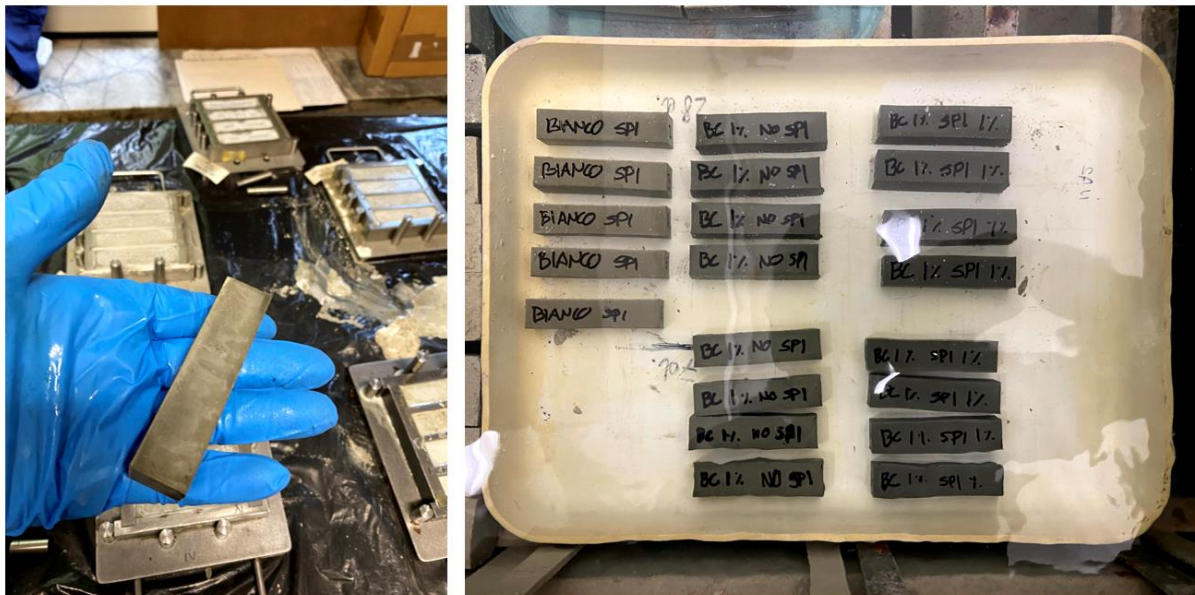
Figure 25. a) Demolding the samples. b) samples in the curing tank.
