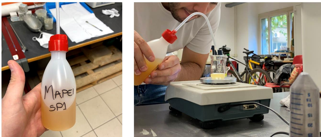
Figure 22. a) Superplasticizer Master Ease 7000 (ME7). b) Weighing the precise amount of the recipe.
