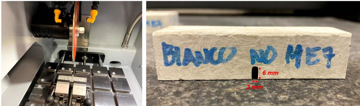
Figure 27. a) Shaft and cutting disc of the machine. B) U-notch sample cut.
