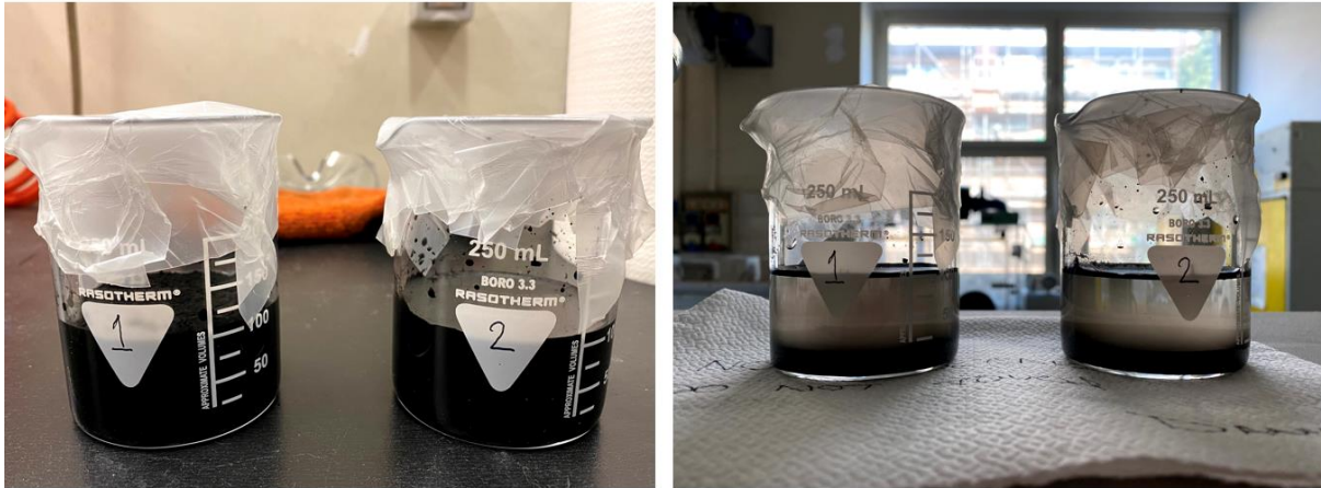
Figure 16. a) Specimen 1 & 2 sealed after adding water. b) Specimen 1 & 2 after 48h in wet conditions.
