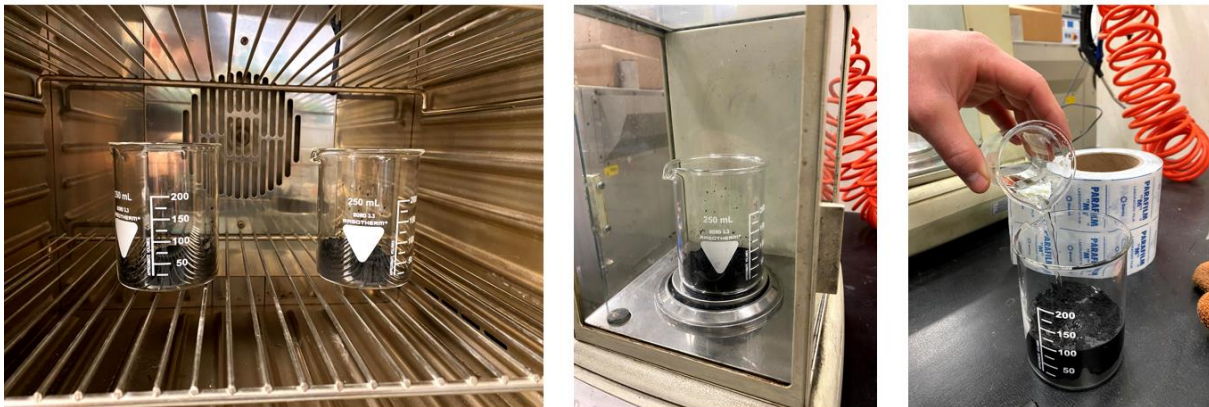
Figure 15. a) Specimen 1 right and 2 left on the oven. b) Dry Biochar. c) Adding 100g of water to specimen.
