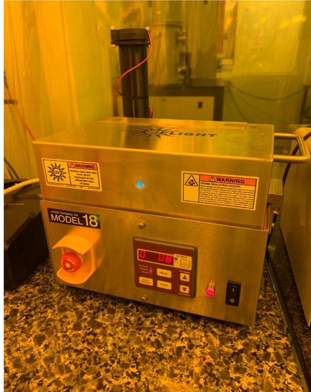
Figure 21: Jetlight UVO-Cleaner® model 18.
