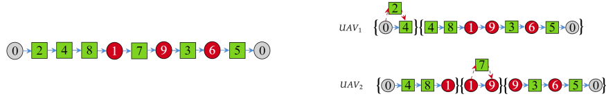
(A) The tsp tour input of the Local Search (B) After the 1 st iteration, the algorithm as- function adapted for two UAVs. Grey nodes represent the depot, green nodes represent drone eligible nodes and red nodes represent truck only nodes.
