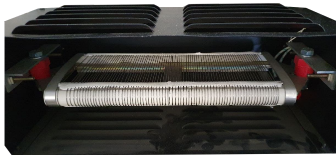
Figure 1.6: The braking resistor used, showing both the surrounding box and the inner thermal wire coil.
