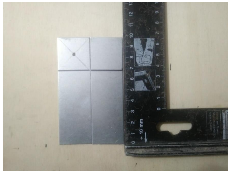
Figure 73 – Specimens of DP600 for degradation evaluation
