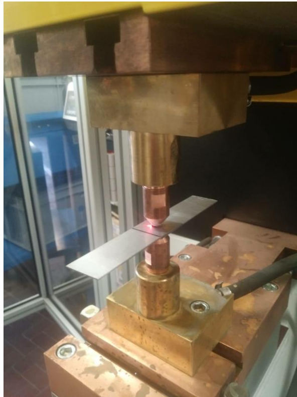
Figure 74 - Specimens under spot welding
