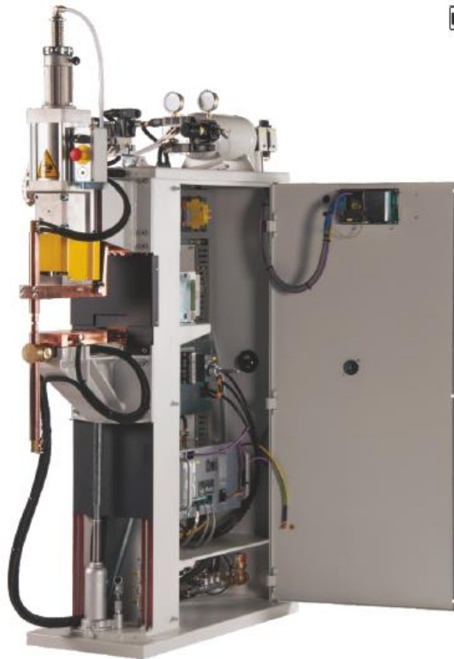
Figure 67 – Tecna Medium Frequency Welder item I122000001
