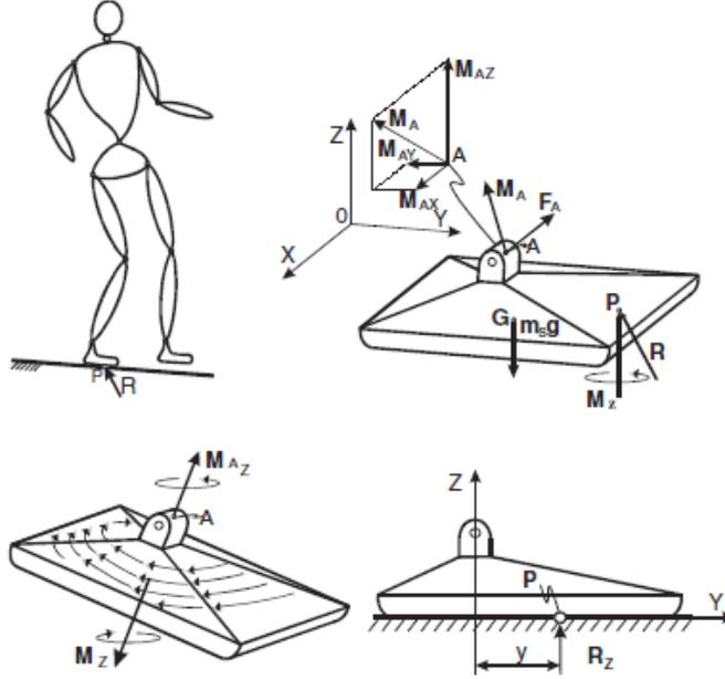
Figure 2.10: Biped body and forces acting on the support foot
