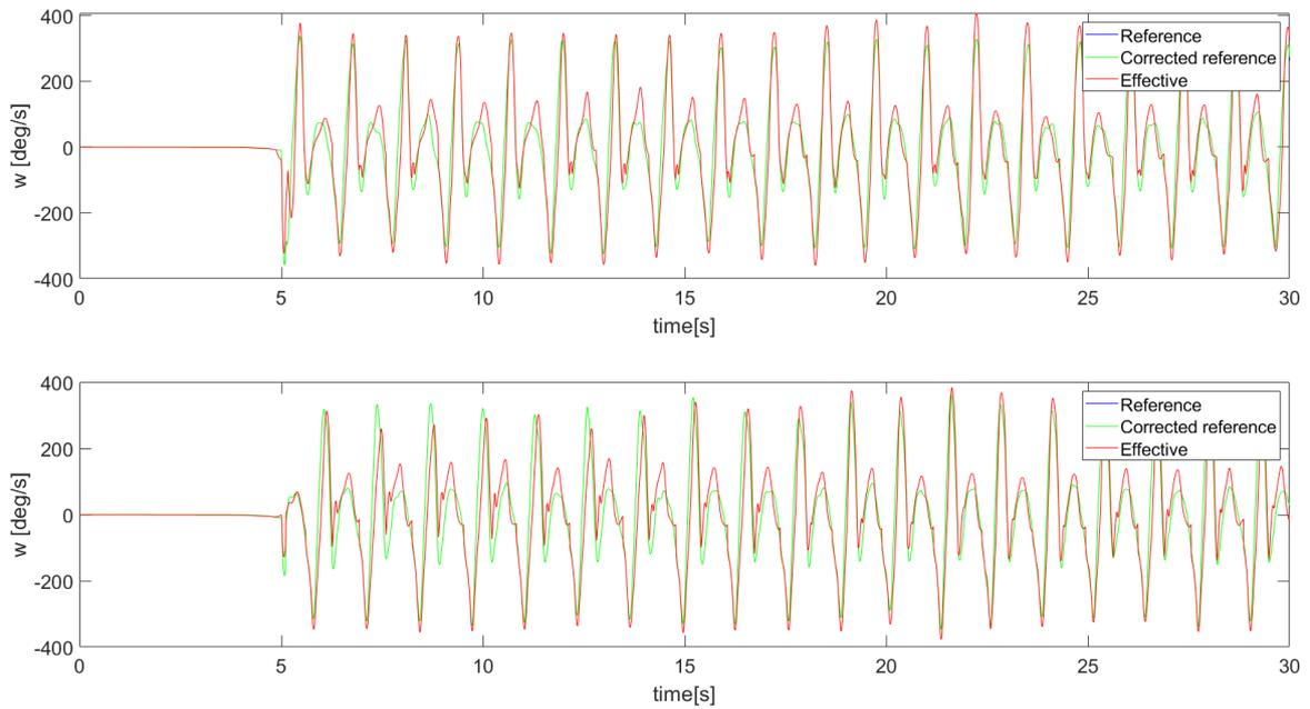
Figure 7.17: From top to bottom: left and right knee joints angular speed.
