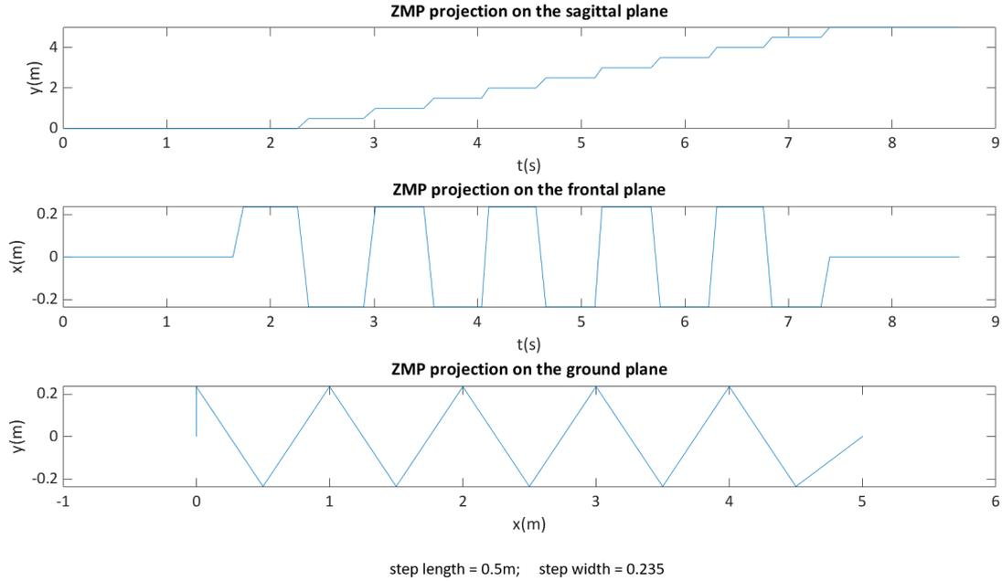
Figure 2.11: Projection of the ZMP for a constant step walk on the Sagittal, Frontal and ground planes
