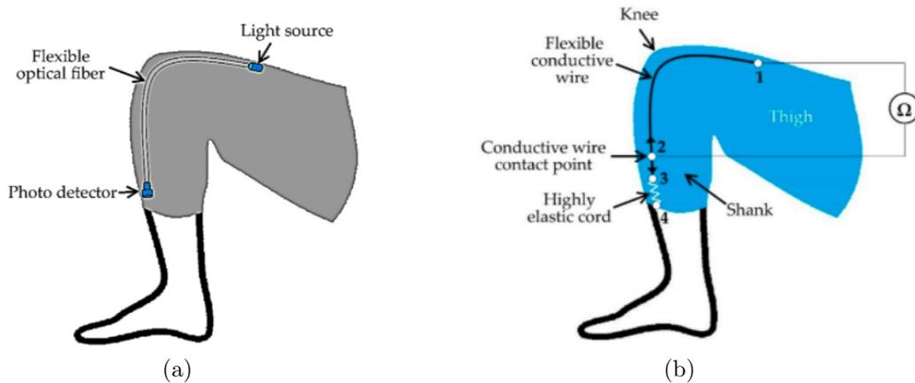
Figure 2.19: (a) Scheme of an optical fiber sensor. (b) Scheme of wearable wire sensor.
