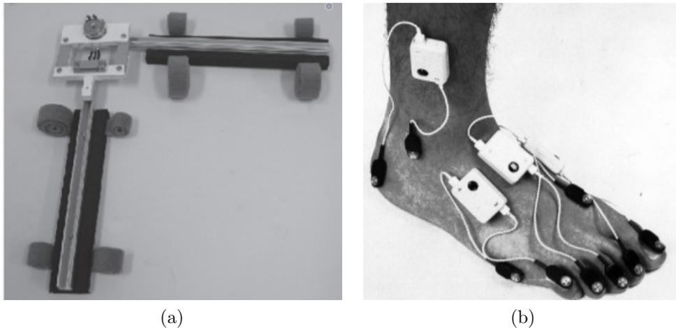
Figure 2.18: (a) A potentiometric electrogoniometer (b) Optoelectronic system positioned on a patient
