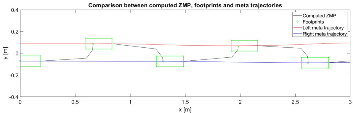
Figure 6.6: ZMP, feet trajectories and footprints in the ground plane (subject AB01 and trial s0x8i0).
