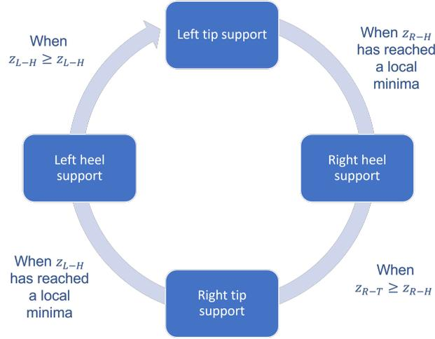
Figure 6.1: State machine representation for the subject AB01 and trial s0x8i0.
