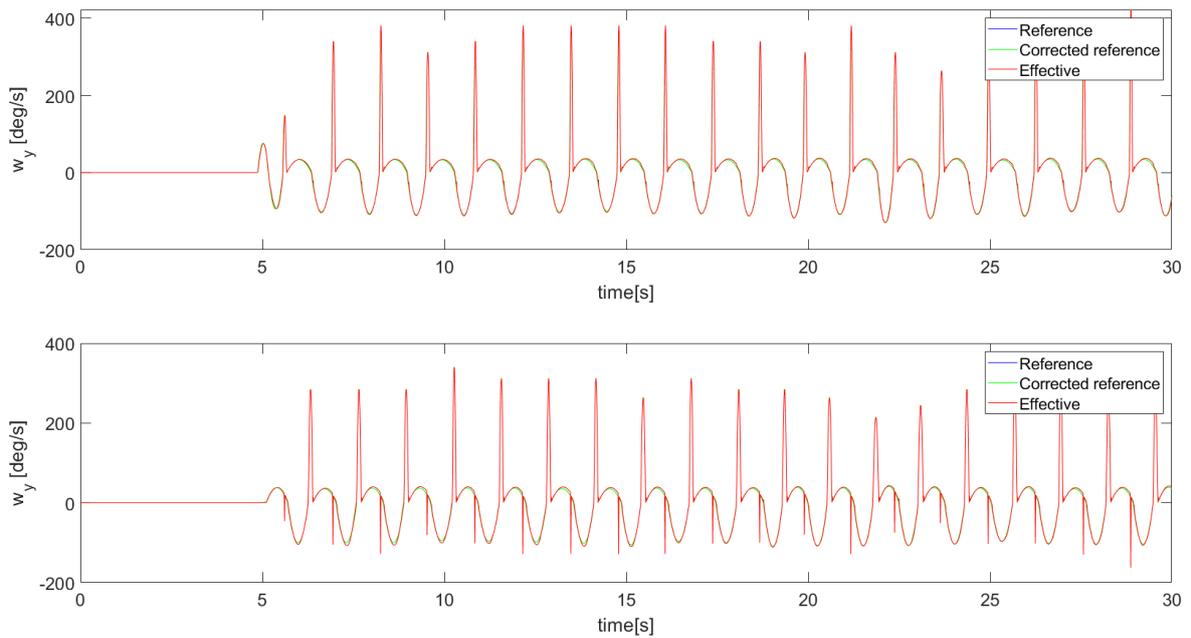
Figure 7.15: From top to bottom: left and right feet angular speeds around y-axis.
