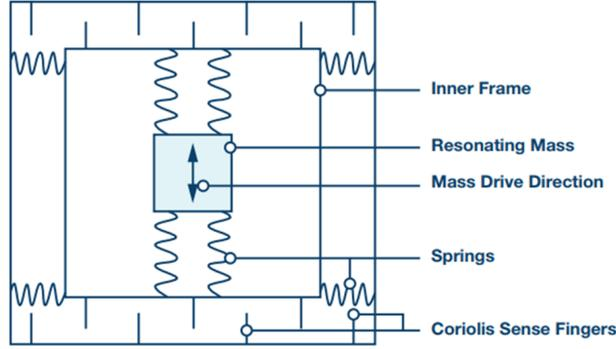
Figure 2.16: MEMS gyroscope scheme
