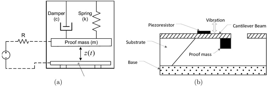
Figure 2.15: (a) Scheme of a capacitive accelerometer (b) Scheme of a piezoresistive accelerometer
