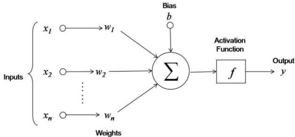
Figure 4.3: Working principle of a neurons
