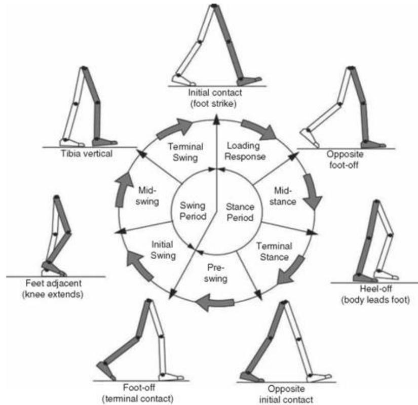
Figure 2.2: Relationship between the main phases and the sub-phases of the gait cycle
