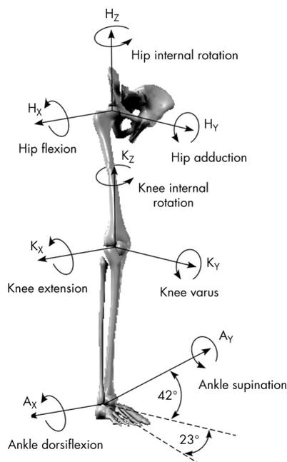
Figure 2.6: Local frames of the joints of a leg.
