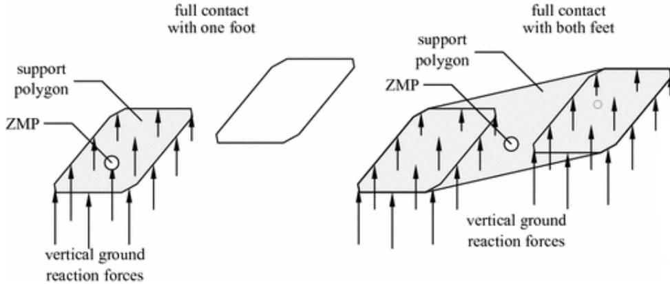
Figure 2.9: Biped body and forces acting on the support foot
