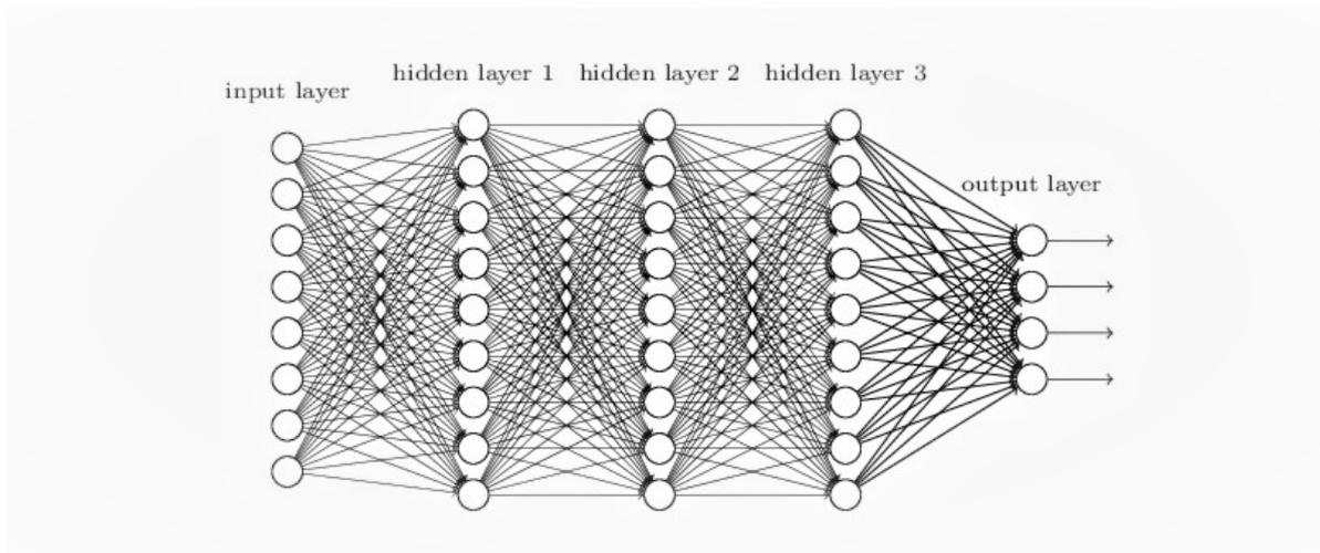
Figure 4.2: Input, output and hidden layers of a multilayer perceptron network
