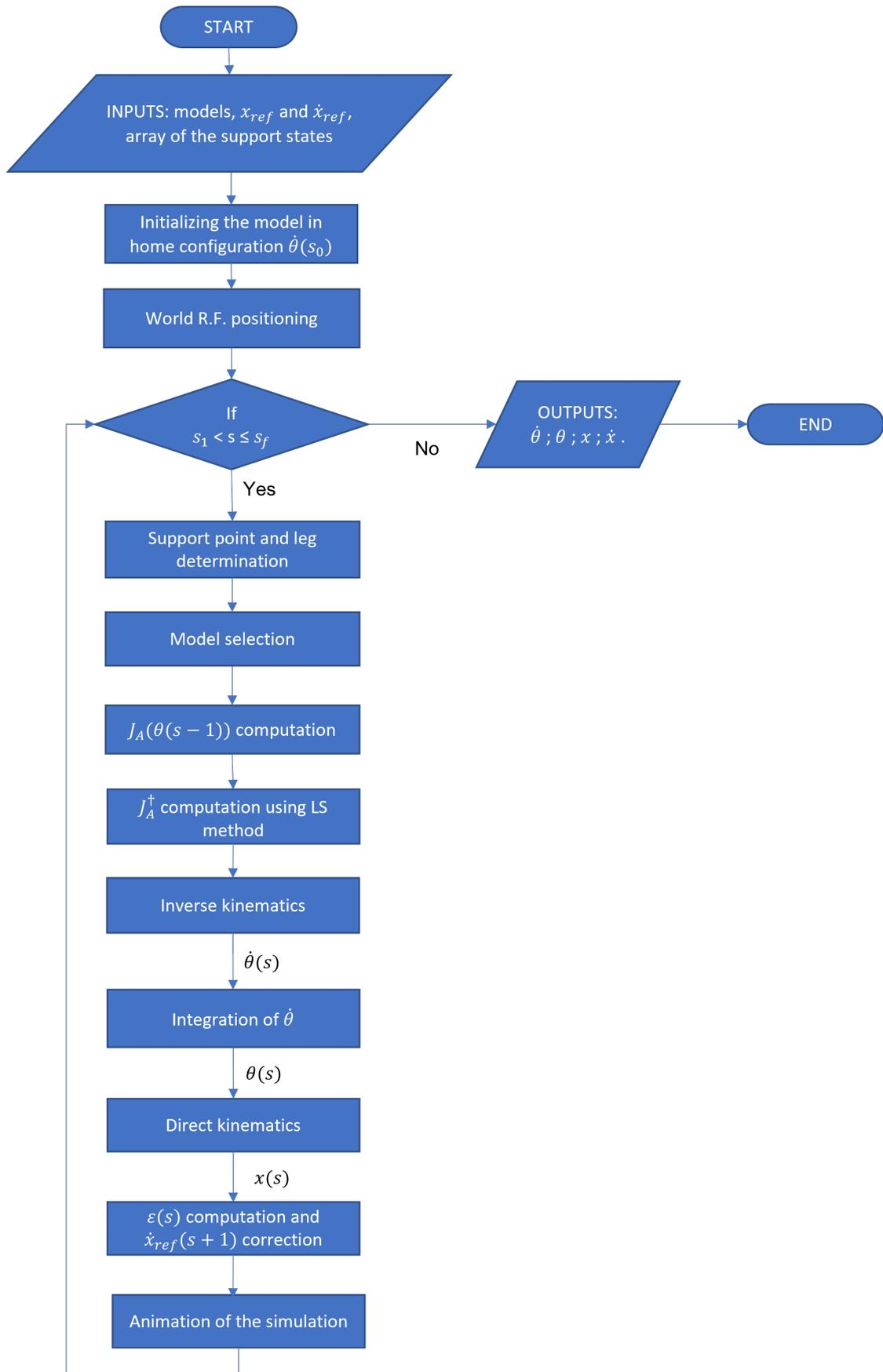
Figure 7.5: Flow diagram representation of the fitting process.
