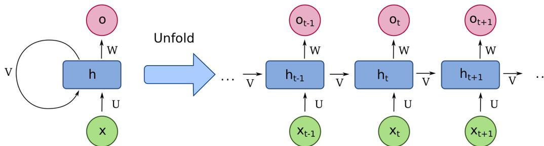
Figure 8.10: General structure of Recurrent neural networks
