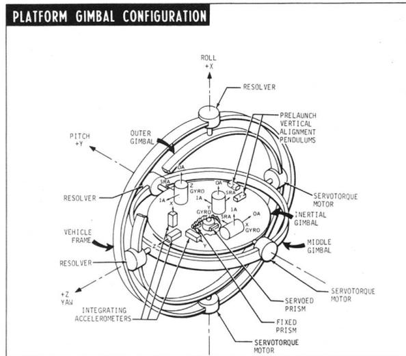
Figure 2.17: Inertial Measurement Units system
