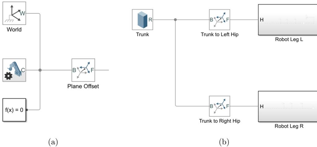
Figure 7.2: (a) World Frame, Solver and Mechanism blocks (b) Model organization into sub-systems.
