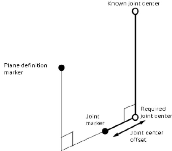
Figure 6.3: General geometric relationship between two successive joint centers and related markers
