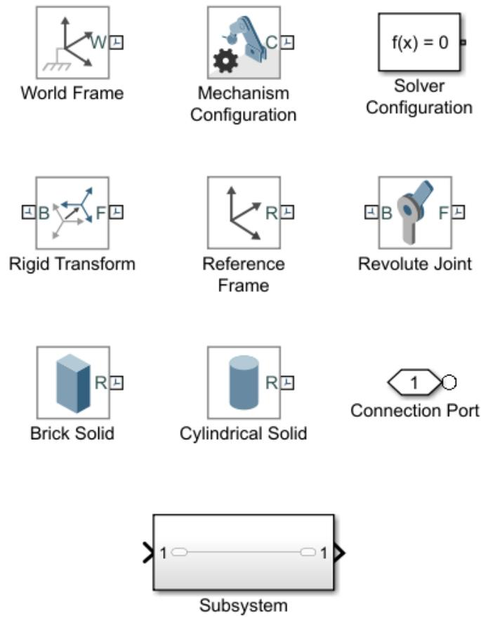
Figure 7.1: Simulink blocks used for the generation of the models
