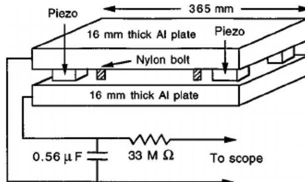
Figure 2.12: Scheme of a piezoelectrical force plate
