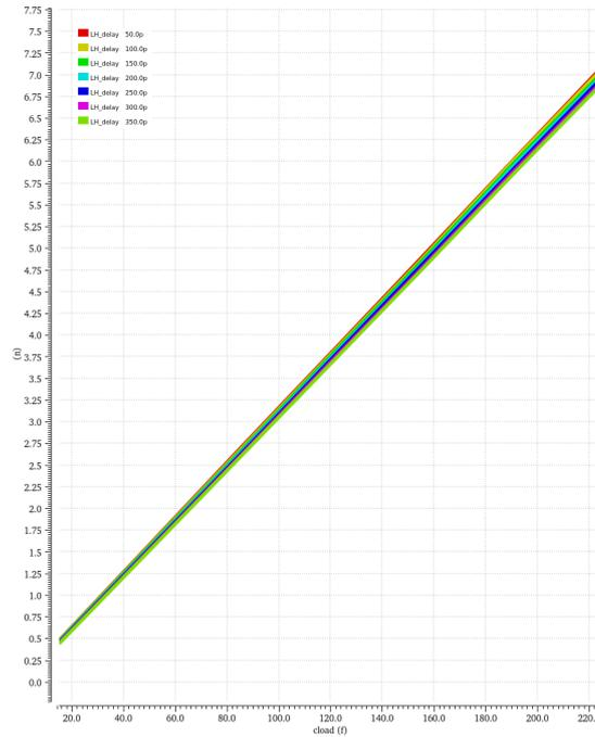
Figure 5.31: Low to high propagation delay (ns), state XOR, cell data ‘0’ and X switching from ‘0’ to ‘1’. LUT cell.
