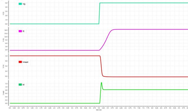
Figure 3.10: Reading waveforms of the FeFET model with  $R_{OUT} = 1 \text{ k}\Omega$  as pull-up resistor and  $C_{LOAD} = 100 \text{ fF}$  as load capacitance.
