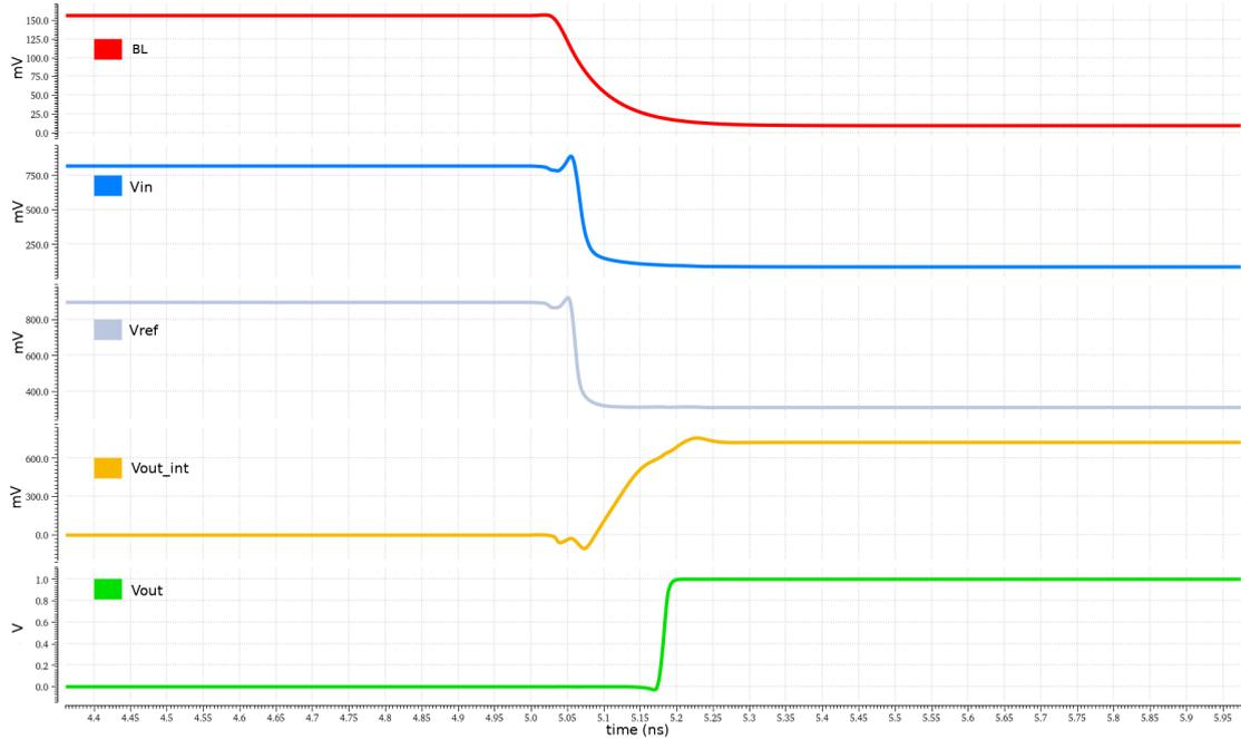
Figure 4.13: Signals in the cascode, differential pair and output stage during the simulation of a reading.
