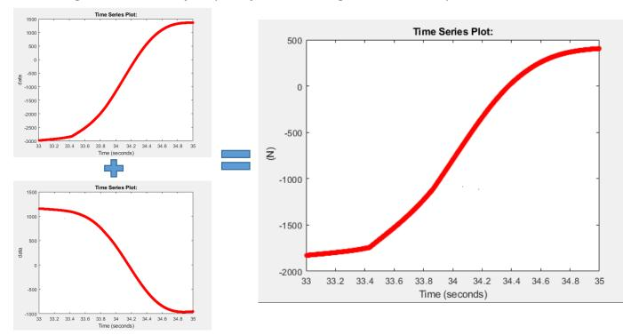
Figure 4.99: Summation of the lower back cylinder forces in fourth state and the final force required from this cylinder at this state (Forces in N).
