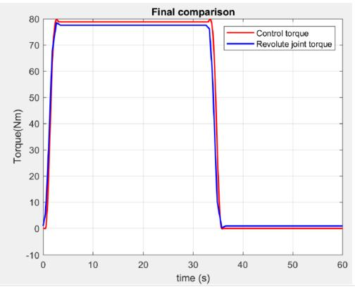
Figure 2.35: Comparison between control scheme torque and imported model torque.
