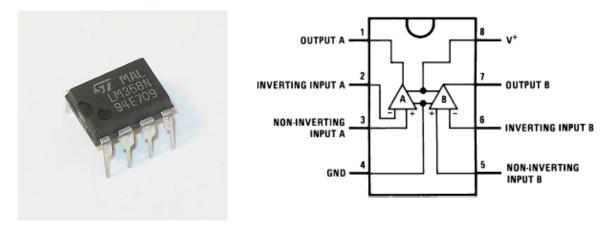
*Figure: 3.49: LM358-n operational amplifier and the pinout data.*
