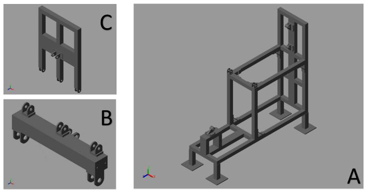
Figure: 4.79: Testbench parts, A is Base, B is Pelvic part, C is Backframe.
