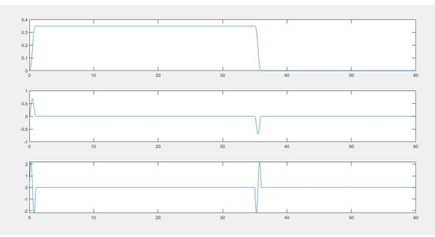
Figure 3.84: Kinematics of the hip joint. (x-axis is in s) (y-axis is in rad, rad/s and rad/s/s).
