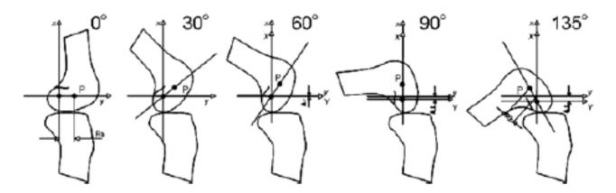
Figure 1.7: Compounded knee rotation and lift at various joint angles.
