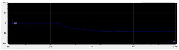
*Figure 3.63: Measurement of the angular position (blue) in clockwise rotation (x-axis is time in ms, and y-axis is angle in degrees).*
