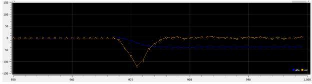
Figure 3.70: Measurement of the angular velocity (yellow) in clockwise rotation (x-axis is time in ms, and y-axis is angle rate in degrees) with delay filter.
