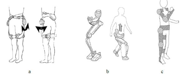
Figure 1.8B: Basic exoskeleton designs shown in ISO 13482 (a) Leg motion assistive device, (b) Body weight supportive device, (c) Exoskeleton wearable robot.
