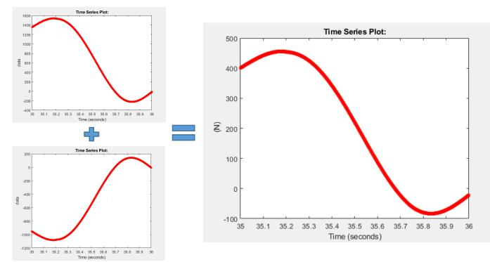
Figure 4.104: Summation of the lower back cylinder forces in fifth state and the final force required from this cylinder at this state (Forces in N).
