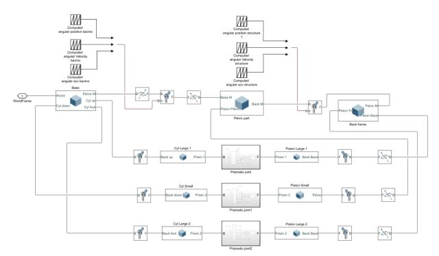
*Figure 4.86: The assembly model used to transfer the cycloidal law to the cylinders.*
