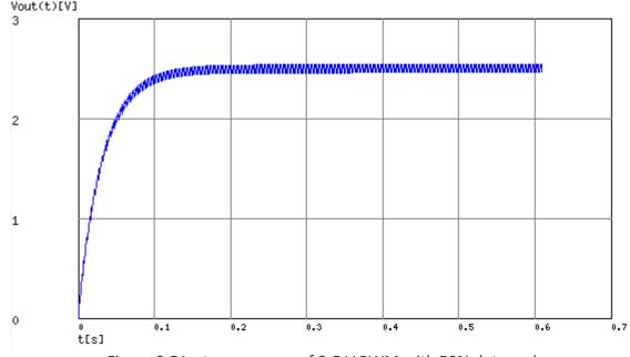
The step response of a 0-5 V PWM with 50% duty cycle is shown. (fig.3.51) Vout(t)[V]
