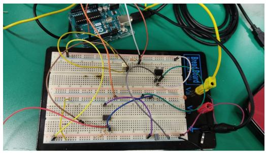
Figure 3.53: electronic circuit connected on bread board and Arduino integrated.
