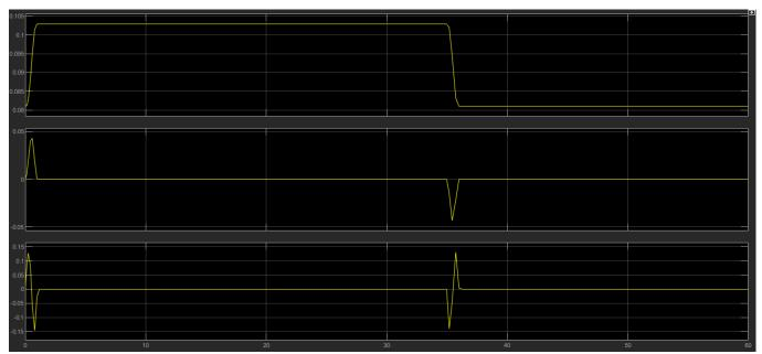
Figure 4.88: Kinematics of the small lower cylinder. (x- axis is in s) (y-axis is in m, m/s and m/s/s).
