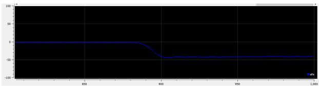
*Figure 3.75: Measurement of the angular position (blue) in clockwise rotation (x-axis is time in ms, and y-axis is angle in degrees) with weights filter.*
