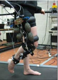
Figure 1.14: Pneumatically powered active (rigid) type exoskeleton.
