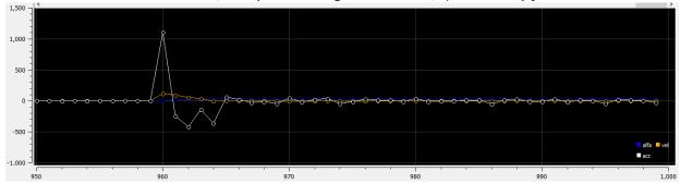
Figure 3.68: Measurement of the angular acceleration (white) in counterclockwise rotation (xaxis is time in ms, and y-axis is velocity rate in rad/s<sup>2</sup>) with delay filter.
