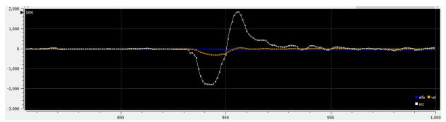
Figure 3.77: Measurement of the angular acceleration (white) in clockwise rotation (x-axis is time in ms, and y-axis is velocity rate in  $rad/s^2$ ) with weights filter.
