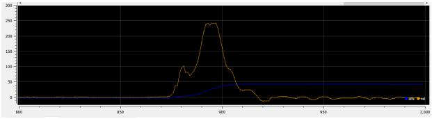
Figure 3.74: Measurement of the angular acceleration (white) in counterclockwise rotation (xaxis is time in ms, and y-axis is velocity rate in rad/s<sup>2</sup>) with weights filter.
