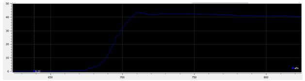
*Figure 3.60: Measurement of the angular position (blue) in counterclockwise rotation (x-axis is time in ms, and y-axis is angle in degrees).*
