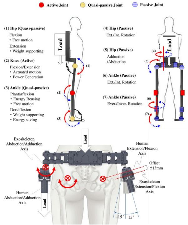
Figure 1.16: Mixed type exoskeleton between active and passive.
