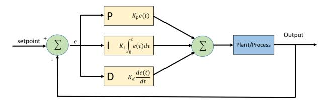
Figure 2.26: Schematic of a PID controller.
