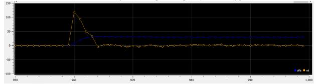
Figure 3.67: Measurement of the angular velocity (yellow) in counterclockwise rotation (x-axis is time in ms, and y-axis is angle rate in rad/s) with delay filter.
