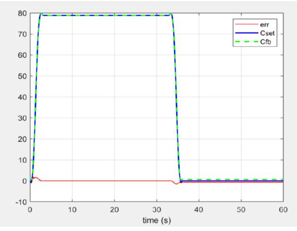
*Figure 2.24: Comparison between* C<sub>SET</sub> *and* C<sub>FB</sub>*, and the error developed.*
