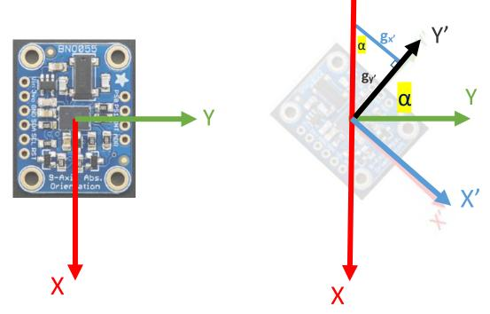
Figure 3.59: Counterclockwise graphical orientation of the sensor.
