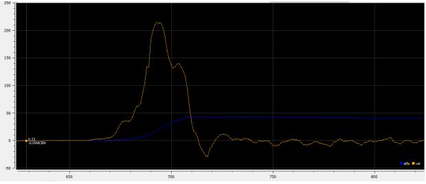
*Figure 3.61: Measurement of the angular velocity (yellow) in counterclockwise rotation (x-axis is time in ms, and y-axis is angle rate in rad/s).*
