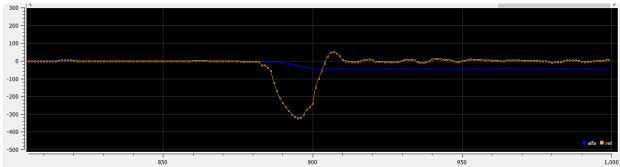
Figure 3.76: Measurement of the angular velocity (yellow) in clockwise rotation (x-axis is time in ms, and y-axis is angle rate in degrees) with weights filter.
