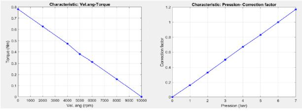
*Figure 2.22: (a) Trend of the angular torque-speed characteristic. (b) Trend of the correction factor for torque.*
