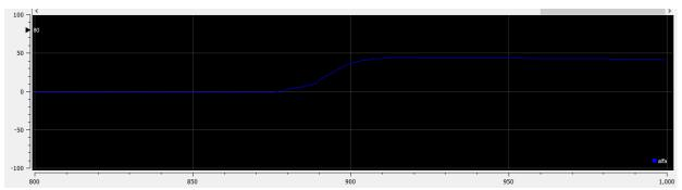
*Figure 3.72: Measurement of the angular position (blue) in counterclockwise rotation (x-axis is time in ms, and y-axis is angle in degrees) with weights filter.*
