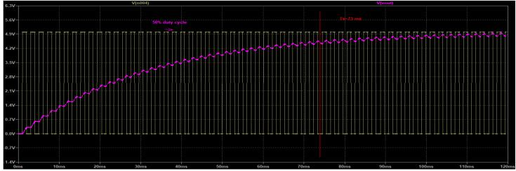
*Figure: 3.52: comparing the PWM signal from Arduino with 50% duty cycle with the output from the designed electronic board.*
