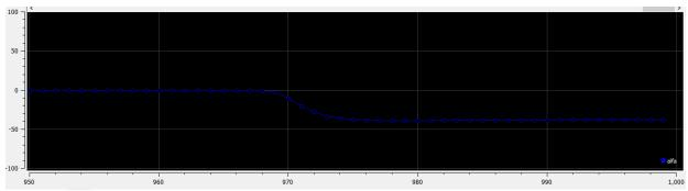
Figure 3.69: Measurement of the angular position (blue) in clockwise rotation (x-axis is time in ms, and y-axis is angle in degrees) with delay filter.
