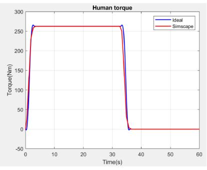
*Figure: 2.37: Comparison between the torque generated by the formula and the one produced by the Simscape model.*
