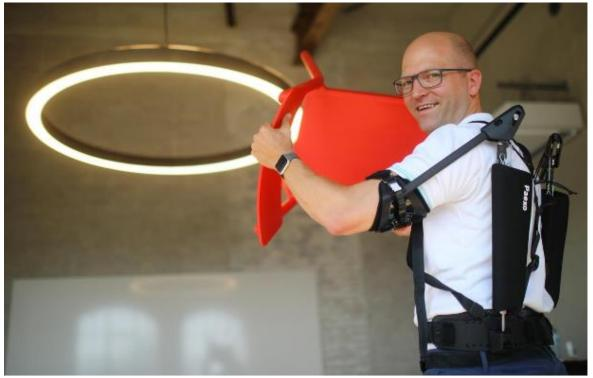
Figure 1.11: Ottobock Paexo Upper extremity exoskeleton.
