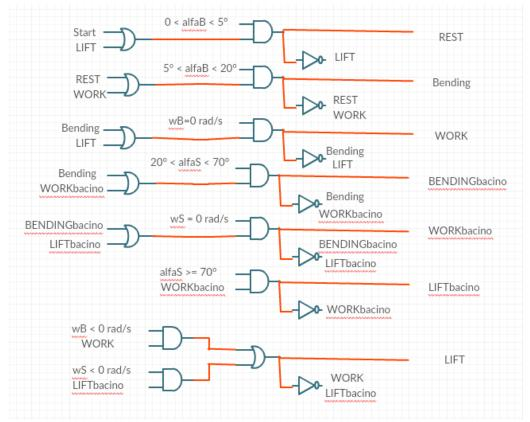
Figure 3.58: logical control representing the sates of operation.
