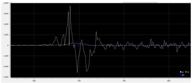
Figure 3.62: Measurement of the angular acceleration (white) in counterclockwise rotation (xaxis is time in ms, and y-axis is velocity rate in rad/s<sup>2</sup>).
