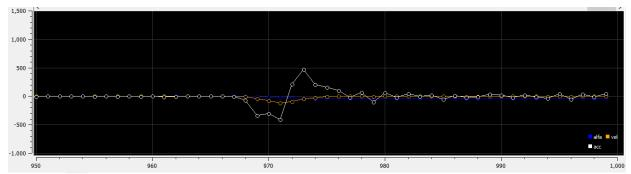
Figure 3.71: Measurement of the angular acceleration (white) in clockwise rotation (x-axis is time in ms, and y-axis is velocity rate in rad/s<sup>2</sup>) with delay filter.
