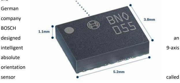
BNO055 (fig.3.44) which has integrated 3 different sensors: 3-axis accelerometer, 3-axis gyroscope, 3-axis magnetometer. The sensor has intelligent data fusion algorithms that uses all data inputs and feed as output quaternions, linear acceleration, rotation, gravity and robust heading. It is used in several applications as: automotive to feed the orientation and acceleration of a vehicle, robotics applications and even gaming joysticks to define heading of the controller in the gamer hands.
