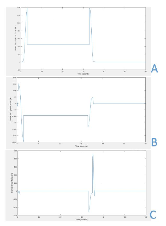
Figure 4.106: A) Upper back cylinder force. B) Lower back cylinder force. C) Front cylinder force.
