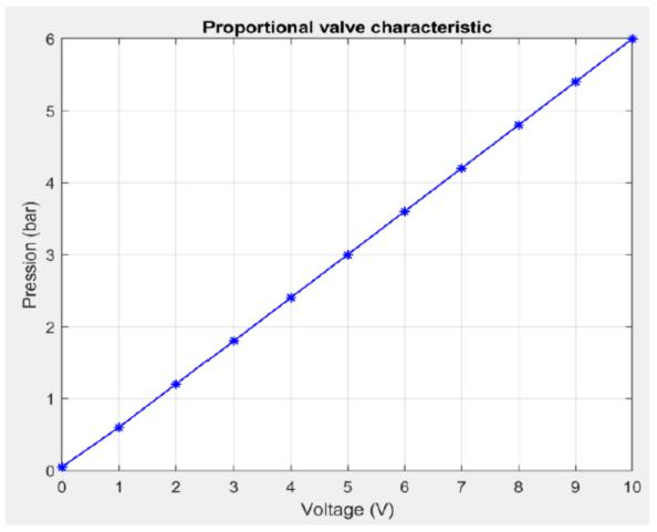
*Figure 2.21: Voltage Pressure characteristics of the proportional valve.*
