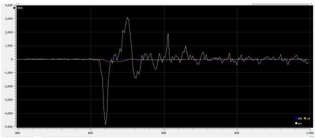
Figure 3.65: Measurement of the angular acceleration (white) in clockwise rotation (x-axis is time in ms, and y-axis is velocity rate in rad/s<sup>2</sup>).
