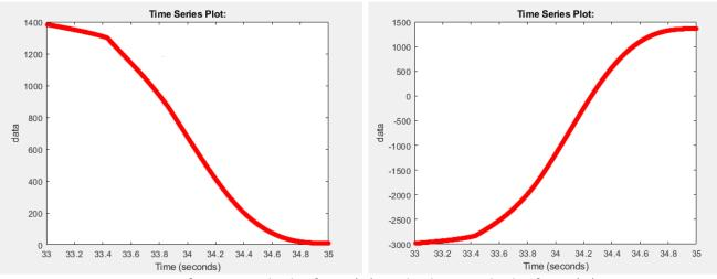
Figure 4.97: Left: upper cylinder force (N), Right: lower cylinder force (N).
