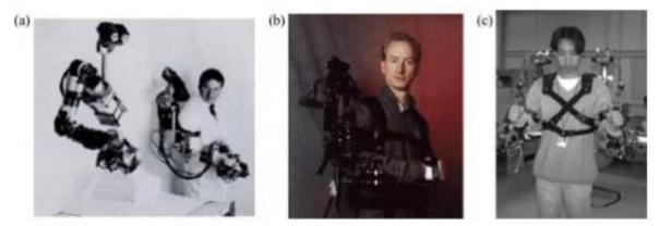
Figure 1.5: Exoskeleton-type master arm: (a) exoskeleton master of GE; (b) exoskeleton arm of Stanford [13]; (c) KIST exoskeleton arm with electric brakes
