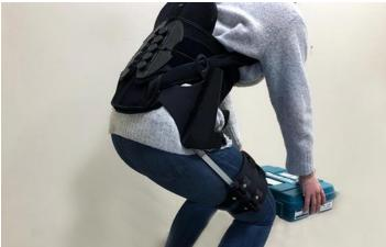
Figure 1.15: Passive type exoskeleton.
