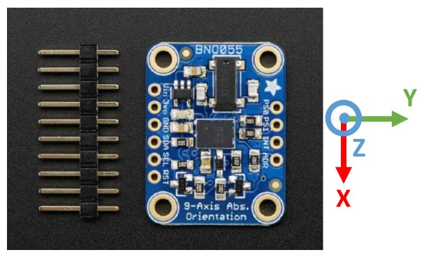
Figure 3.45: Adafruit BNO055 absolute orientation sensor (Appendix J).
