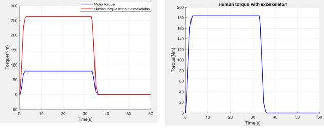
*Figure 2.38: Torque produced by the air motor and the human with and without the exoskeleton.*
