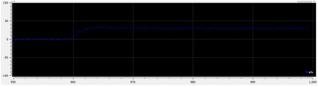
Figure 3.66: Measurement of the angular position (blue) in counterclockwise rotation (x-axis is time in ms, and y-axis is angle in degrees) with delay filter.
