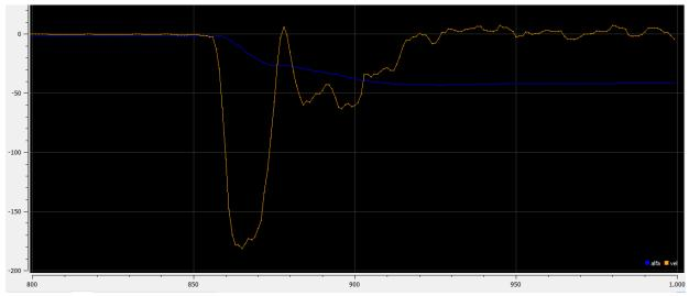
*Figure 3.64: Measurement of the angular velocity (yellow) in clockwise rotation (x-axis is time in ms, and y-axis is angle rate in degrees).*
