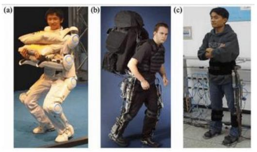
Figure 1.6: Walking assistive exoskeleton: (a) HAL-5 system [16]; (b) BLEEX lower limb exoskeleton [17]; (c) exoskeleton leg for human's walking power augmentation of Zhejiang University
