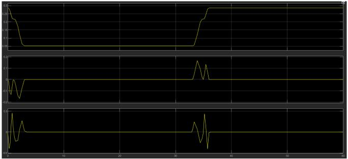
Figure 4.89: Kinematics of the large frontal cylinder. (x- axis is in s) (y-axis is in m, m/s and m/s/s).
