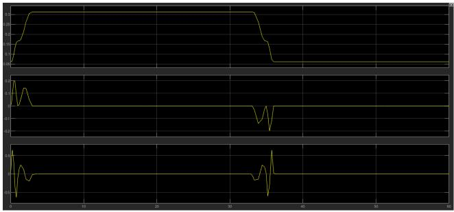
Figure 4.87: Kinematics of the large upper cylinder. (x- axis is in s) (y-axis is in m, m/s and m/s/s).
