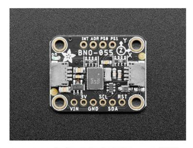
The new version of the board includes SparkFun qwiic (https://adafru.it/Fpw) compatible STEMMA QT (https://adafru.it/Ft4) connectors for the I2C bus so you don't even need to solder! Use a a plug-and-play STEMMA QT cable to get 9 DoF data ASAP.
