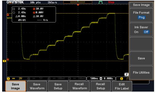
*Figure 3.54: stepping duty cycle output from electronic board.*
