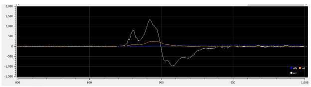
Figure 3.73: Measurement of the angular velocity (yellow) in counterclockwise rotation (x-axis is time in ms, and y-axis is angle rate in rad/s) with weights filter.
