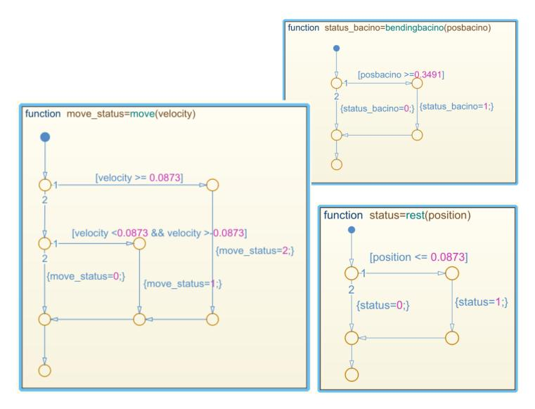
Figure 3.57: Functions used to define conditions to translate between phases.
