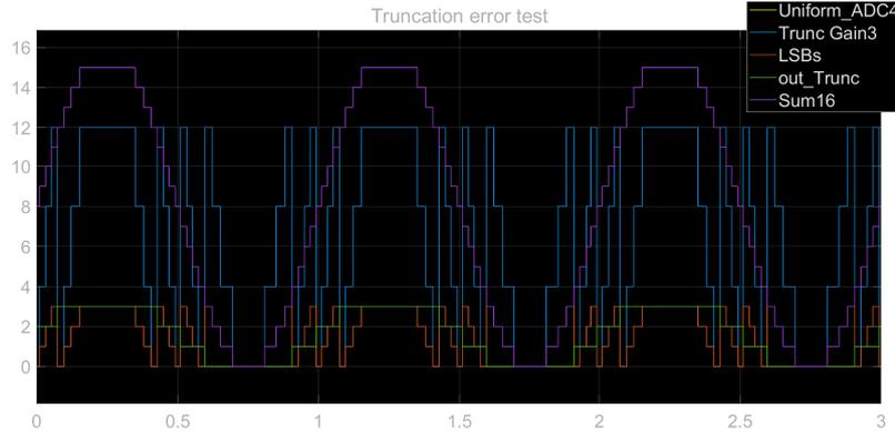
Figure 3.44: Timing diagram of truncation and LSBs recovering
