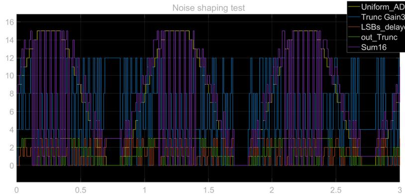
Figure 3.46: Noise shaping test results ( $nbit_{ADC} = 4$ ,  $LSBs = 2$ ,  $MSBs = nbit_{PWM} = 2$ )
