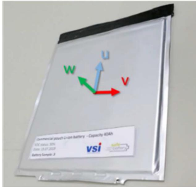
Figure 4.1: Reference system used for the orientation of the orthotropic thermal conductivity measurements. The “w” vector is on the battery thickness direction, “v” vector is parallel to the tabs direction, and “u” vector is perpendicular to them [15]
