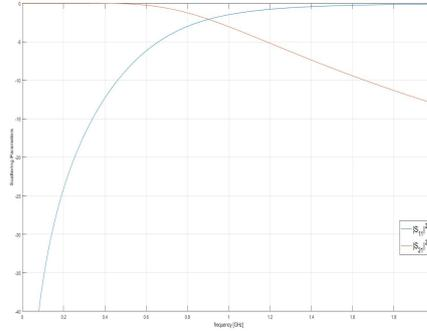
**Figure 3.5:** Low Pass Filter Degree 2 &  $f_c=800$  MHz with lumped elements
