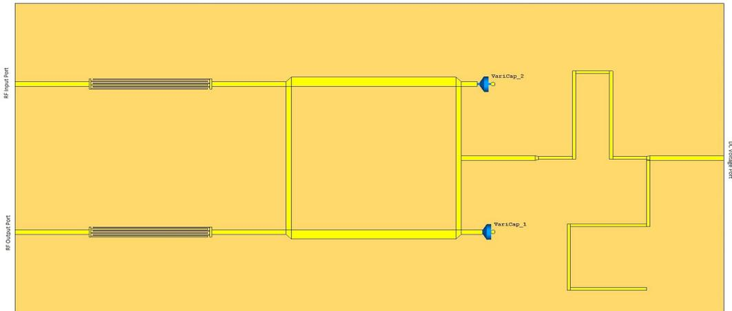
**Figure 3.11:** Analog Phase Shifter with Varactor Diodes
