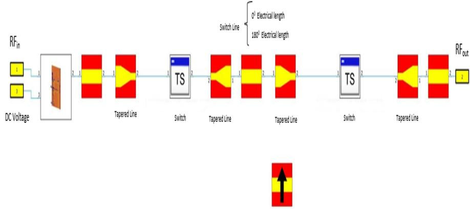
**Figure 3.17:** Schematic of the Analog Phase Shifter with MACOM switch
