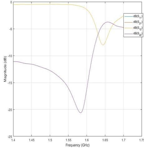
**Figure 3.4:**  $|S_{11}(j\omega)|$  &  $|S_{21}(j\omega)|$  of the IDC
