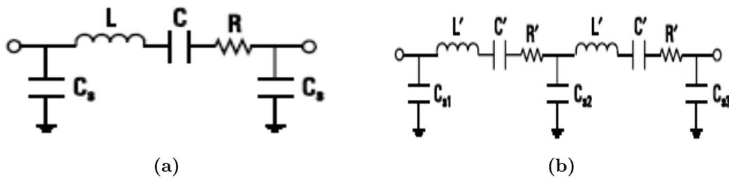
**Figure 2.5:** Equivalent Lumped Element model of IDC, (a) Low frequency (b) High frequency
