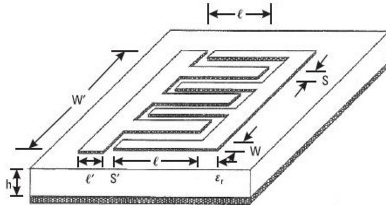
**Figure 2.4:** Interdigital Capacitor schematic
