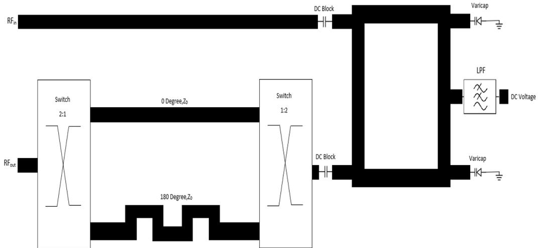
**Figure 2.2:** Schematic of the Analog Phase Shifter with MACOM switches
