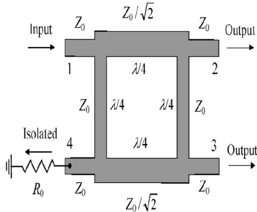
Figure 2.3: Branch Line Quadrature Hybrid with Microstrip
