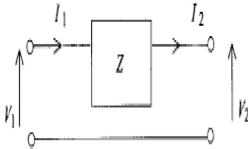
**Figure 2.8:** Series Circuit Element
