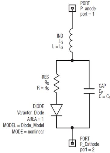
**Figure 3.8:** Spice model of varactor diode
