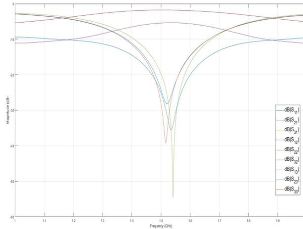
**Figure 3.2:** Scattering Parameters of the Quadrature Hybrid
