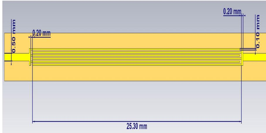
**Figure 3.3:** Interdigital Capacitor
