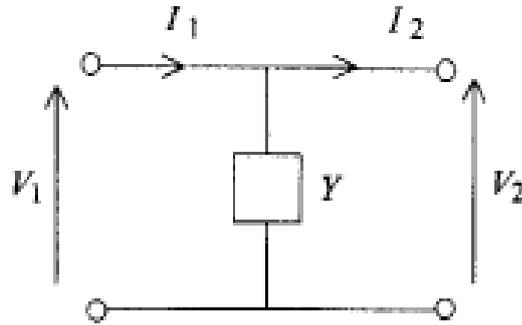
**Figure 2.9:** Shunt Circuit Element
