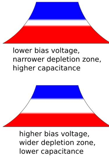
**Figure 2.12:** Affect of voltage on Depletion layer
