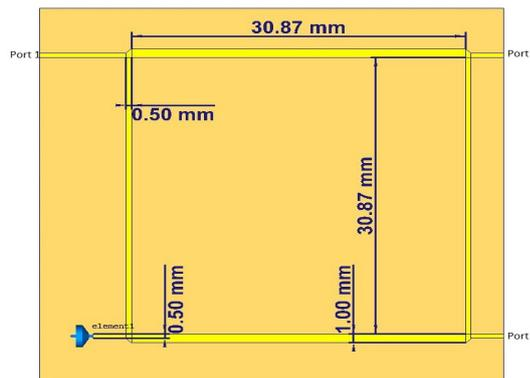
**Figure 3.1:** Designed Branch Line Quadrature Hybrid
