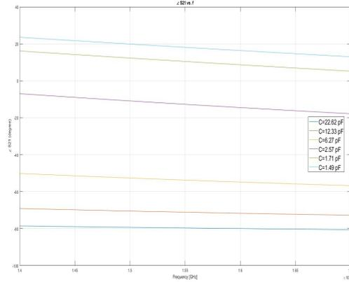
**Figure 3.10:** Variation of the output signal phase by changing the varactor diode’s voltage
