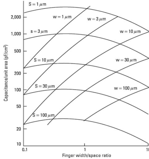
**Figure 2.6:** Design Curve
