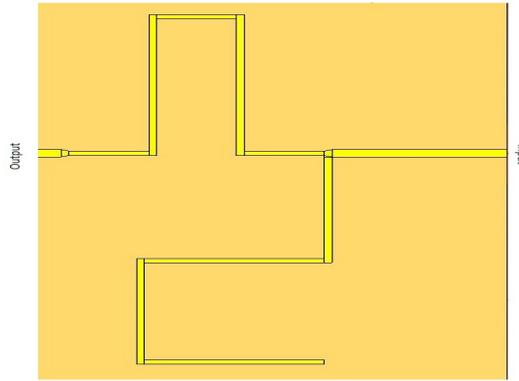
**Figure 3.6:** Low Pass Filter Degree 2 &  $f_c=800$  MHz
