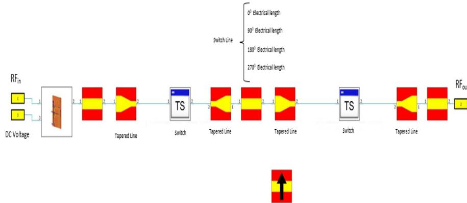
Figure 3.14: Schematic of the Analog Phase Shifter with JRC switch
