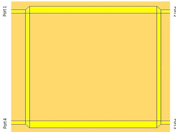
**Figure 1.1:** Quadrature Hybrid-Branch Microstrip Line
