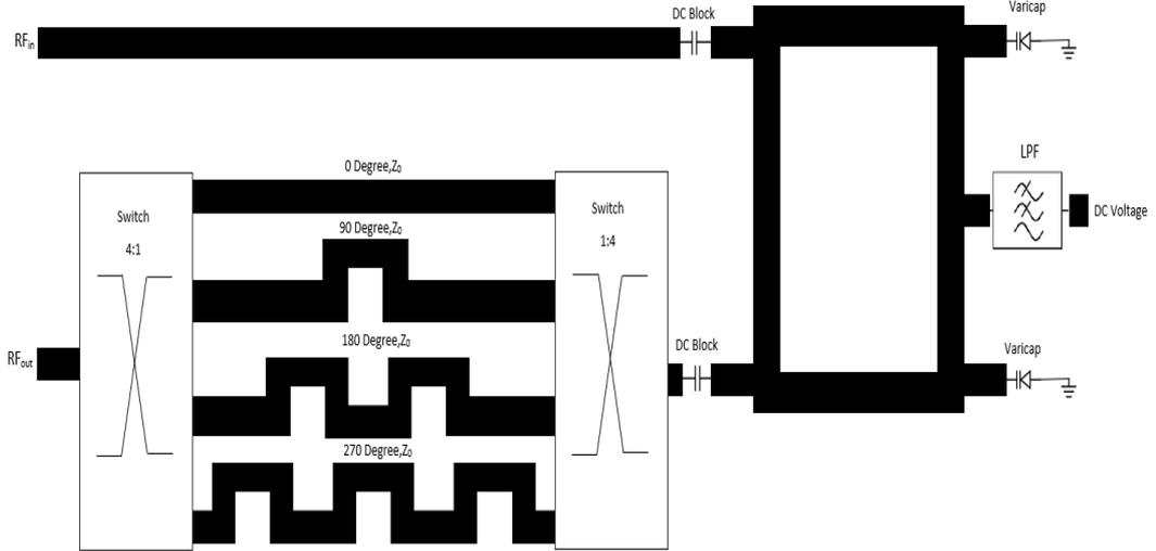
**Figure 2.1:** Schematic of the Analog Phase Shifter with JRC switches
