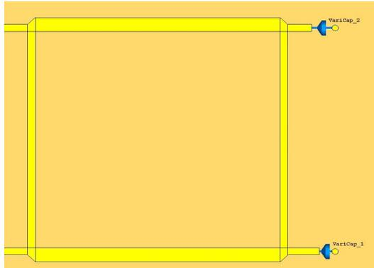
**Figure 3.9:** Quadrature branch line with varactor diodes
