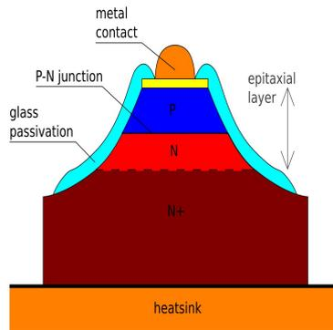
**Figure 2.11:** Internal Structure of Varactor Diode
