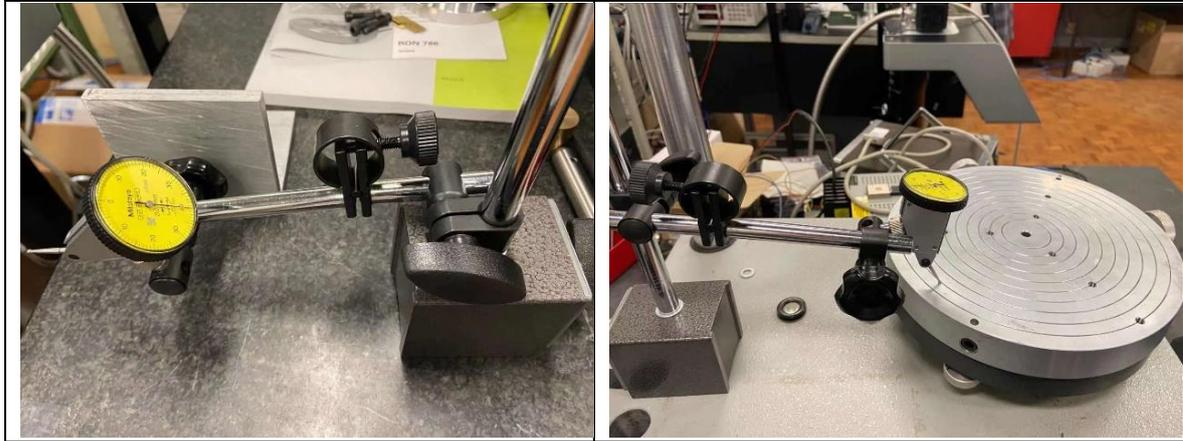
*Figure 4.1.4-1 roundness platform horizon calibration*
