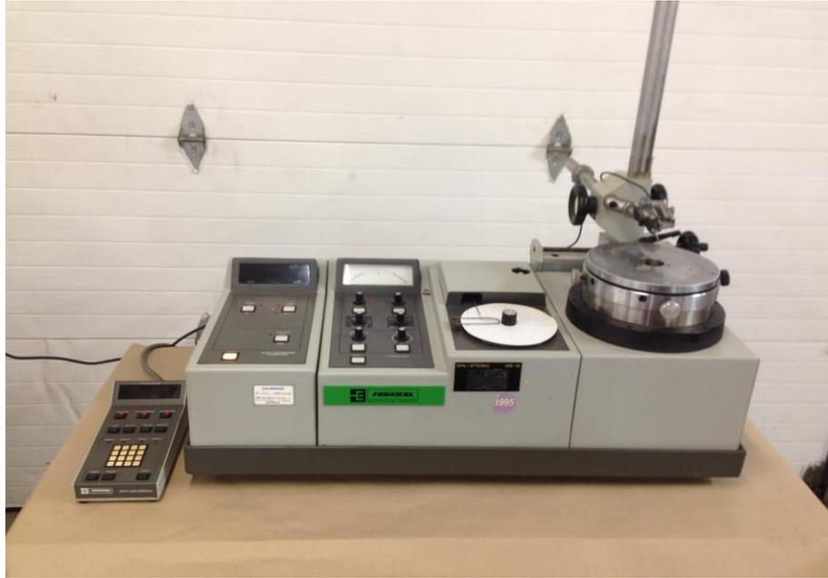
*Figure 2.3.1-1 the whole equipment of the roundness checker*
