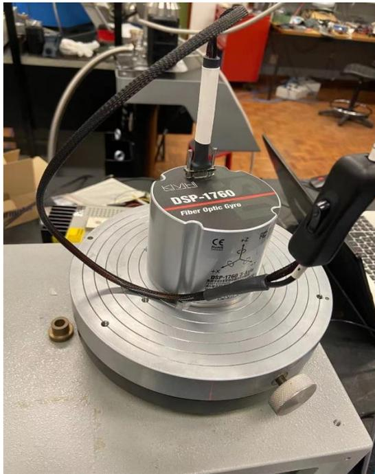
Figure 5.1.1-1 FOG test on Z-axis
