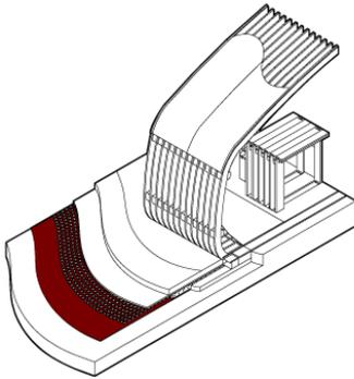
The general requisite for the mentioned layers is the resistance against water and root action. Both layers can be integrated as one single element and being also compatible, resist the permanent loads of the upper layers and resist the presence of microorganisms. The Zinco's company proposes to implement two stratum; the Protection Mat SSM 45 [appendix 2] and the Antirroot WSF40 [appendix 1]. However, other companies propose a single sheet with both functions
