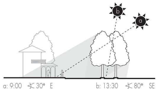
Scheme sections of a typical street of Turin, illustrating examples of sun inclination during the solstices in the morning and mid-day. Elaborated by the author.
