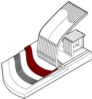
The referential Zinco<sup>®</sup> substrate consists in an allegedly ecological mix, since it is produced from recycled materials. Essentially, composed by treated bricks based on minerals and fiber matter compost. The brand offered mix depth of "Zincoterra" varies from 80mm to 90mm.
