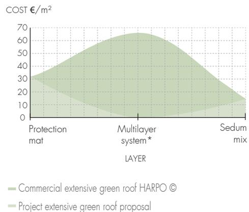
[\*] The multilayer system of the commercial version includes growing media, filter mat, drainage layer, mechanical protection sheet. Its equivalent, in the propose includes: Growing media, filter and drainage. Elaborated by the author using as reference cost reports provided by Harpo
