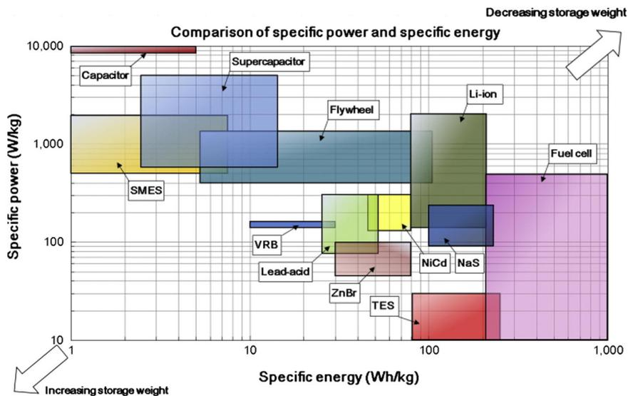
Figure 1.2 A Ragone plot for energy storage devices comparison. [5]
