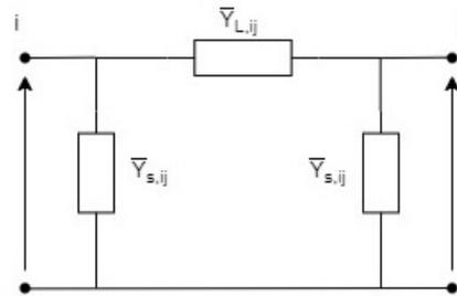
Figure 3.2  $\pi$ -equivalent circuit for a generic branch.
