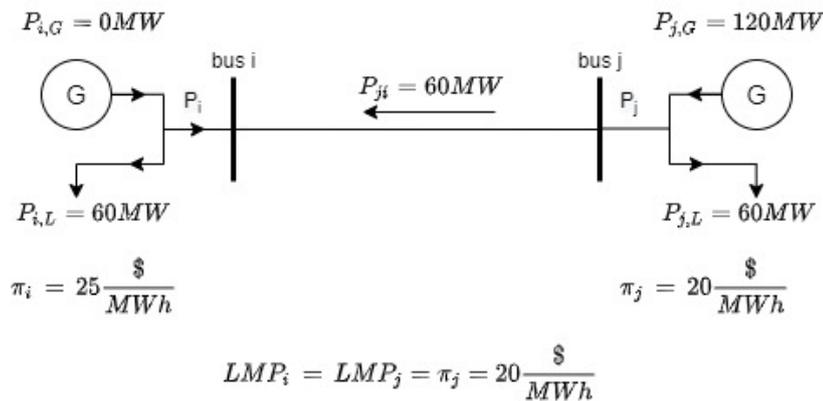
Figure 3.7 Two bus non-congested system example.
