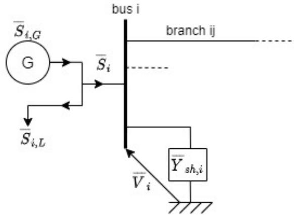
Figure 3.1 A generic representation of a bus  $i$ , with multiple connection to the grid.
