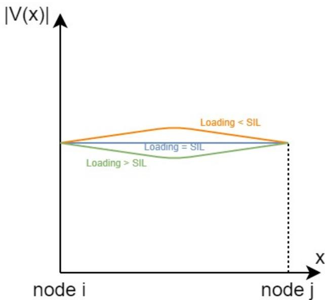
Figure 3.3 Approximated voltage profiles in a transmission line with respect to the SIL.
