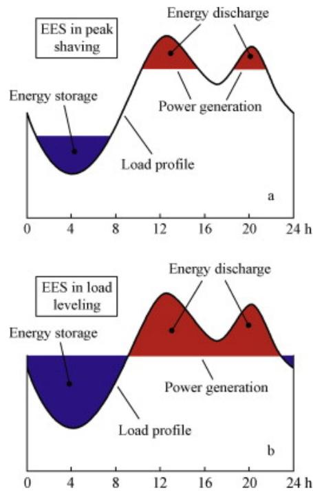
Figure 4.4 Electrical Energy Storage (ESS) role for Peak shaving (a) and Load Levelling (b) [64].
