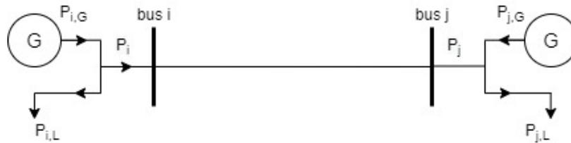
Figure 3.6 Two bus system example.
