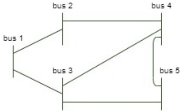
Figure 7.1 5 bus system, single line diagram.
