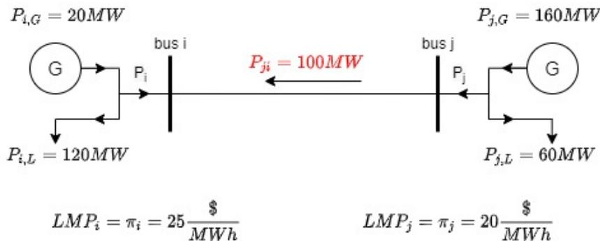
Figure 3.8 LMP in case of congestion in a two bus system
