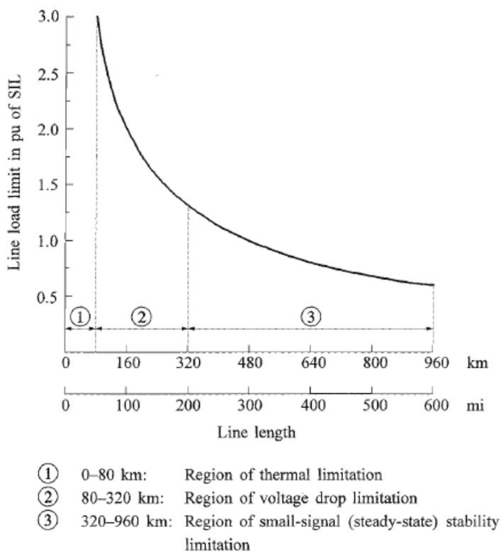
Figure 3.4 Loadability curve for a transmission line [17].
