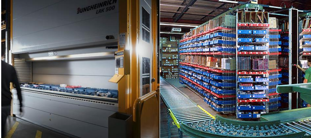
Figure 2.20. Paternoster and carouse racks (source: Jungheinrich AG, Cisco Eagle Ltd)
