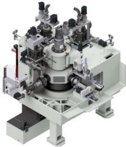
Figure 1.8. Transfer machine for manufacturing of machined components (source: Sistech Srl)
