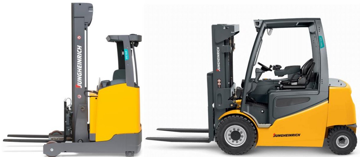
Figure 3.6. Reach truck and counterbalanced forklift truck (source: Jungheinrich AG)
