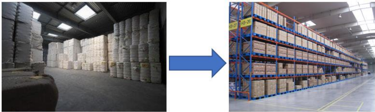
Figure 4.4. Improvement of the finished good warehouse: from stacks to racks
