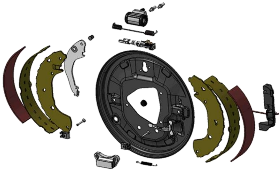
Figure 1.5. Exploded view diagram of the Simplex drum brake,
