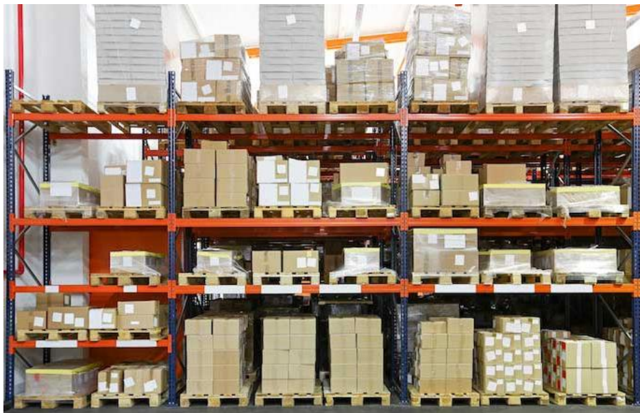
Figure 2.17. Conventional rack systems (source: Noega Systems)
