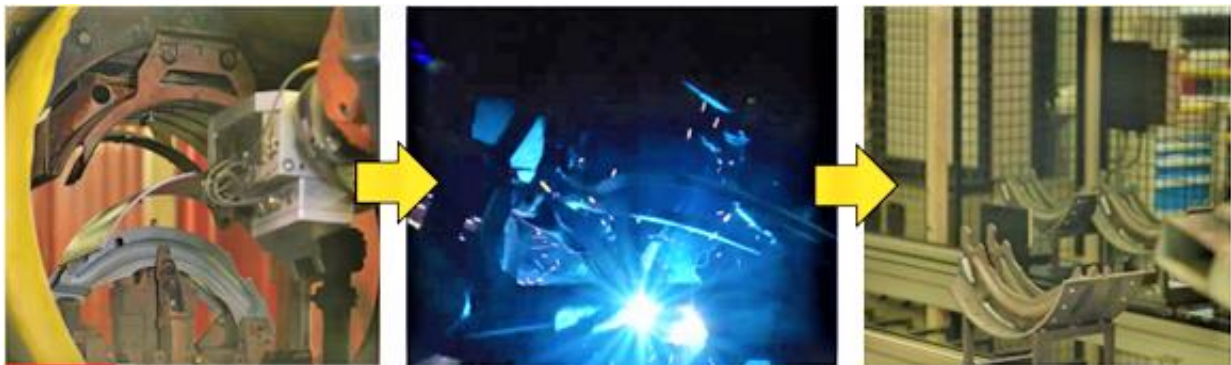
Figure 1.6. Shoe welding procedure: from the left to the right, web and table placement on the clamping jig, welding and finished product (source: BWP Bergische Achsen KG)
