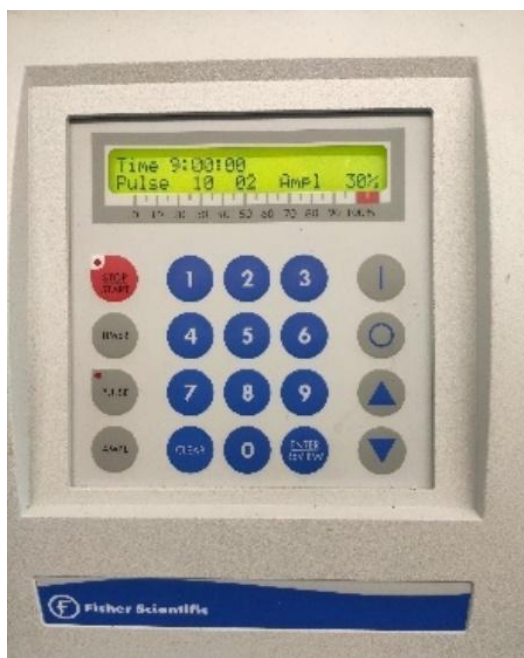
FIGURE 11. 500W FB505 SONIC DISMEMBRATOR FISHER SCIENTIFIC CONTROL SYSTEM
