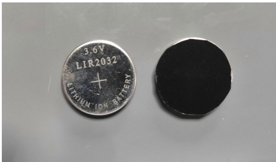
FIGURE 27. COIN CELL CARBON TAPE COATING
